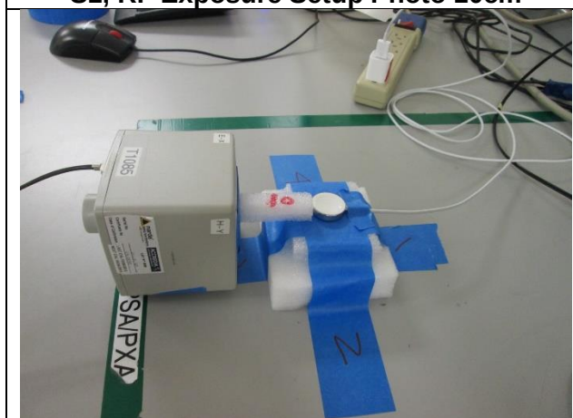
S3, RF Exposure Setup Photo 10cm
