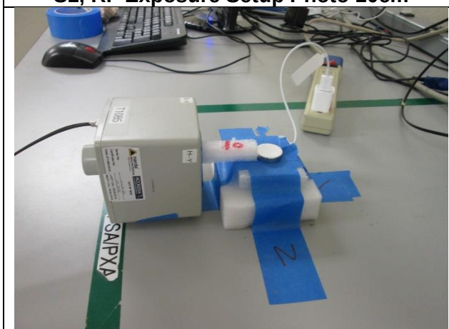
S3, RF Exposure Setup Photo 10cm
