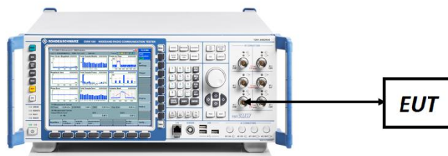
Figure 7-5. Conducted Power Measurement Setup
