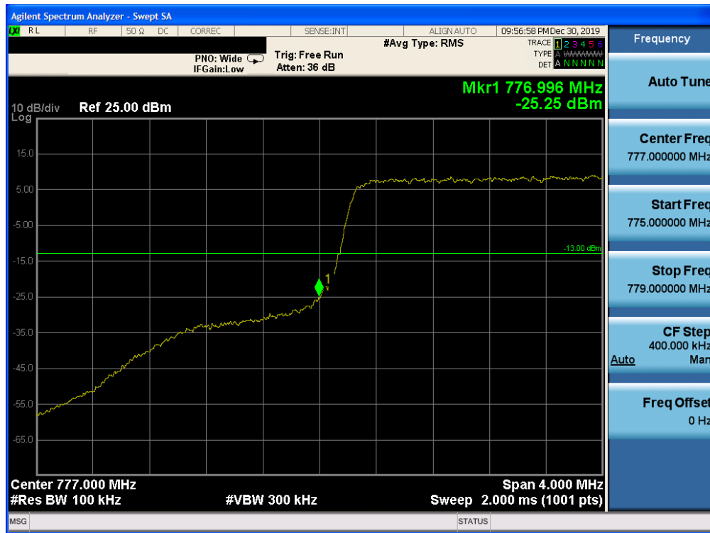
Plot 7-181. Lower Band Edge Plot (Band 13 – 5.0MHz QPSK – RB Size 25)
