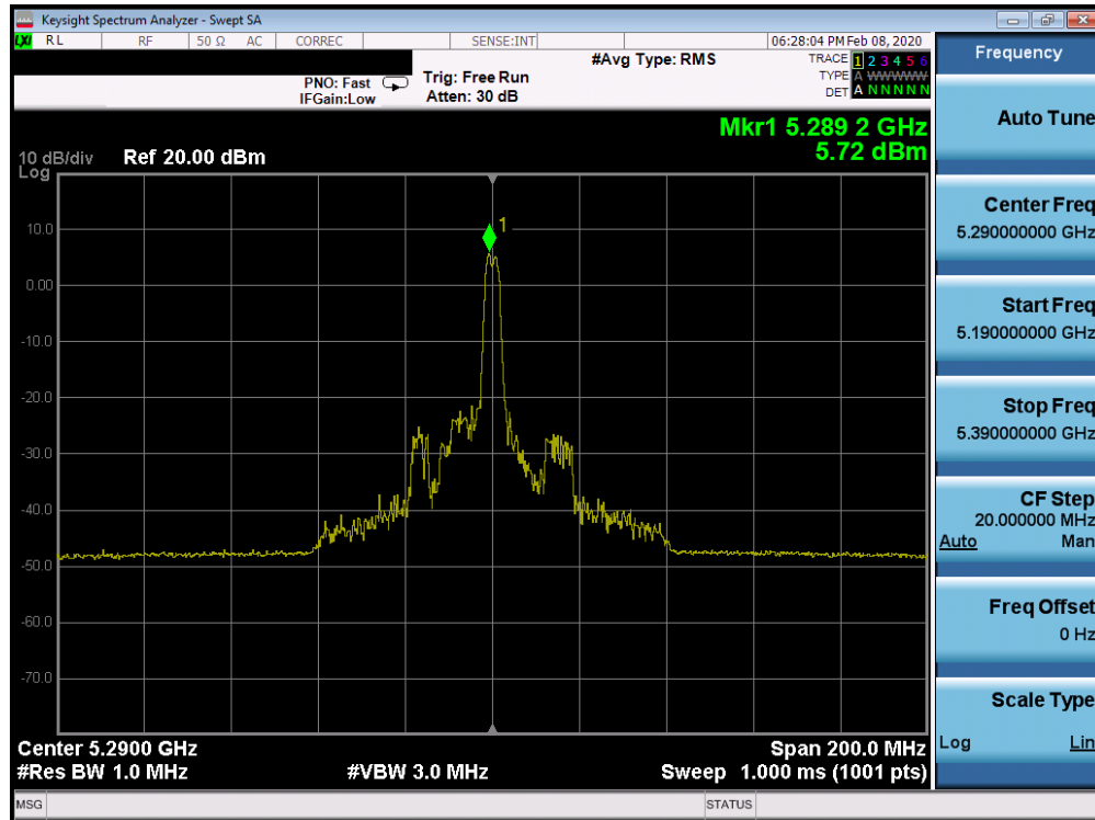
Plot 7-555. Power Spectral Density Plot CDD CORE 0 (80MHz BW 802.11ax Index 18 – RU26 (UNII Band 2A) – Ch. 58)
