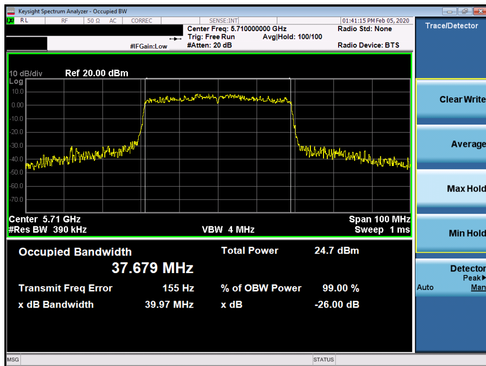
Plot 7-152. 26dB Bandwidth Plot SISO CORE 1 (40MHz BW 802.11ax – RU484 (UNII Band 2C) – Ch. 142)
