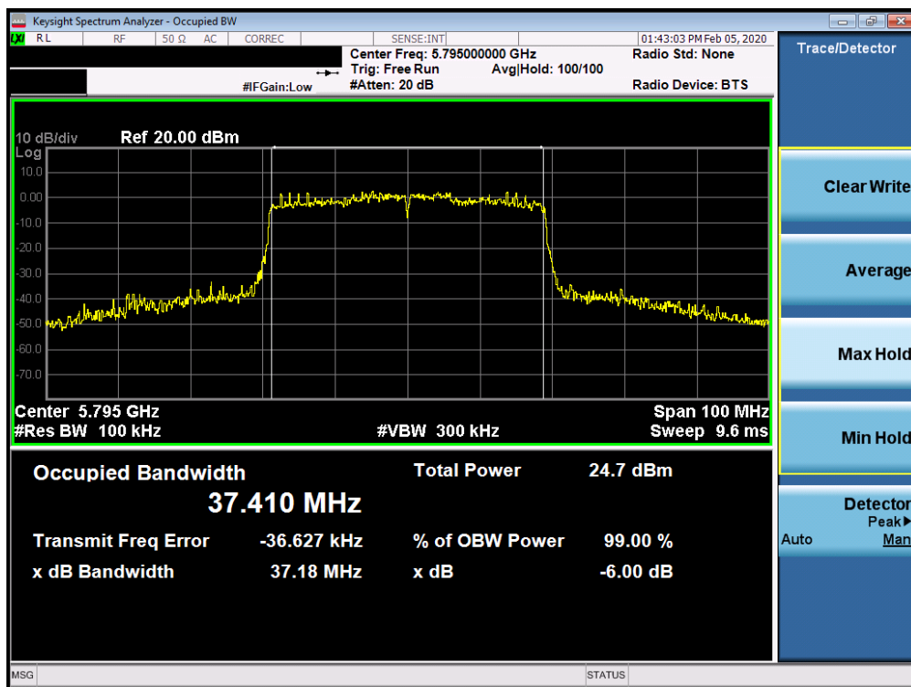
Plot 7-204. 6dB Bandwidth Plot SISO CORE 1 (40MHz BW 802.11ax – RU484 (UNII Band 3) – Ch. 159)
