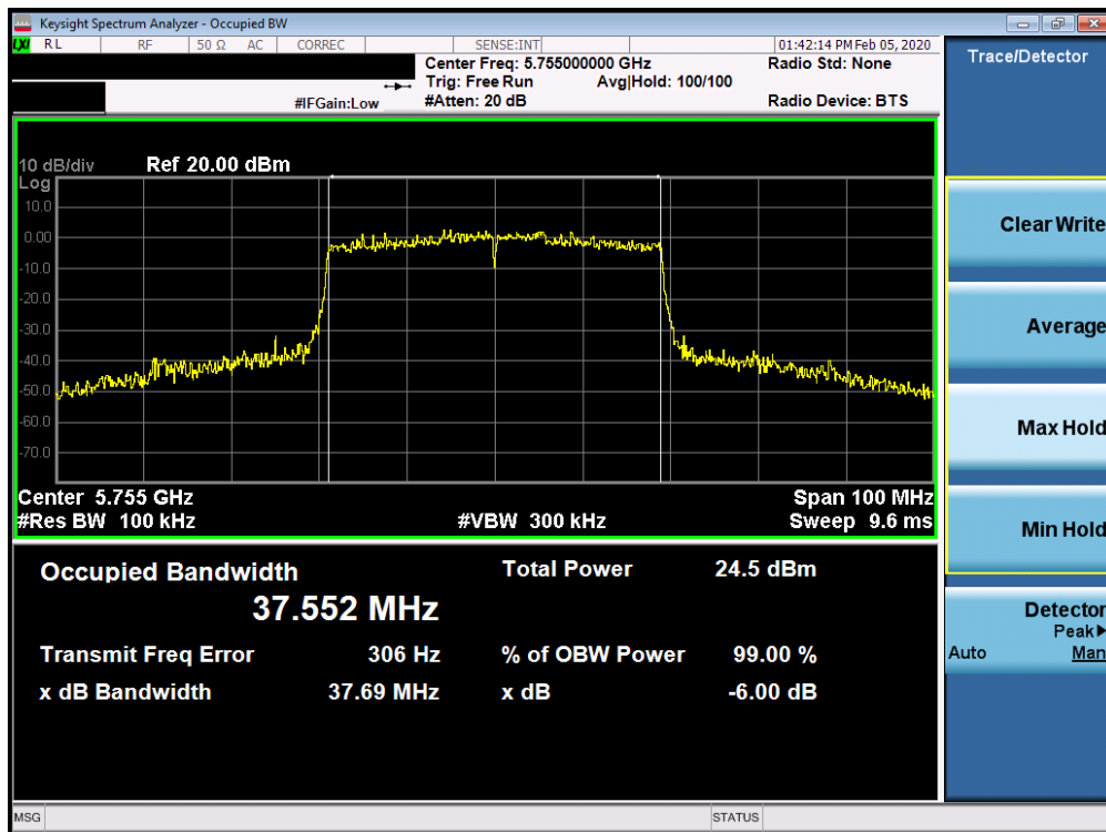
Plot 7-203. 6dB Bandwidth Plot SISO CORE 1 (40MHz BW 802.11ax – RU484 (UNII Band 3) – Ch. 151)
