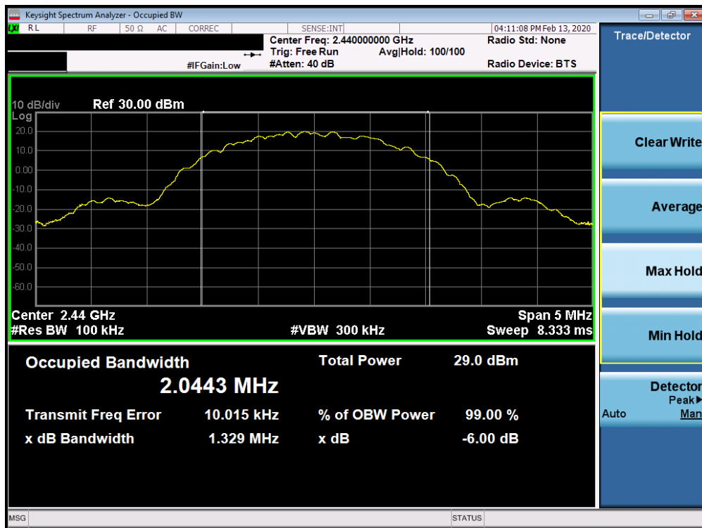
Plot 7-5. 6dB Bandwidth Plot Ant 4a (Bluetooth (LE), 2Mbps, ePA – Ch. 19)
