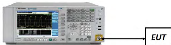
Figure 7-1. Test Instrument & Measurement Setup
