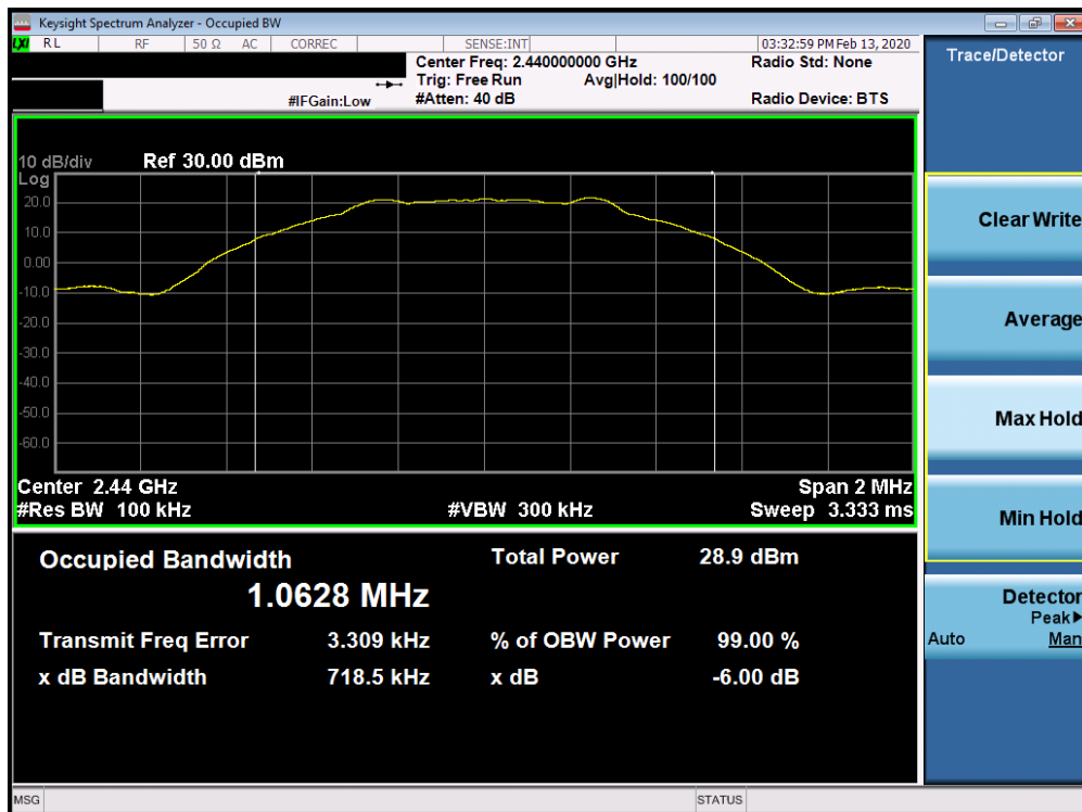
Plot 7-2. 6dB Bandwidth Plot Ant 4a (Bluetooth (LE), 1Mbps, ePA – Ch. 19)
