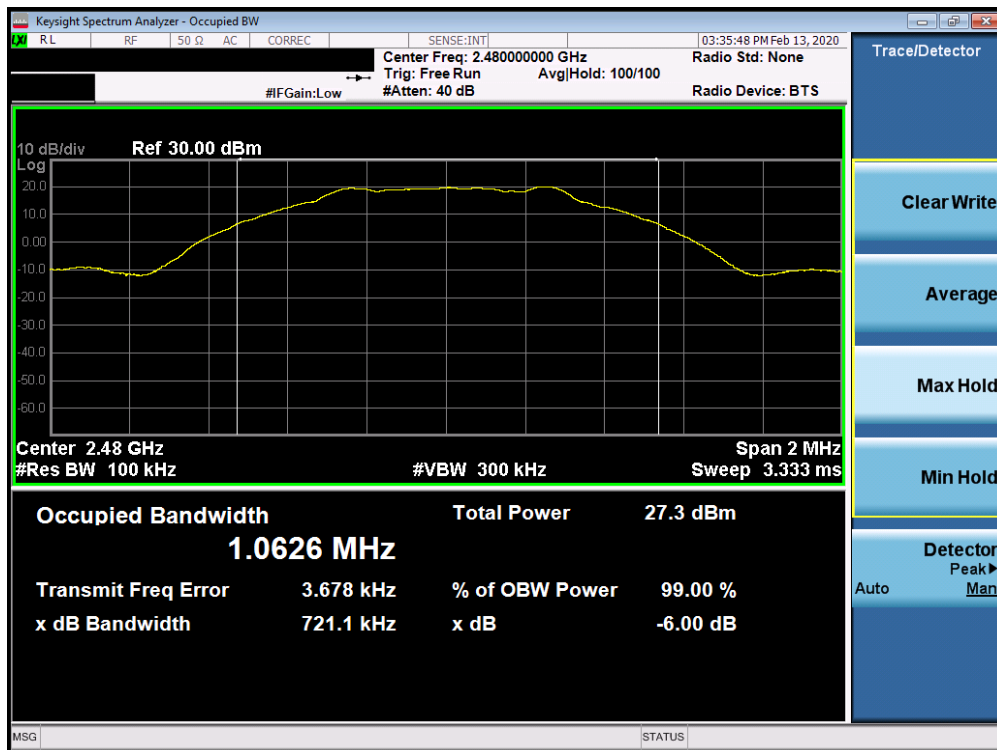
Plot 7-3. 6dB Bandwidth Plot Ant 4a (Bluetooth (LE), 1Mbps, ePA – Ch. 39)
