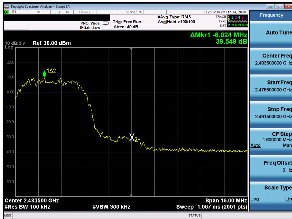
Plot 7-68. Band Edge Plot Ant 2a (Bluetooth (HDR8), ePA – Ch. 75)
