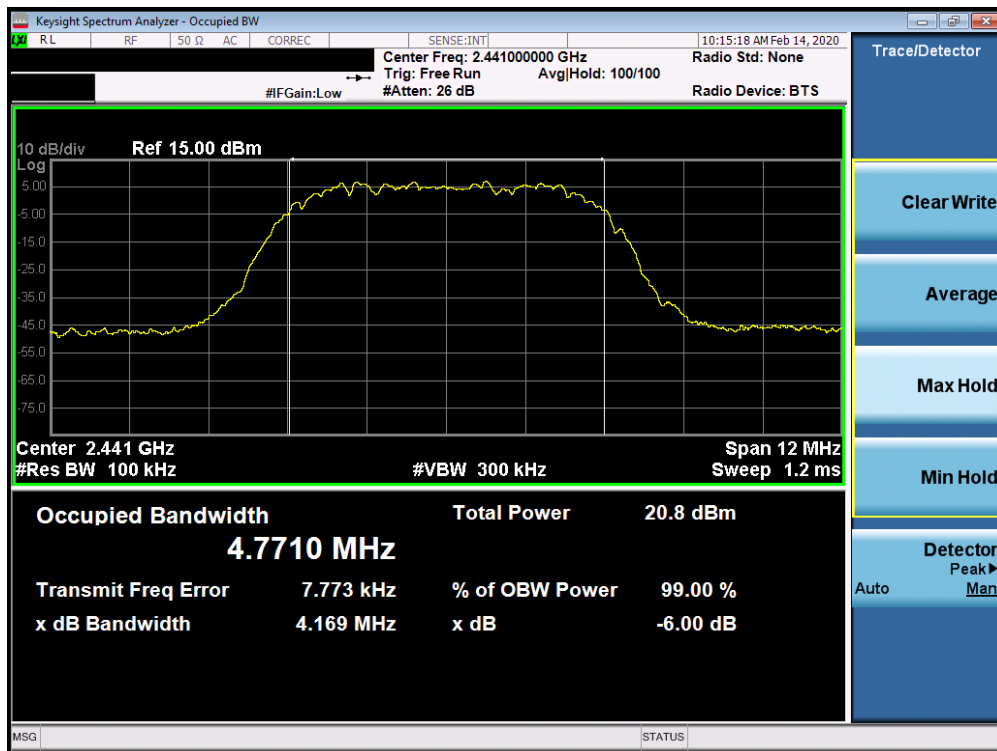
Plot 7-5. 6dB Bandwidth Plot Ant 4a (Bluetooth (HDR8), 8Mbps, ePA – Ch. 38)
