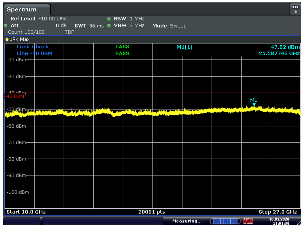
Plot 7-429. Radiated Spurious Plot 18GHz – 27GHz V (Band 30)
