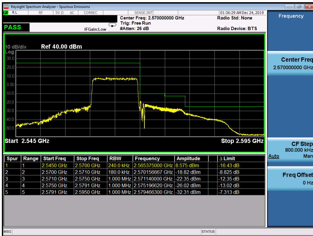
Plot 7-312. Upper ACP Plot (Band 7 – 10.0MHz QPSK – RB Size 50)
