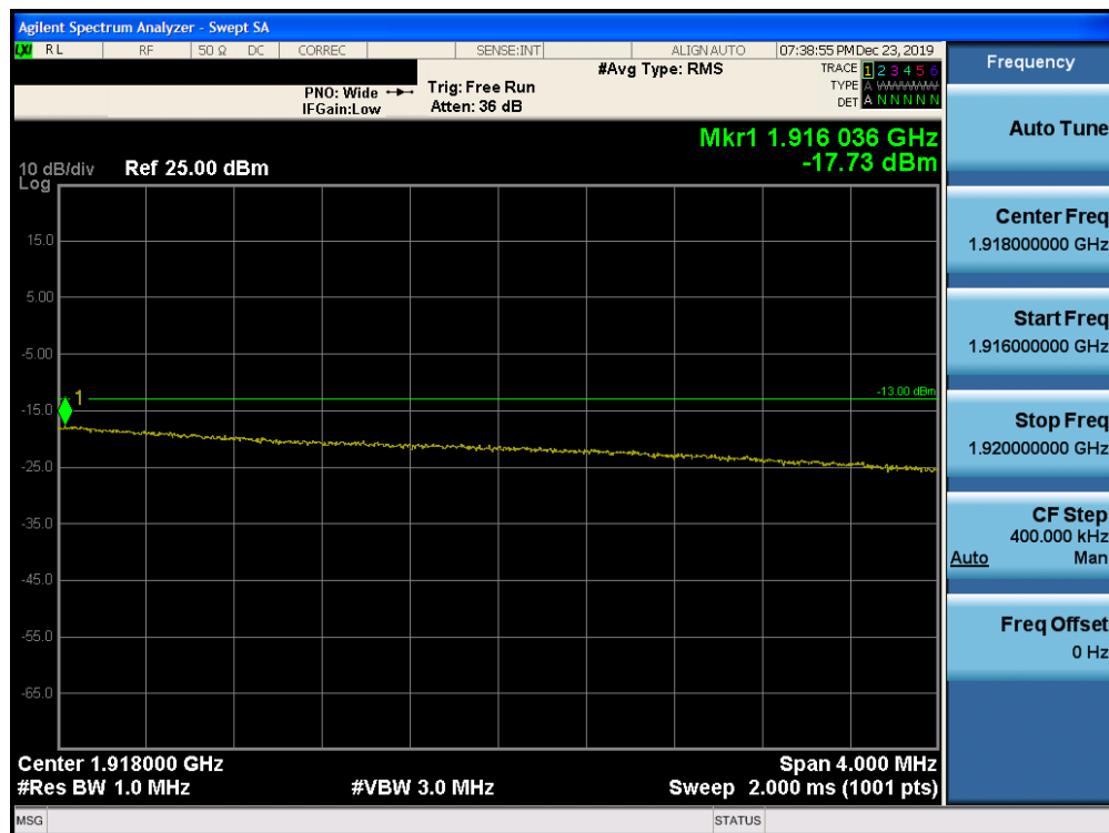
Plot 7-276. Upper Extended Band Edge Plot (Band 2 – 20.0MHz QPSK – RB Size 100)
