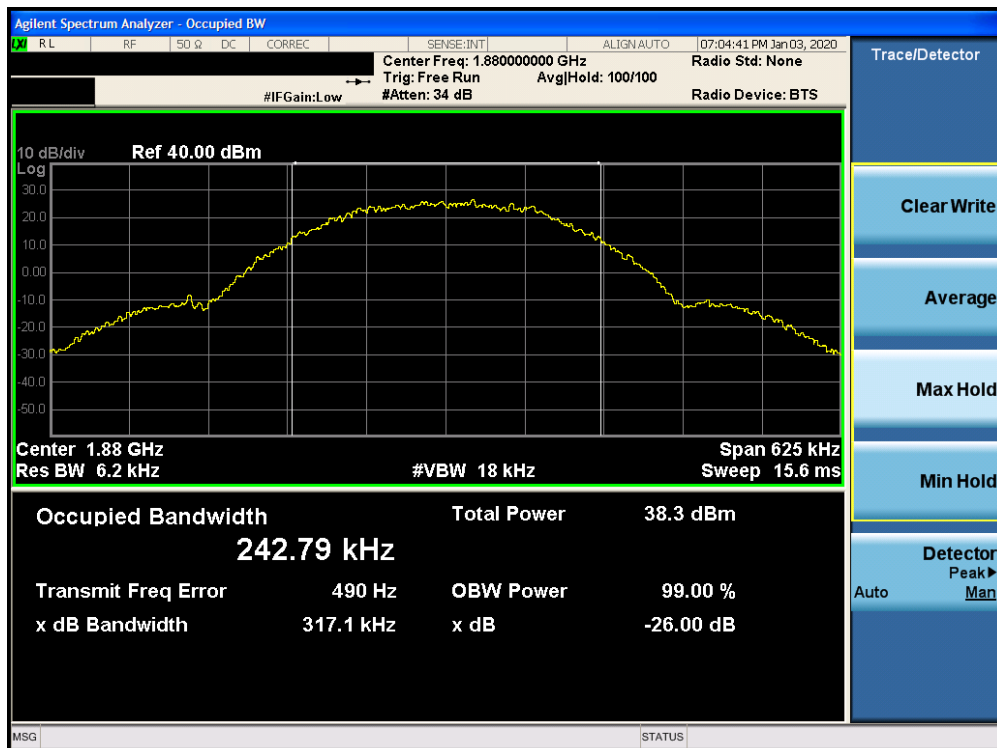
Plot 7-3. Occupied Bandwidth Plot (PCS GPRS Mode)
