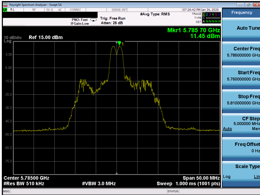
Plot 7-445. Power Spectral Density Plot SISO CORE 1 (20MHz BW 802.11ax Index 4 – RU26 (UNII Band 3) – Ch. 157)
