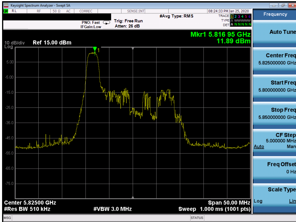
Plot 7-319. Power Spectral Density Plot SISO CORE 0 (20MHz BW 802.11ax Index 0 – RU26 (UNII Band 3) – Ch. 165)
