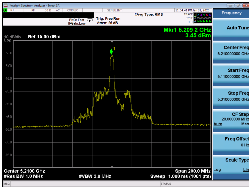
Plot 7-310. Power Spectral Density Plot ISSED SISO CORE 0 (80MHz BW 802.11ax Index 18 – RU26 (UNII Band 1) – Ch. 42)
