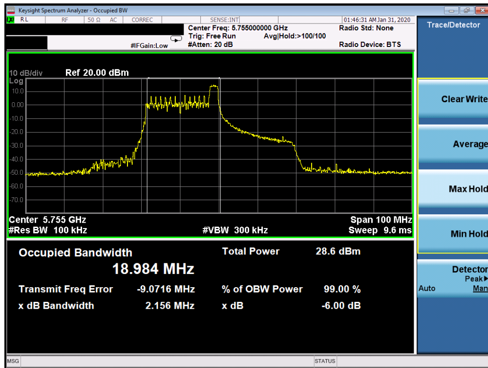
Plot 7-174. 6dB Bandwidth Plot SISO CORE 0 (40MHz BW 802.11ax Index 8 – RU26 (UNII Band 3) – Ch. 151)
