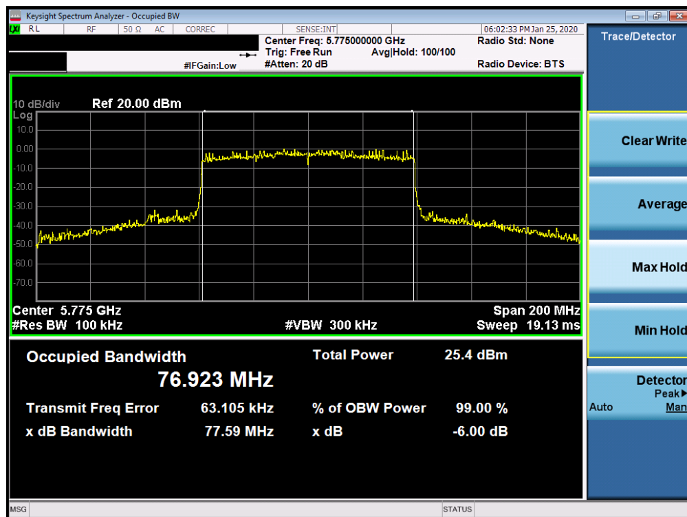
Plot 7-184. 6dB Bandwidth Plot SISO CORE 0 (80MHz BW 802.11ax – RU996 (UNII Band 3) – Ch. 155)
