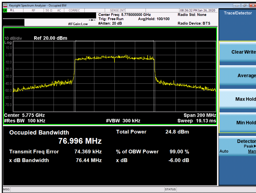
Plot 7-208. 6dB Bandwidth Plot SISO CORE 1 (80MHz BW 802.11ax - RU996 (UNII Band 3) – Ch. 155)
