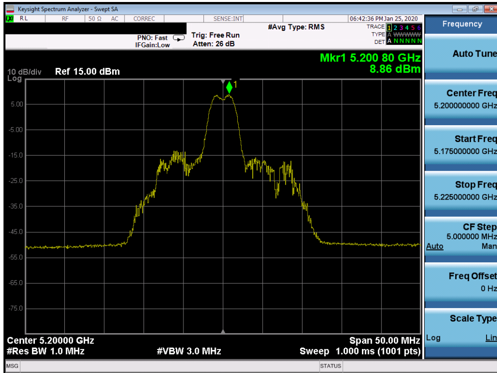
Plot 7-213. Power Spectral Density Plot SISO CORE 0 (20MHz BW 802.11ax Index 4 – RU26 (UNII Band 1) – Ch. 40)
