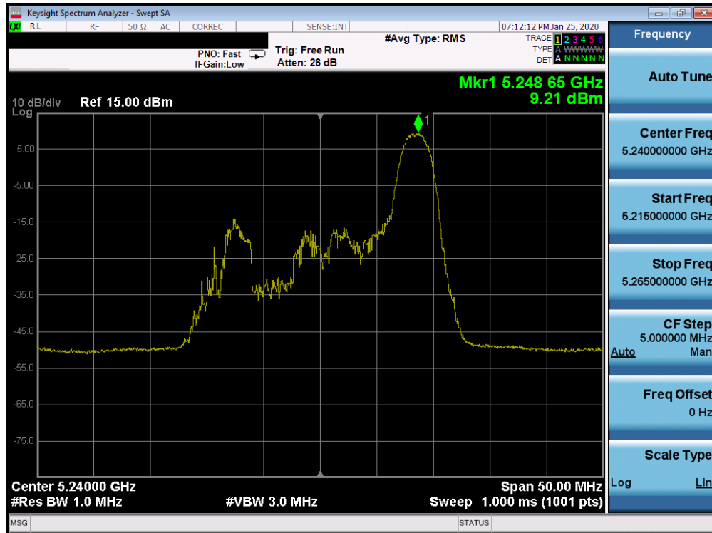
Plot 7-217. Power Spectral Density Plot SISO CORE 0 (20MHz BW 802.11ax Index 8 – RU26 (UNII Band 1) – Ch. 48)
