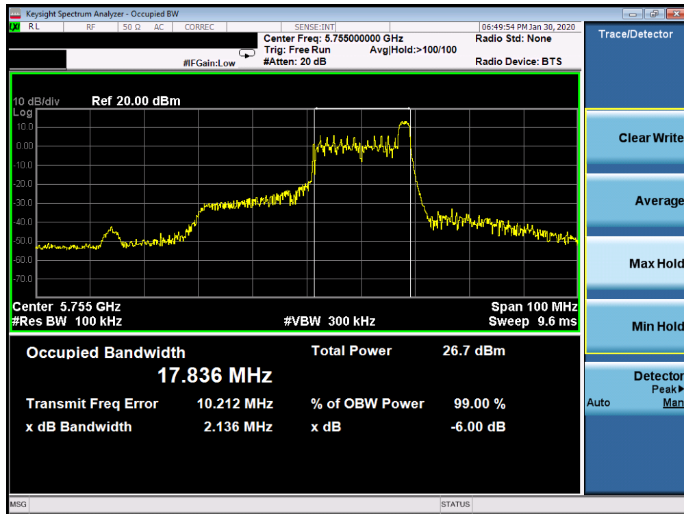
Plot 7-199. 6dB Bandwidth Plot SISO CORE 1 (40MHz BW 802.11ax Index 17 – RU26 (UNII Band 3) – Ch. 151)
