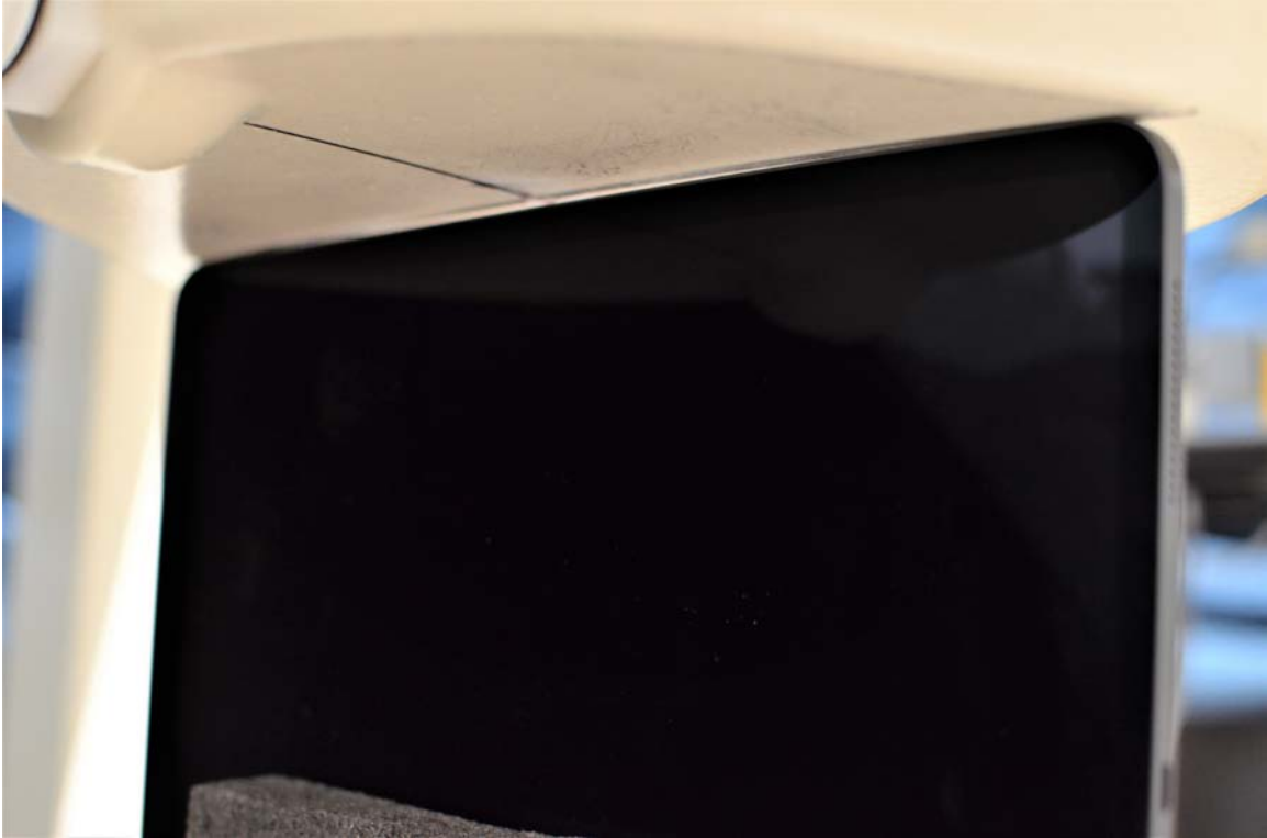
SAR Test Setup Photo 5: Right Edge at 0.0 cm
