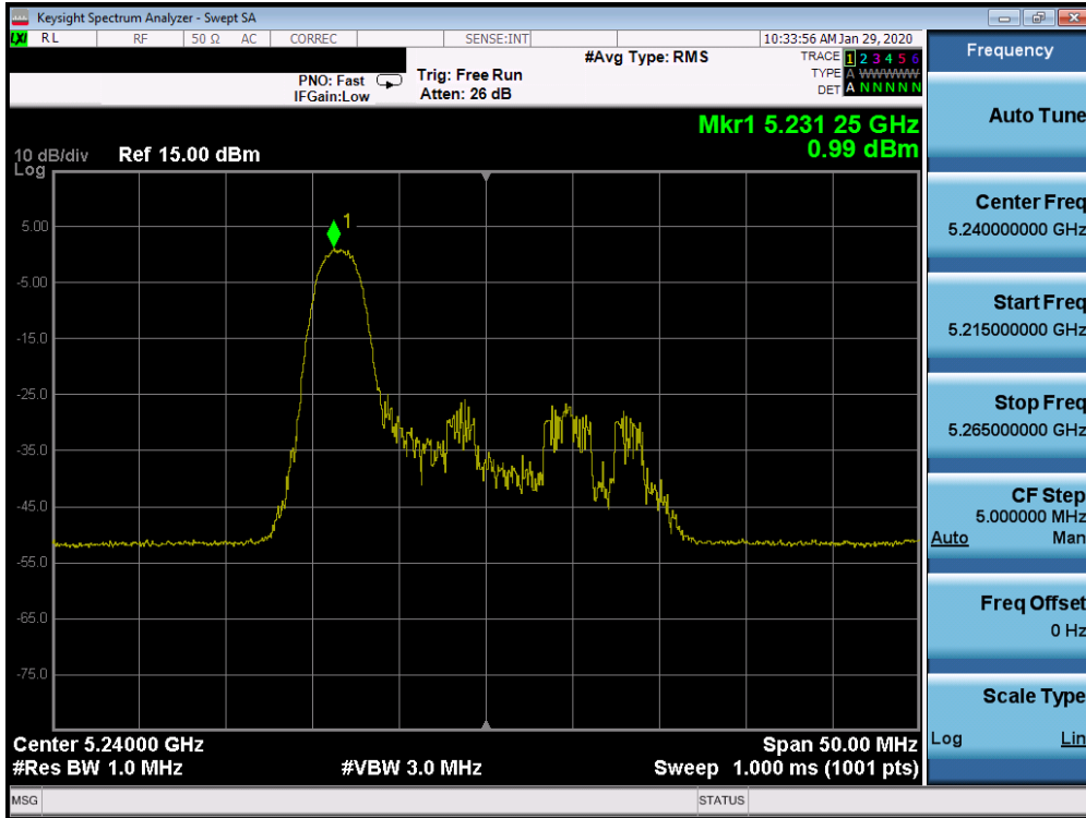
Plot 7-637. Power Spectral Density Plot ISED CDD CORE 0 (20MHz BW 802.11ax Index 0 – RU26 (UNII Band 1) – Ch. 48)
