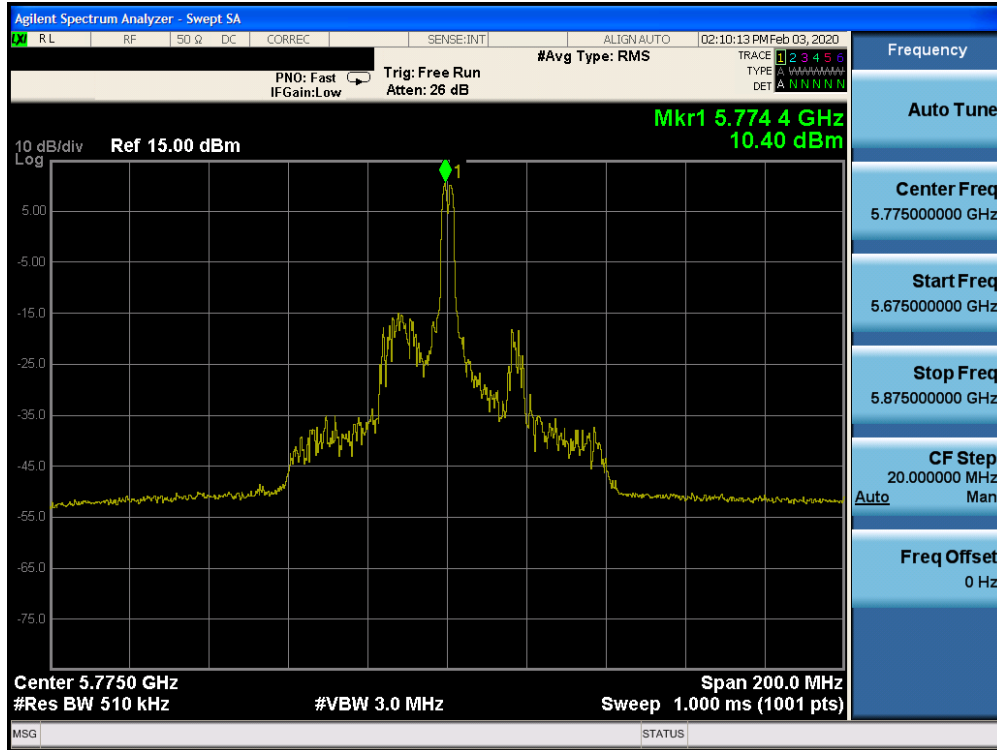
Plot 7-715. Power Spectral Density Plot CDD CORE 0 (80MHz BW 802.11ax Index 18 – RU26 (UNII Band 3) – Ch. 155)
