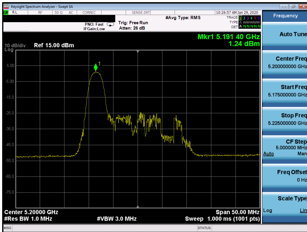
Plot 7-632. Power Spectral Density Plot ISED CDD CORE 1 (20MHz BW 802.11ax Index 0 – RU26 (UNII Band 1) – Ch. 40)
