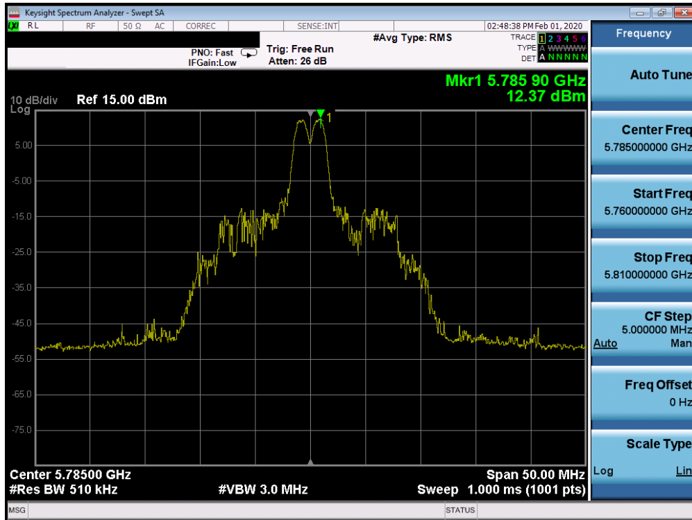
Plot 7-681. Power Spectral Density Plot CDD CORE 0 (20MHz BW 802.11ax Index 4 – RU26 (UNII Band 3) – Ch. 157)
