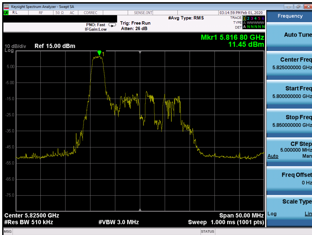
Plot 7-686. Power Spectral Density Plot CDD CORE 1 (20MHz BW 802.11ax Index 0 – RU26 (UNII Band 3) – Ch. 165)
