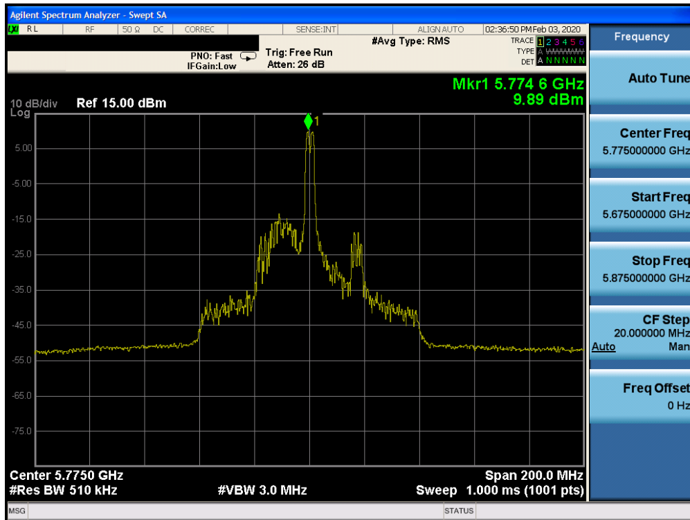
Plot 7-716. Power Spectral Density Plot CDD CORE 1 (80MHz BW 802.11ax Index 18 – RU26 (UNII Band 3) – Ch. 155)
