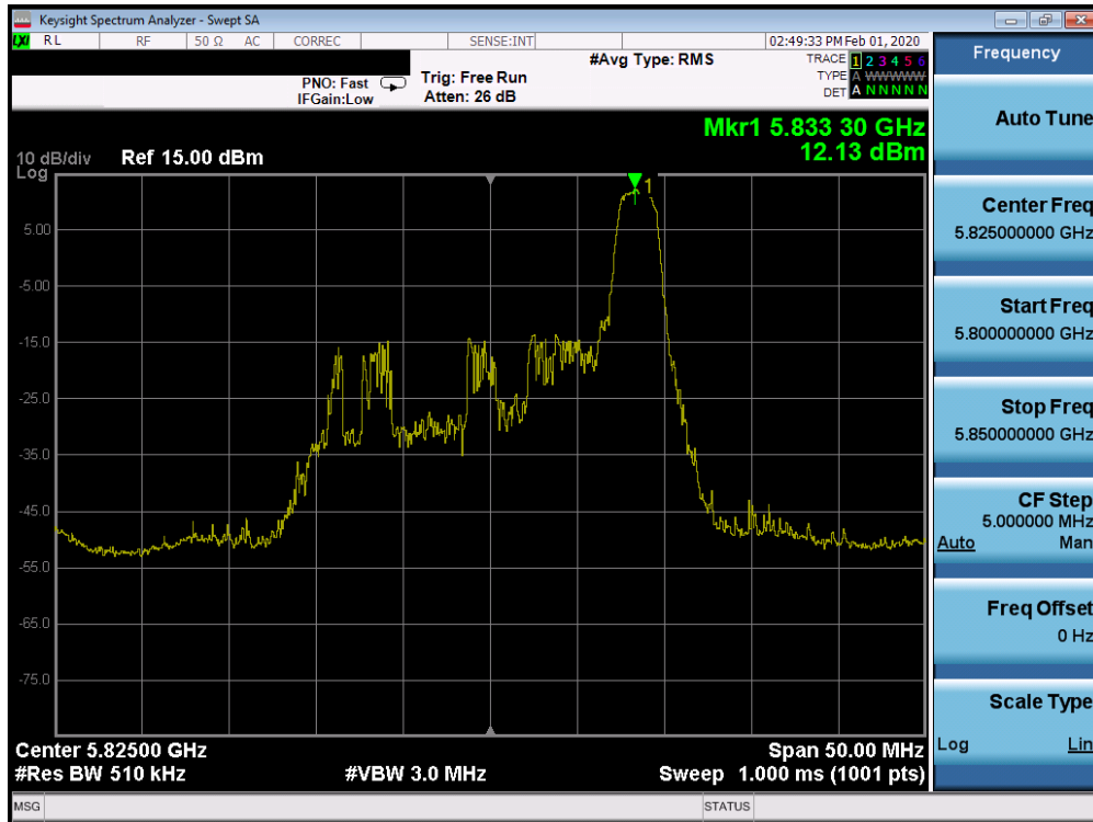
Plot 7-689. Power Spectral Density Plot CDD CORE 0 (20MHz BW 802.11ax Index 8 – RU26 (UNII Band 3) – Ch. 165)
