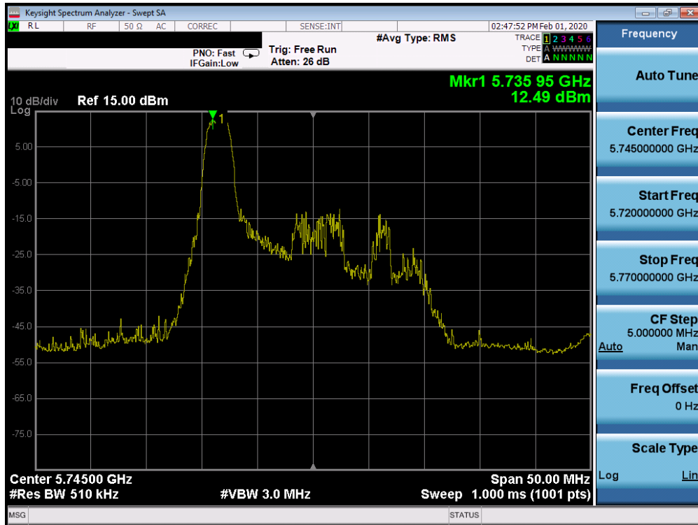
Plot 7-673. Power Spectral Density Plot CDD CORE 0 (20MHz BW 802.11ax Index 0 – RU26 (UNII Band 3) – Ch. 149)
