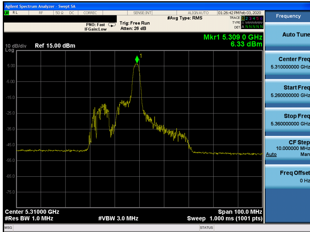
Plot 7-545. Power Spectral Density Plot CDD CORE 0 (40MHz BW 802.11ax Index 8 – RU26 (UNII Band 2A) – Ch. 62)
