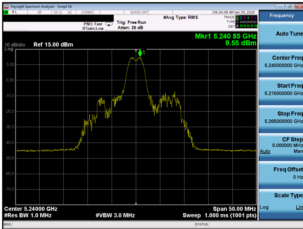
Plot 7-344. Power Spectral Density Plot SISO CORE 1 (20MHz BW 802.11ax Index 4 – RU26 (UNII Band 1) – Ch. 48)
