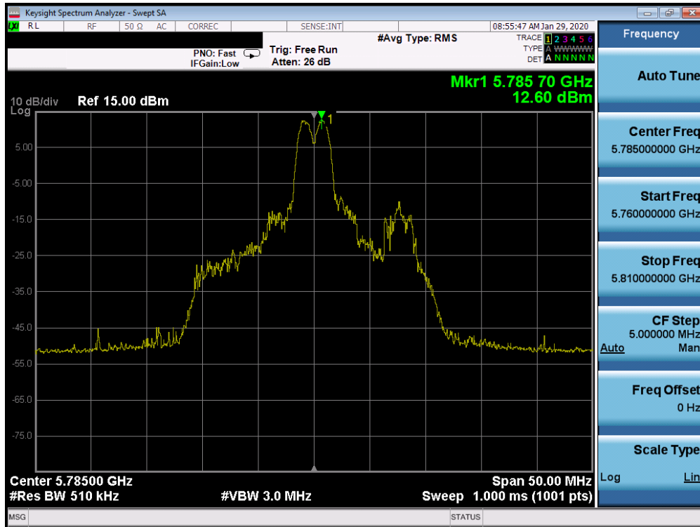
Plot 7-293. Power Spectral Density Plot SISO CORE 0 (20MHz BW 802.11ax Index 4 – RU26 (UNII Band 3) – Ch. 157)
