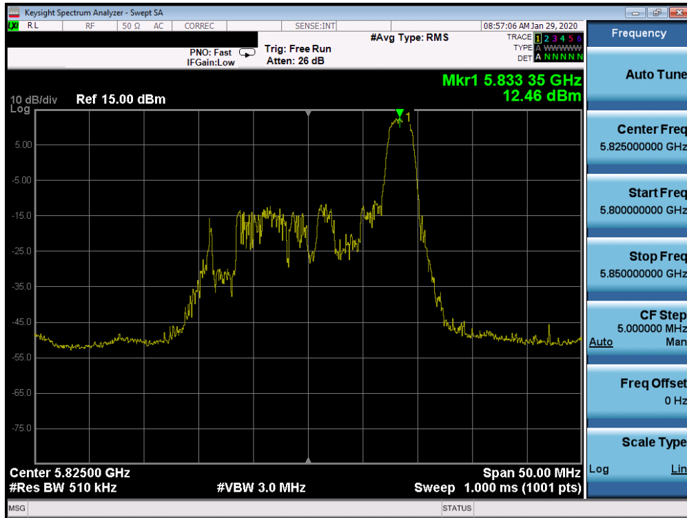
Plot 7-297. Power Spectral Density Plot SISO CORE 0 (20MHz BW 802.11ax Index 8 – RU26 (UNII Band 3) – Ch. 165)
