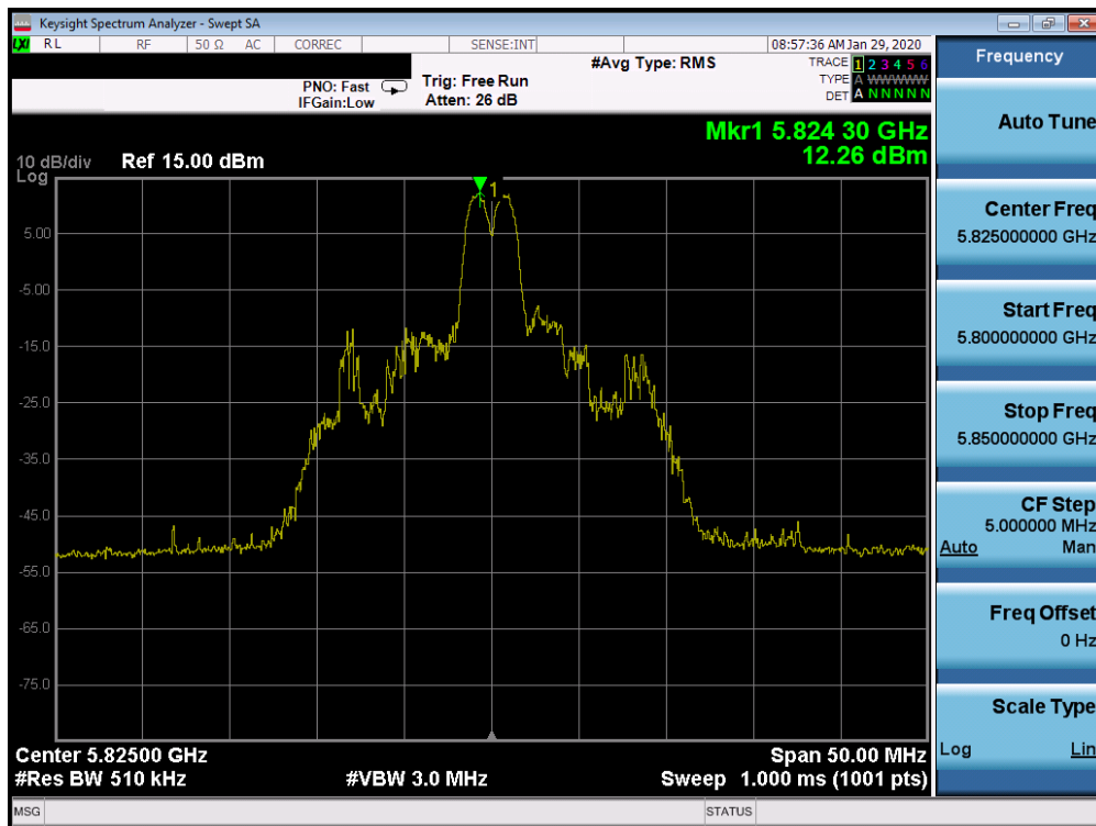
Plot 7-296. Power Spectral Density Plot SISO CORE 0 (20MHz BW 802.11ax Index 4 – RU26 (UNII Band 3) – Ch. 165)
