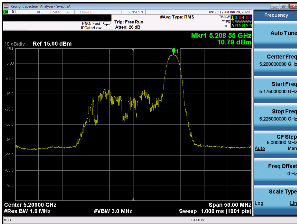
Plot 7-342. Power Spectral Density Plot SISO CORE 1 (20MHz BW 802.11ax Index 8– RU26 (UNII Band 1) – Ch. 40)
