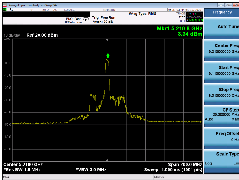
Plot 7-334. Power Spectral Density ISED Plot SISO CORE 0 (80MHz BW 802.11ax Index 18 – RU26 (UNII Band 1) – Ch. 42)
