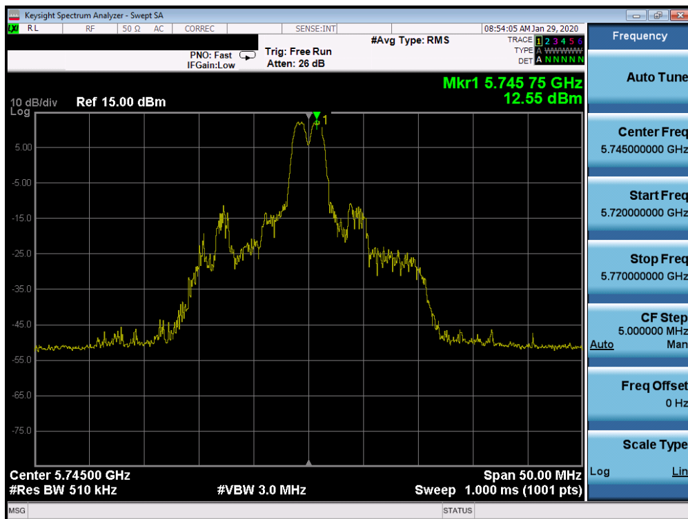
Plot 7-290. Power Spectral Density Plot SISO CORE 0 (20MHz BW 802.11ax Index 4 – RU26 (UNII Band 3) – Ch. 149)
