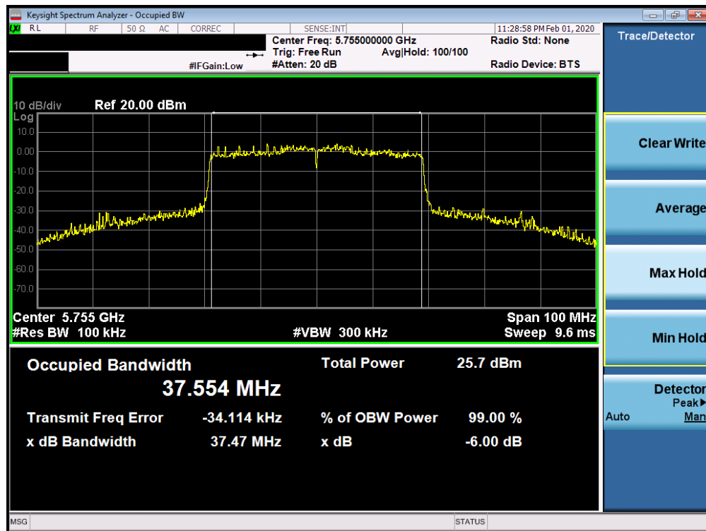
Plot 7-179. 6dB Bandwidth Plot SISO CORE 0 (40MHz BW 802.11ax – RU484 (UNII Band 3) – Ch. 151)
