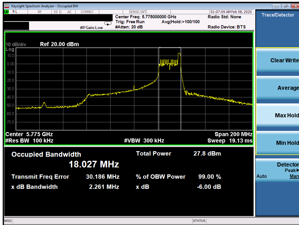
Plot 7-207. 6dB Bandwidth Plot SISO CORE 1 (80MHz BW 802.11ax Index 36 – RU26 (UNII Band 3) – Ch. 155)
