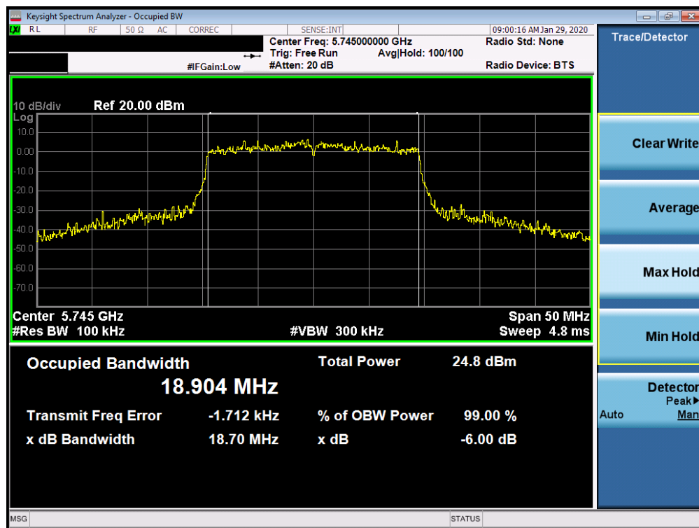
Plot 7-170. 6dB Bandwidth Plot SISO CORE 0 (20MHz BW 802.11ax– RU242 (UNII Band 3) – Ch. 149)
