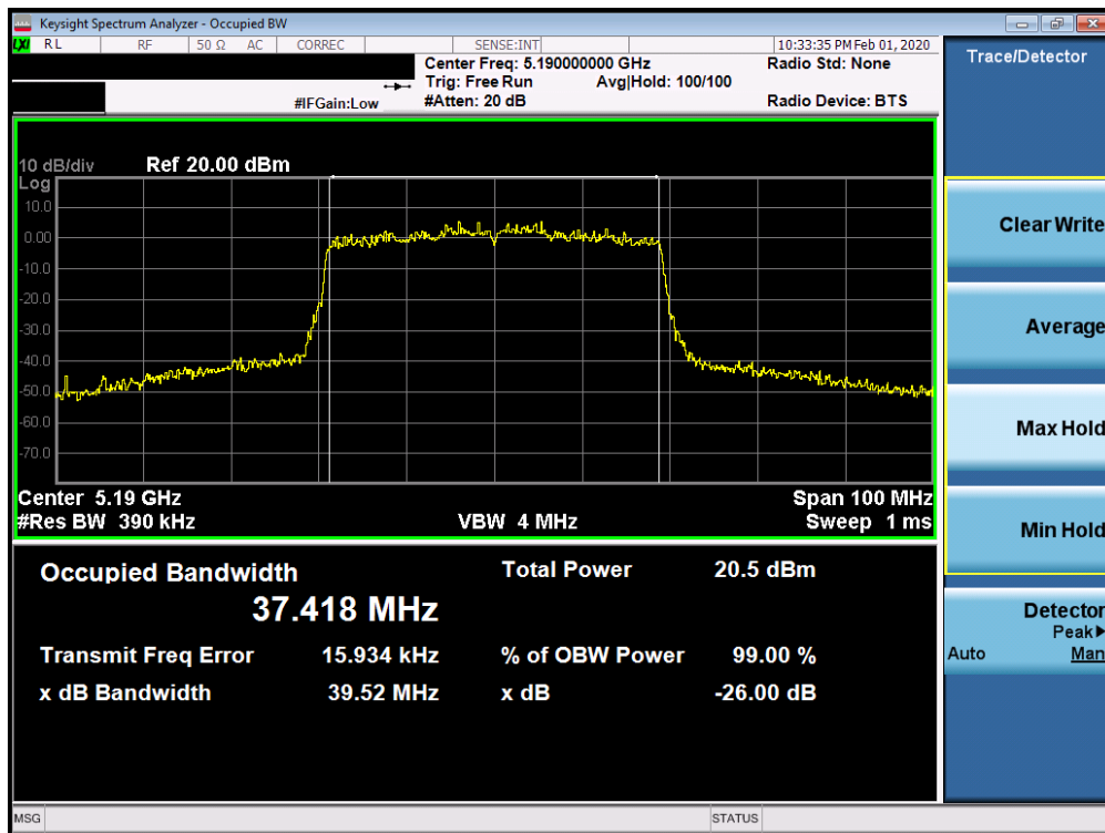
Plot 7-19. 26dB Bandwidth Plot SISO CORE 0 (40MHz BW 802.11ax – RU484 (UNII Band 1) – Ch. 38)
