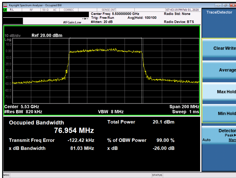
Plot 7-79. 26dB Bandwidth Plot SISO CORE 0 (80MHz BW 802.11ax – RU996 (UNII Band 2C) – Ch. 106)
