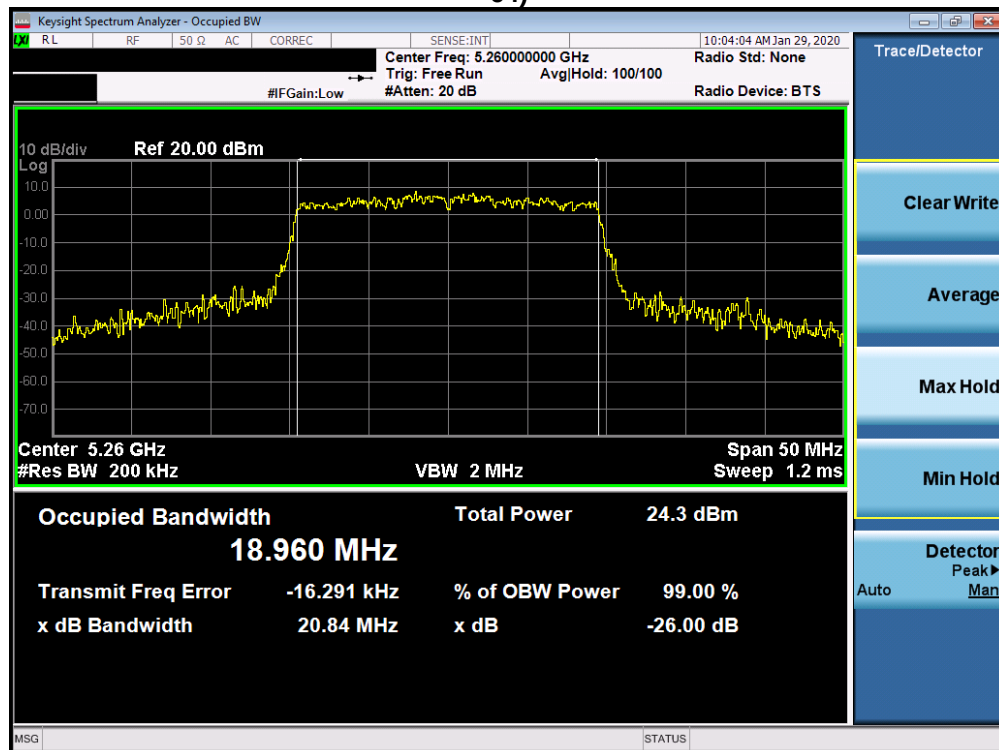
Plot 7-114. 26dB Bandwidth Plot SISO CORE 1 (20MHz BW 802.11ax– RU242 (UNII Band 2A) – Ch. 52)
