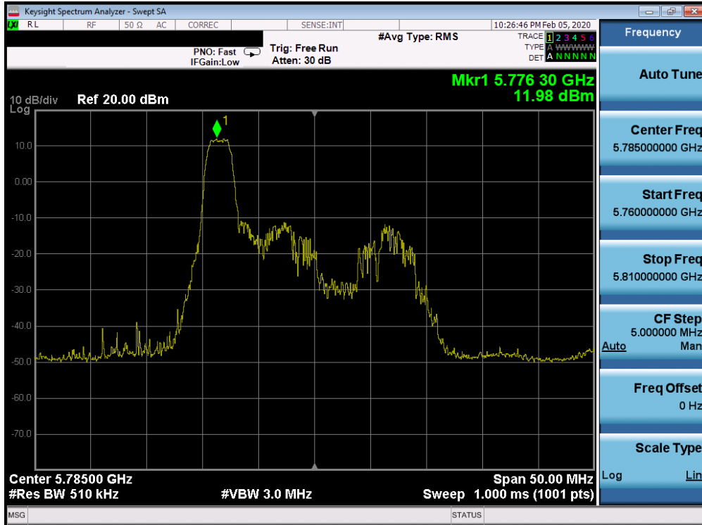
Plot 7-652. Power Spectral Density Plot CDD CORE 0 (20MHz BW 802.11ax Index 0 – RU26 (UNII Band 3) – Ch. 157)
