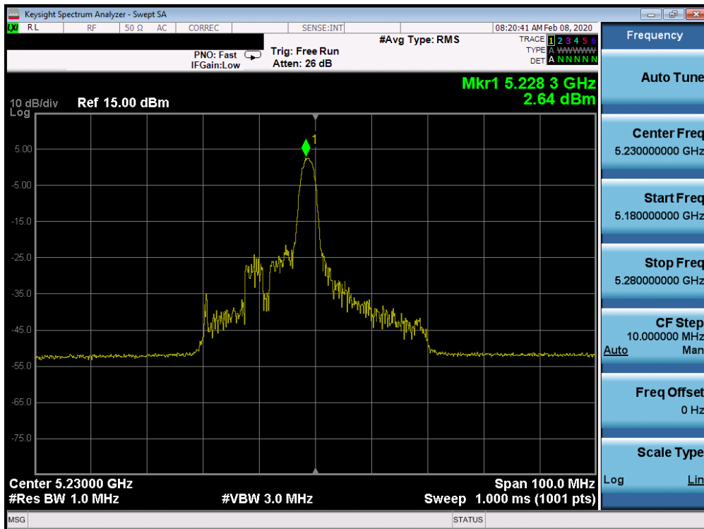
Plot 7-631. Power Spectral Density Plot ISED CDD CORE 1 (40MHz BW 802.11ax Index 8 – RU26 (UNII Band 1) – Ch. 46)
