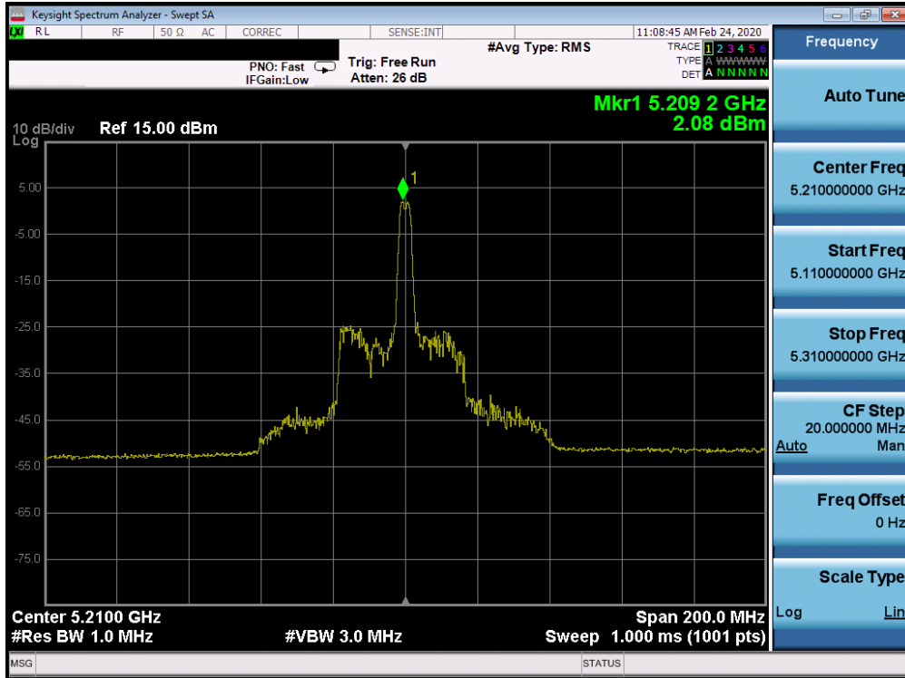
Plot 7-640. Power Spectral Density Plot ISED CDD CORE 0 (80MHz BW 802.11ax Index 18 – RU26 (UNII Band 1) – Ch. 42)
