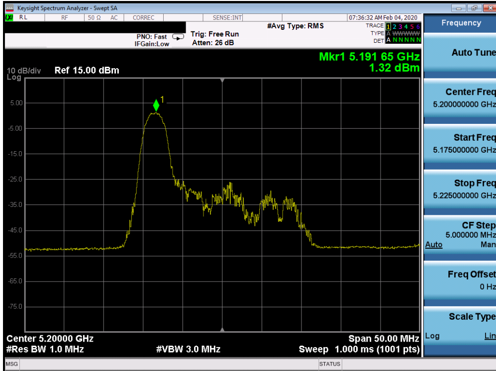
Plot 7-604. Power Spectral Density Plot ISED CDD CORE 0 (20MHz BW 802.11ax Index 0 – RU26 (UNII Band 1) – Ch. 40)
