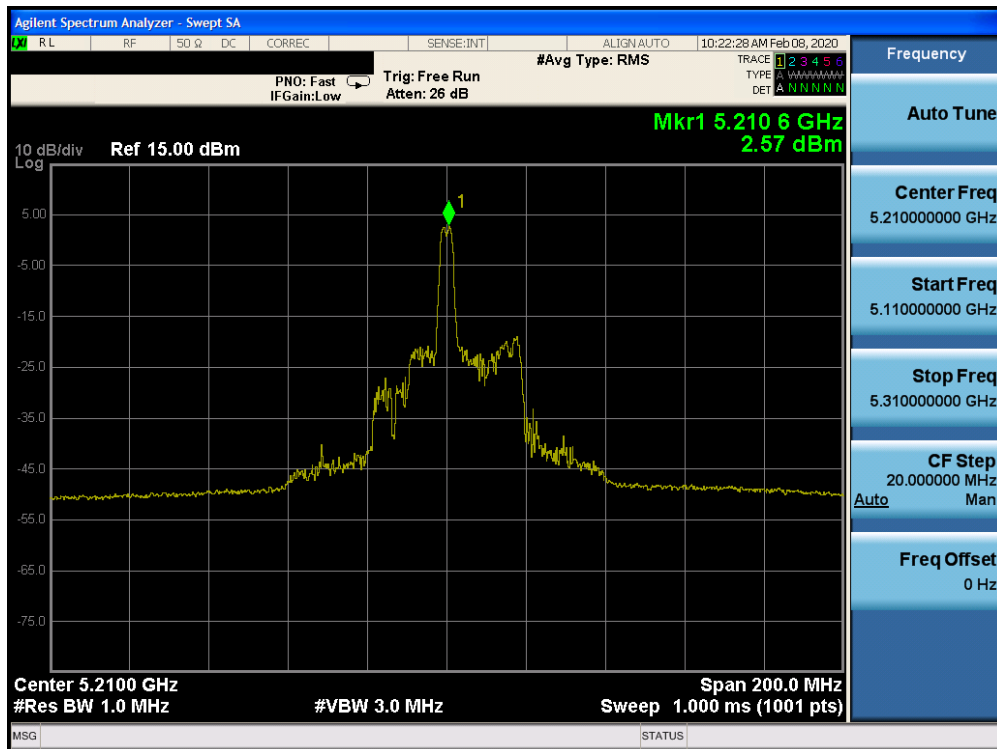
Plot 7-641. Power Spectral Density Plot ISED CDD CORE 1 (80MHz BW 802.11ax Index 18 – RU26 (UNII Band 1) – Ch. 42)
