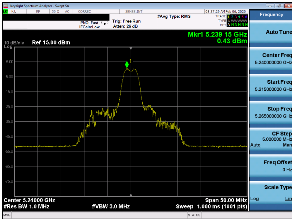
Plot 7-613. Power Spectral Density Plot ISED CDD CORE 1 (20MHz BW 802.11ax Index 4 – RU26 (UNII Band 1) – Ch. 48)
