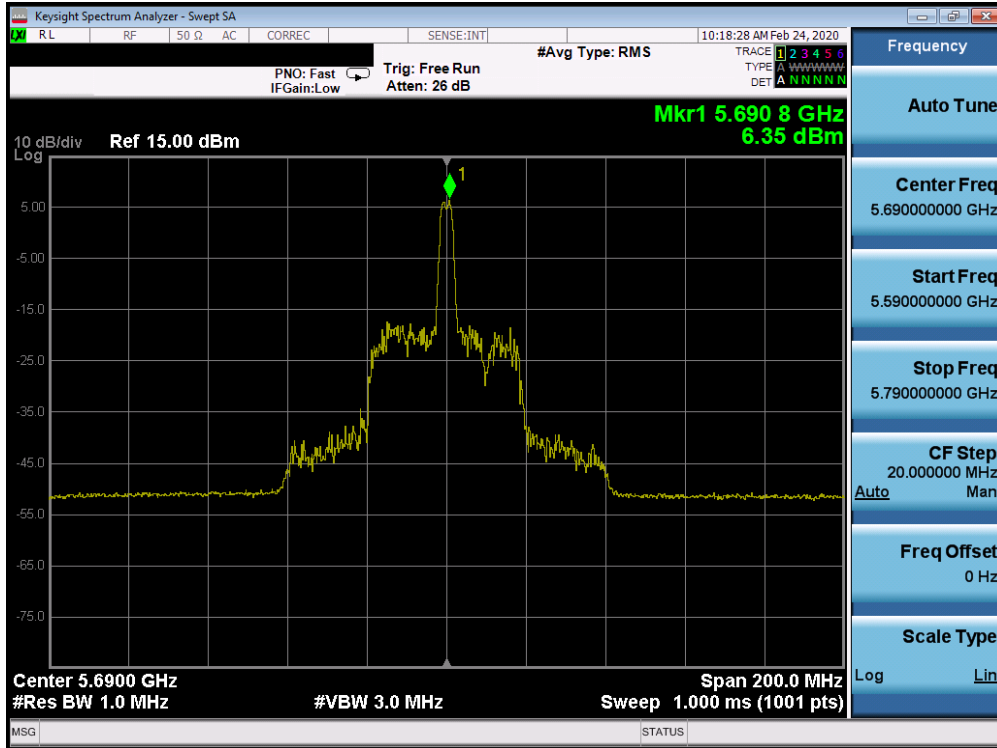
Plot 7-590. Power Spectral Density Plot SDM CORE 0 (80MHz BW 802.11ax Index 18 – RU26 (UNII Band 2C) – Ch. 138)
