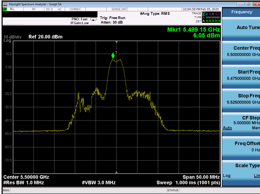
Plot 7-536. Power Spectral Density Plot SDM CORE 0 (20MHz BW 802.11ax Index 4 – RU26 (UNII Band 2C) – Ch. 100)
