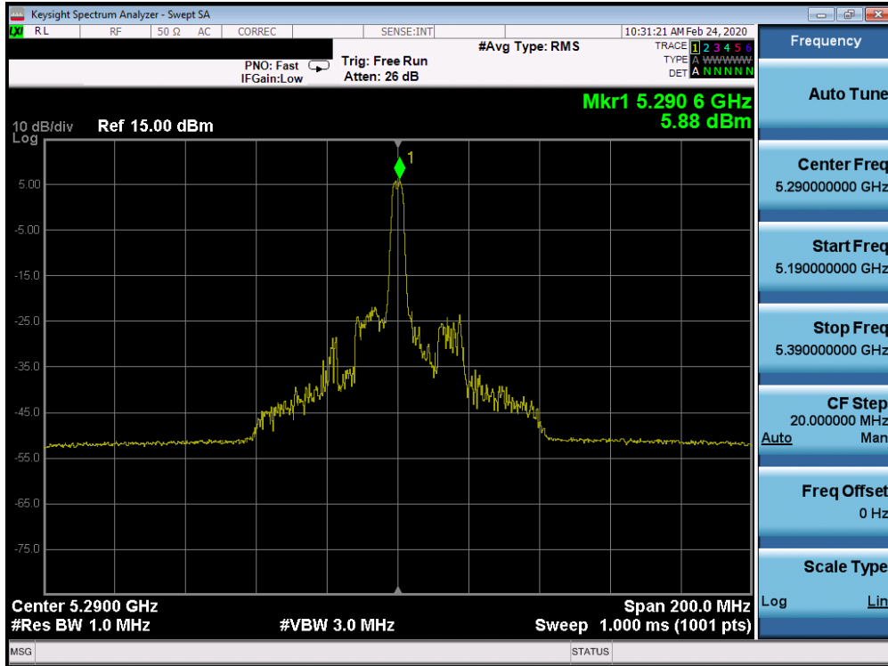
Plot 7-528. Power Spectral Density Plot SDM CORE 0 (80MHz BW 802.11ax Index 18 – RU26 (UNII Band 2A) – Ch. 58)
