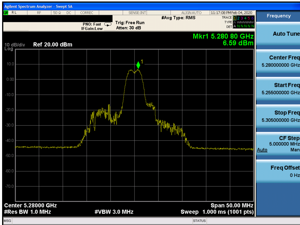
Plot 7-495. Power Spectral Density Plot SDM CORE 1 (20MHz BW 802.11ax Index 4 – RU26 (UNII Band 2A) – Ch. 56)
