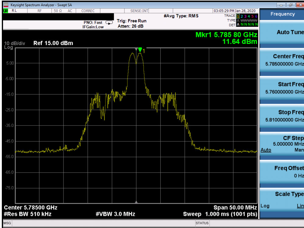
Plot 7-418. Power Spectral Density Plot SISO CORE 1 (20MHz BW 802.11ax Index 4 – RU26 (UNII Band 3) – Ch. 157)
