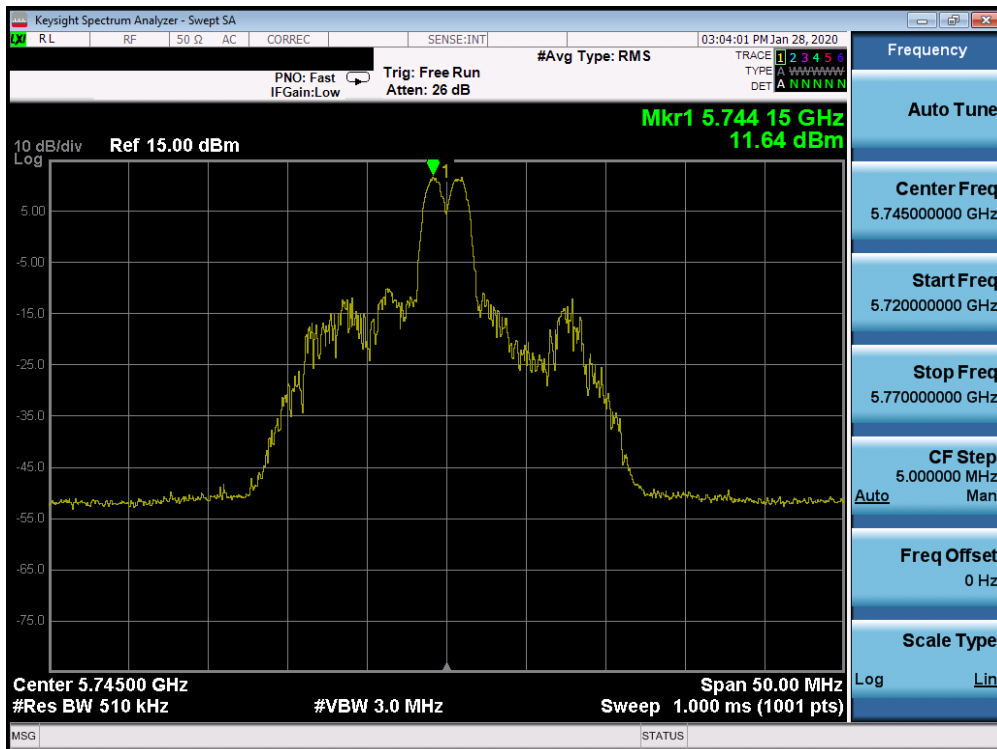
Plot 7-415. Power Spectral Density Plot SISO CORE 1 (20MHz BW 802.11ax Index 4 – RU26 (UNII Band 3) – Ch. 149)
