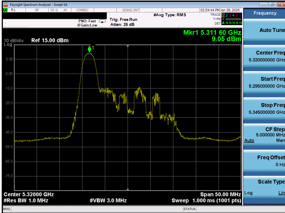
Plot 7-364. Power Spectral Density Plot SISO CORE 1 (20MHz BW 802.11ax Index 0 – RU26 (UNII Band 2A) – Ch. 64)
