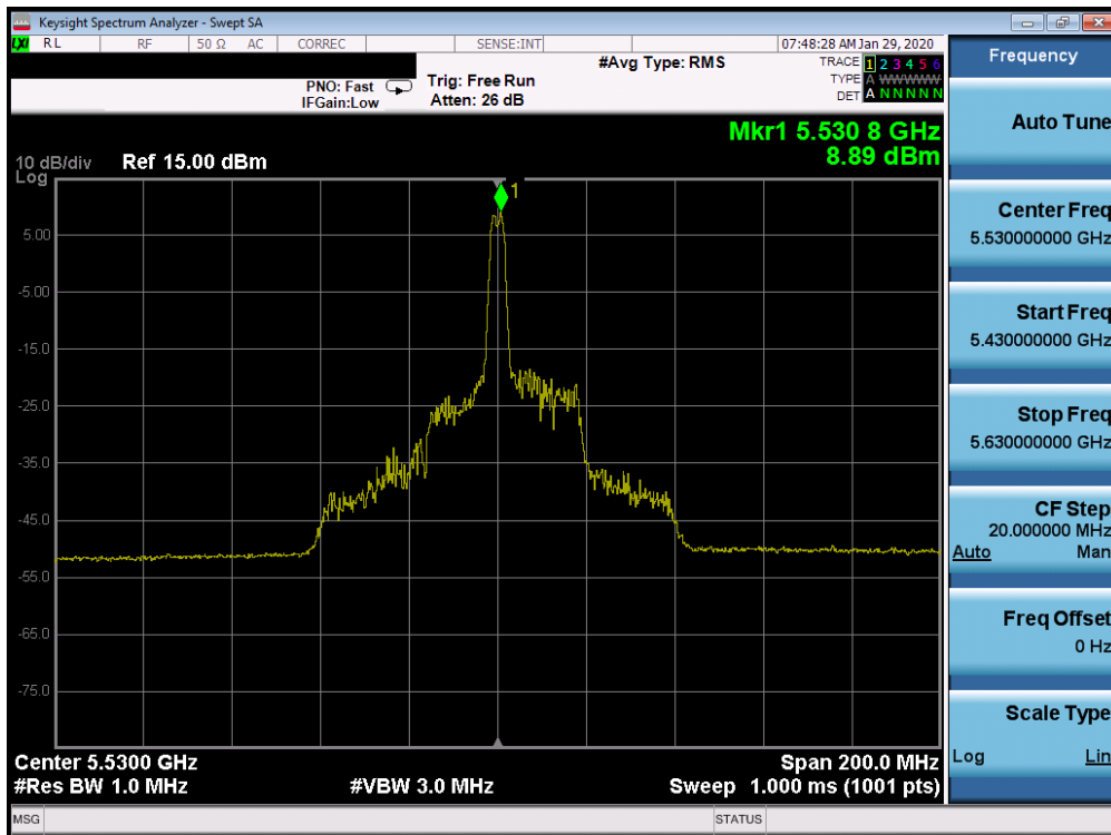
Plot 7-407. Power Spectral Density Plot SISO CORE 1 (80MHz BW 802.11ax Index 18 – RU26 (UNII Band 2C) – Ch. 106)
