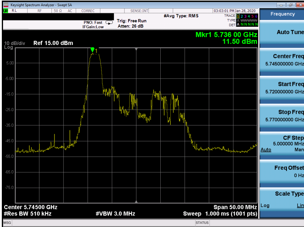
Plot 7-414. Power Spectral Density Plot SISO CORE 1 (20MHz BW 802.11ax Index 0 – RU26 (UNII Band 3) – Ch. 149)
