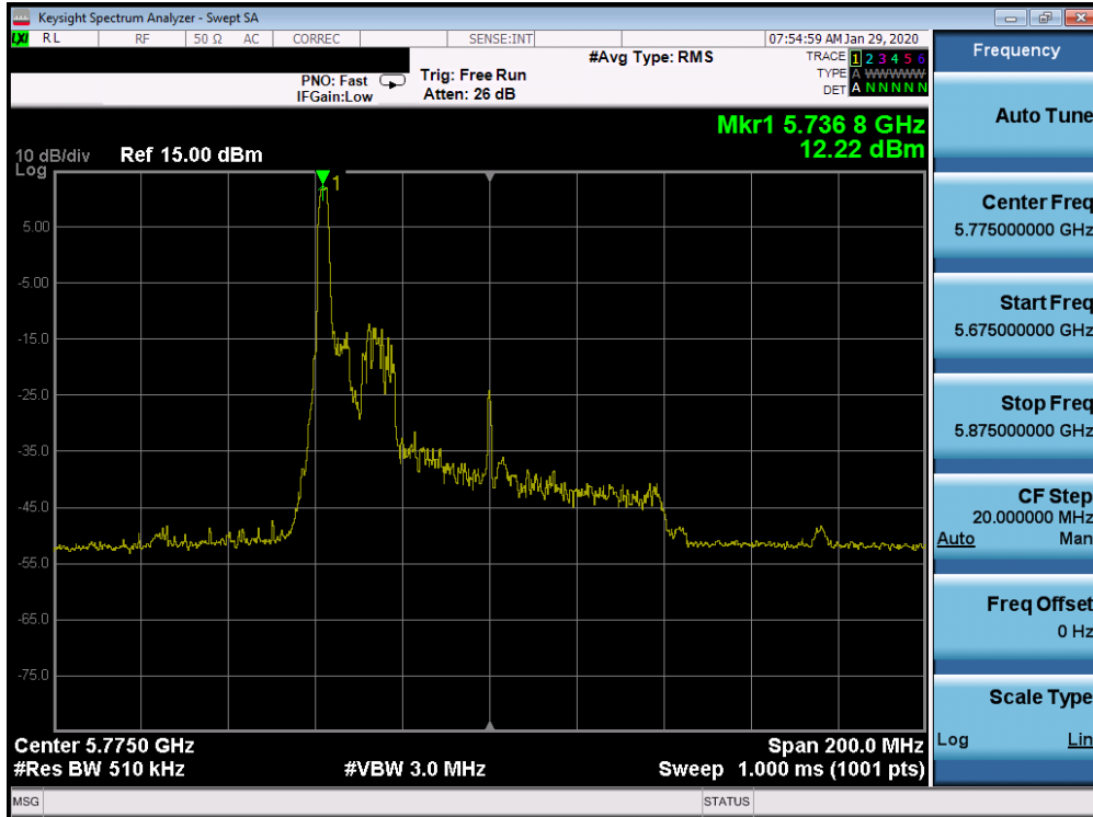
Plot 7-434. Power Spectral Density Plot SISO CORE 1 (80MHz BW 802.11ax Index 0 – RU26 (UNII Band 3) – Ch. 155)
