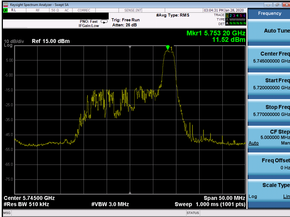
Plot 7-416. Power Spectral Density Plot SISO CORE 1 (20MHz BW 802.11ax Index 8 – RU26 (UNII Band 3) – Ch. 149)
