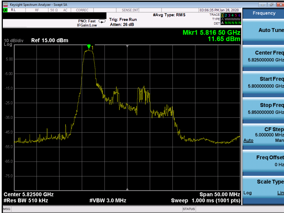
Plot 7-420. Power Spectral Density Plot SISO CORE 1 (20MHz BW 802.11ax Index 0 – RU26 (UNII Band 3) – Ch. 165)
