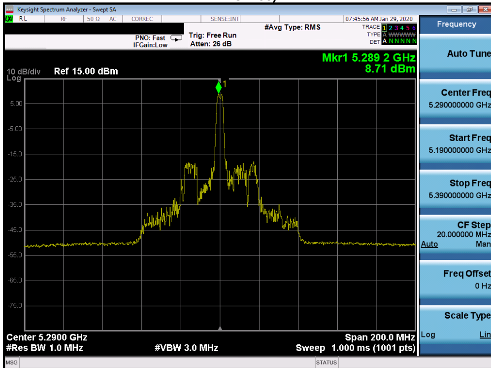
Plot 7-379. Power Spectral Density Plot SISO CORE 1 (80MHz BW 802.11ax Index 18 – RU26 (UNII Band 2A) – Ch. 58)
