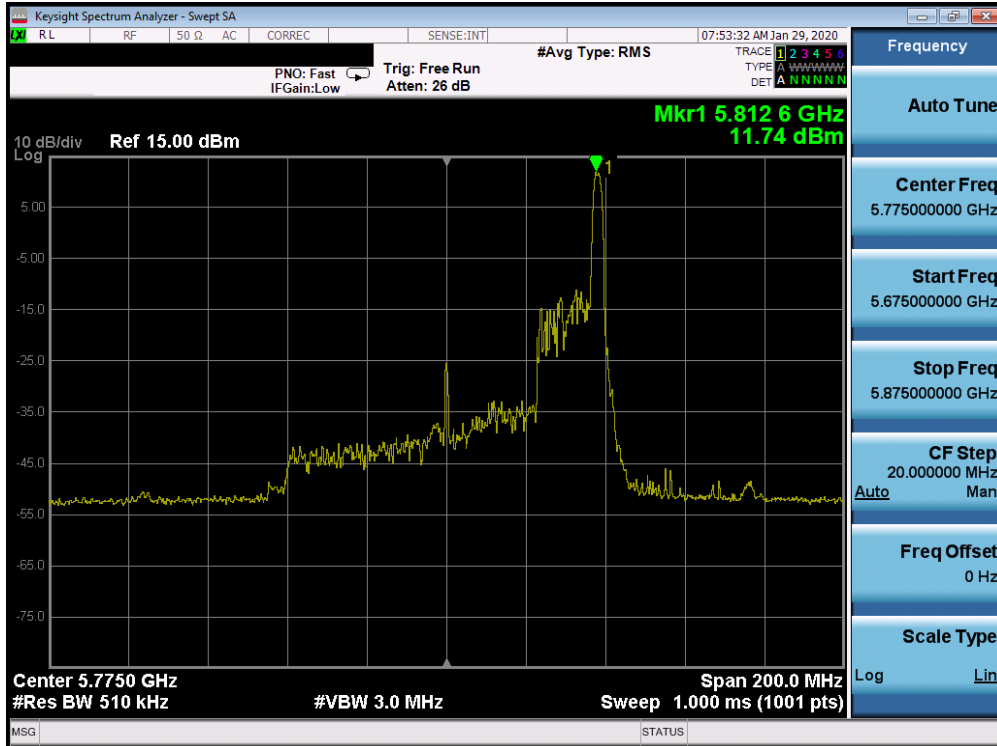
Plot 7-436. Power Spectral Density Plot SISO CORE 1 (80MHz BW 802.11ax Index 36 – RU26 (UNII Band 3) – Ch. 155)
