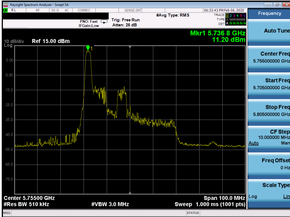
Plot 7-426. Power Spectral Density Plot SISO CORE 1 (40MHz BW 802.11ax Index 0 – RU26 (UNII Band 3) – Ch. 151)
