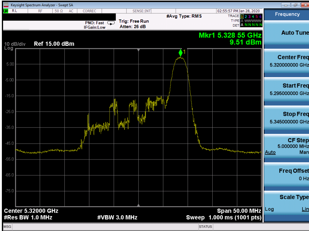
Plot 7-366. Power Spectral Density Plot SISO CORE 1 (20MHz BW 802.11ax Index 8 – RU26 (UNII Band 2A) – Ch. 64)
