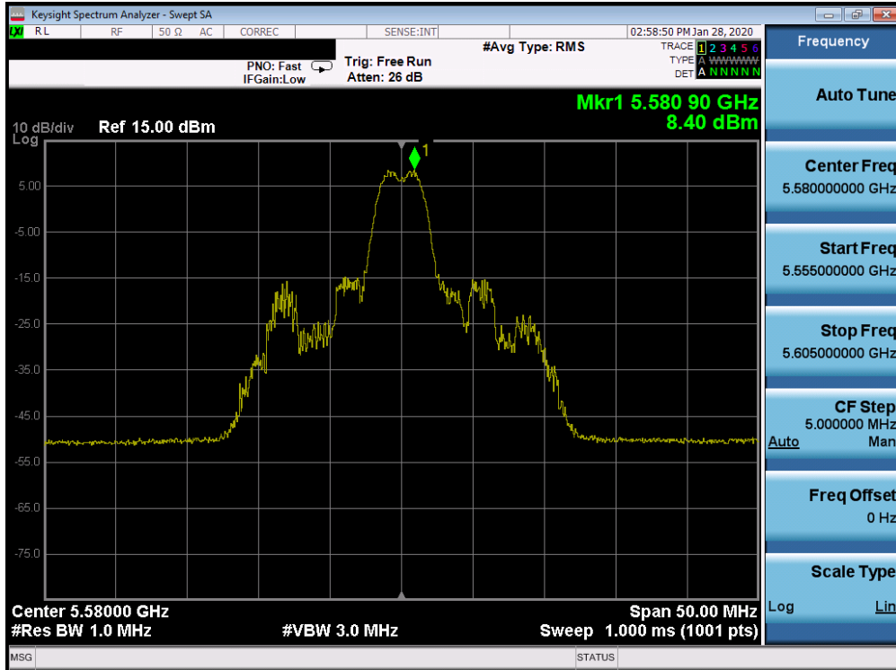
Plot 7-386. Power Spectral Density Plot SISO CORE 1 (20MHz BW 802.11ax Index 4 – RU26 (UNII Band 2C) – Ch. 116)
