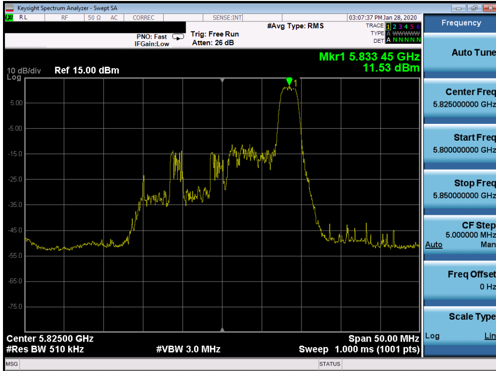
Plot 7-422. Power Spectral Density Plot SISO CORE 1 (20MHz BW 802.11ax Index 8 – RU26 (UNII Band 3) – Ch. 165)
