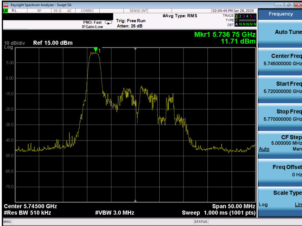
Plot 7-310. Power Spectral Density Plot SISO CORE 0 (20MHz BW 802.11ax Index 0 – RU26 (UNII Band 3) – Ch. 149)
