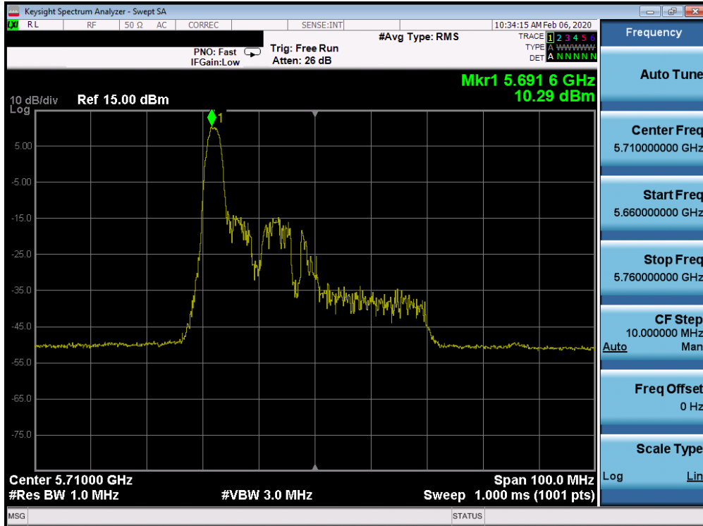
Plot 7-275. Power Spectral Density Plot SISO CORE 0 (40MHz BW 802.11ax Index 0 – RU26 (UNII Band 2C) – Ch. 142)
