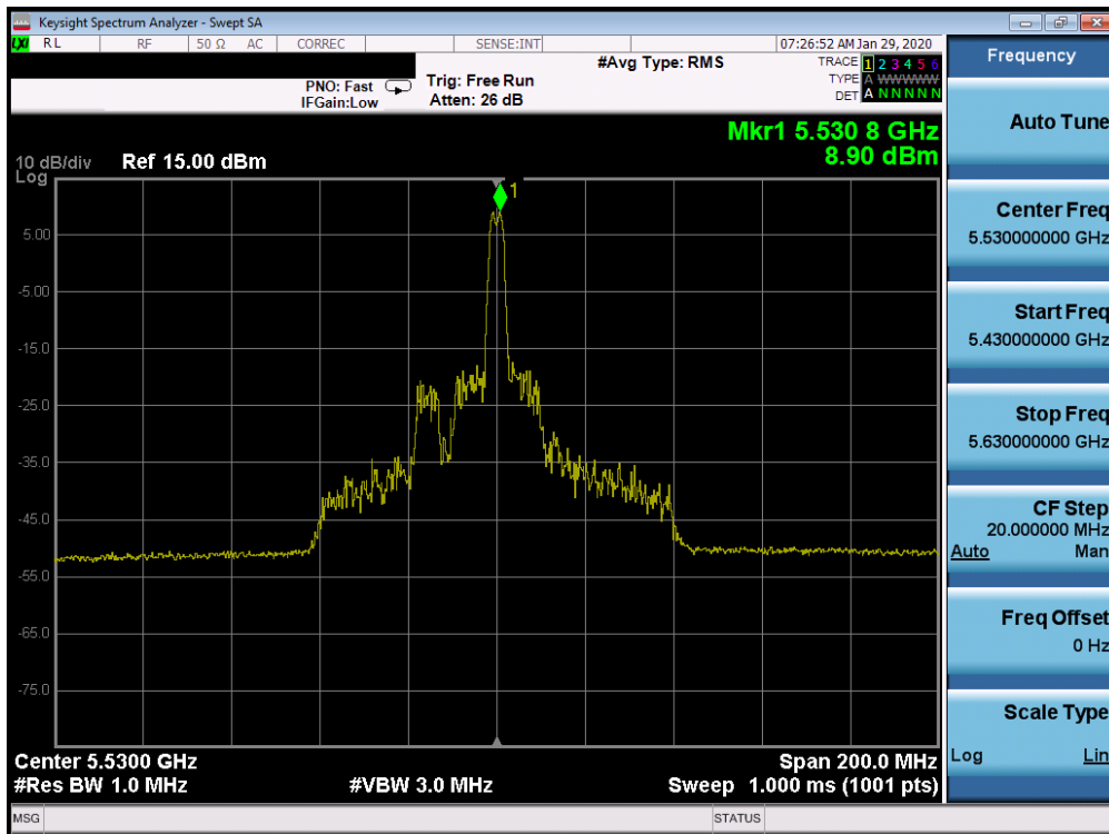
Plot 7-282. Power Spectral Density Plot SISO CORE 0 (80MHz BW 802.11ax Index 18 – RU26 (UNII Band 2C) – Ch. 106)
