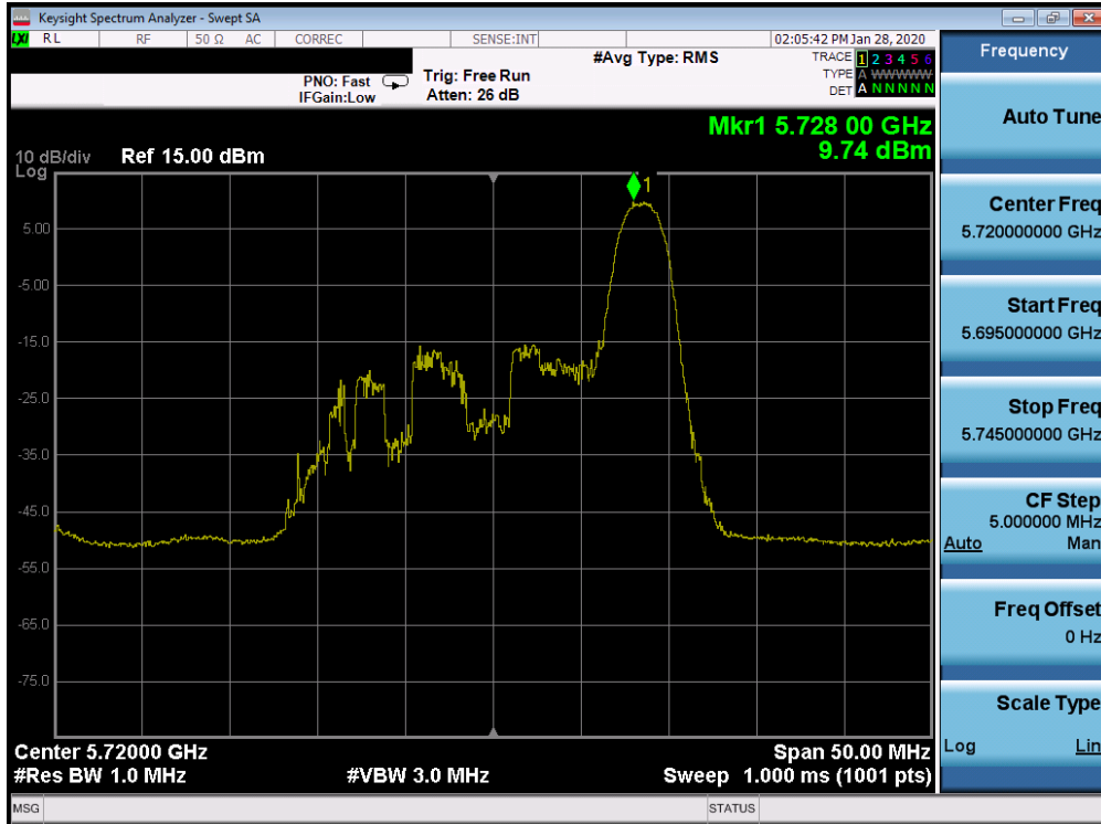
Plot 7-265. Power Spectral Density Plot SISO CORE 0 (20MHz BW 802.11ax Index 8 – RU26 (UNII Band 2C) – Ch. 144)
