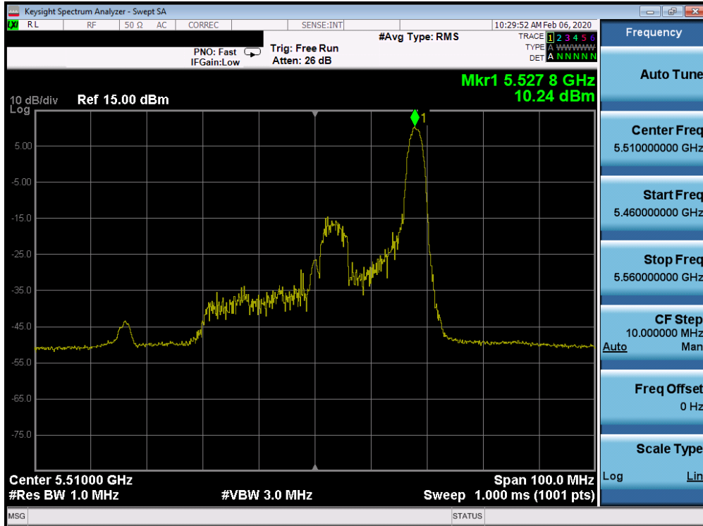
Plot 7-271. Power Spectral Density Plot SISO CORE 0 (40MHz BW 802.11ax Index 17 – RU26 (UNII Band 2C) – Ch. 102)
