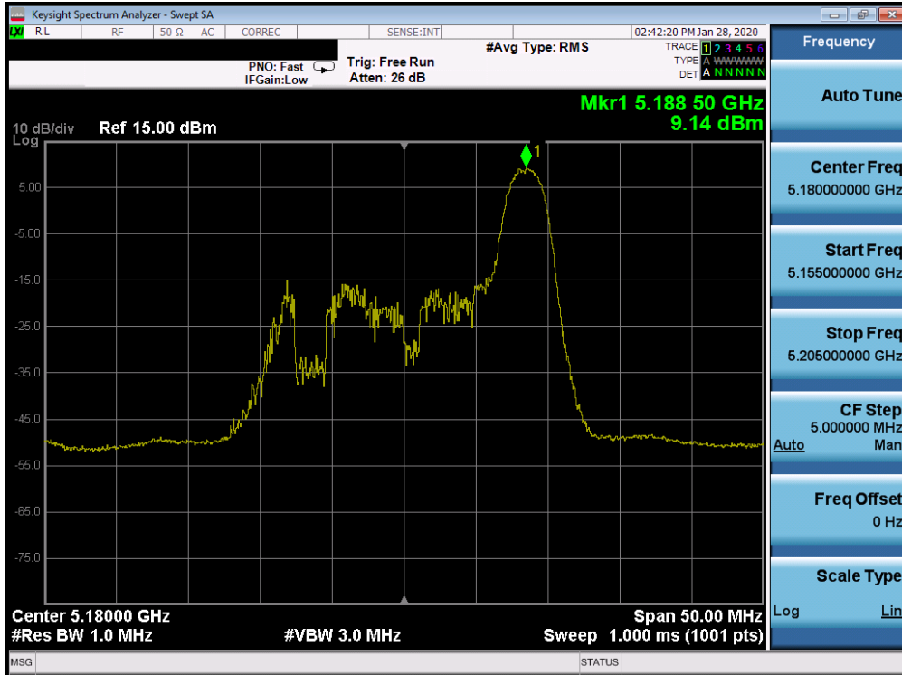
Plot 7-336. Power Spectral Density Plot SISO CORE 1 (20MHz BW 802.11ax Index 8 – RU26 (UNII Band 1) – Ch. 36)
