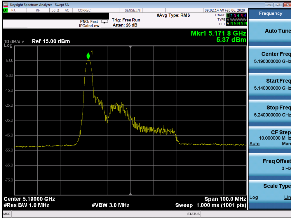
Plot 7-301. Power Spectral Density ISED Plot SISO CORE 0 (40MHz BW 802.11ax Index 0 – RU26 (UNII Band 1) – Ch. 38)
