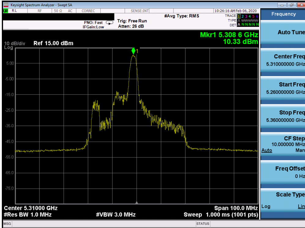
Plot 7-249. Power Spectral Density Plot SISO CORE 0 (40MHz BW 802.11ax Index 8 – RU26 (UNII Band 2A) – Ch. 62)
