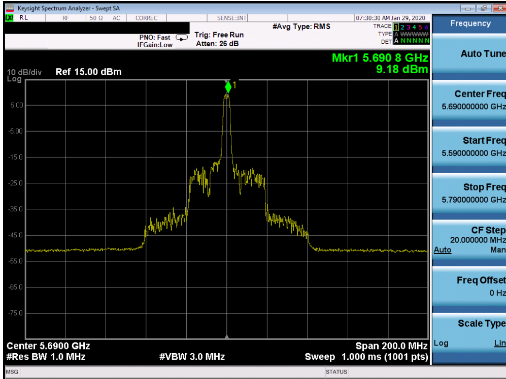
Plot 7-285. Power Spectral Density Plot SISO CORE 0 (80MHz BW 802.11ax Index 18 – RU26 (UNII Band 2C) – Ch. 138)
