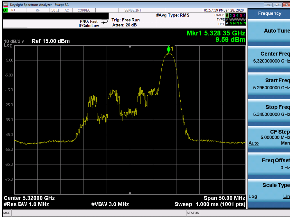
Plot 7-241. Power Spectral Density Plot SISO CORE 0 (20MHz BW 802.11ax Index 8 – RU26 (UNII Band 2A) – Ch. 64)
