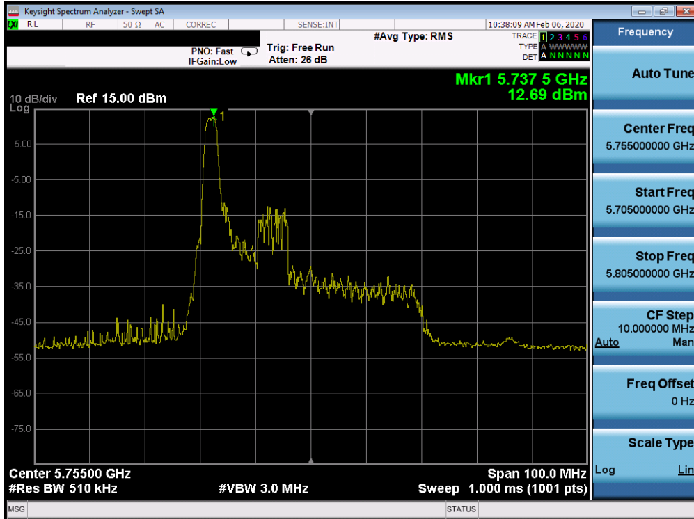
Plot 7-322. Power Spectral Density Plot SISO CORE 0 (40MHz BW 802.11ax Index 0 – RU26 (UNII Band 3) – Ch. 151)
