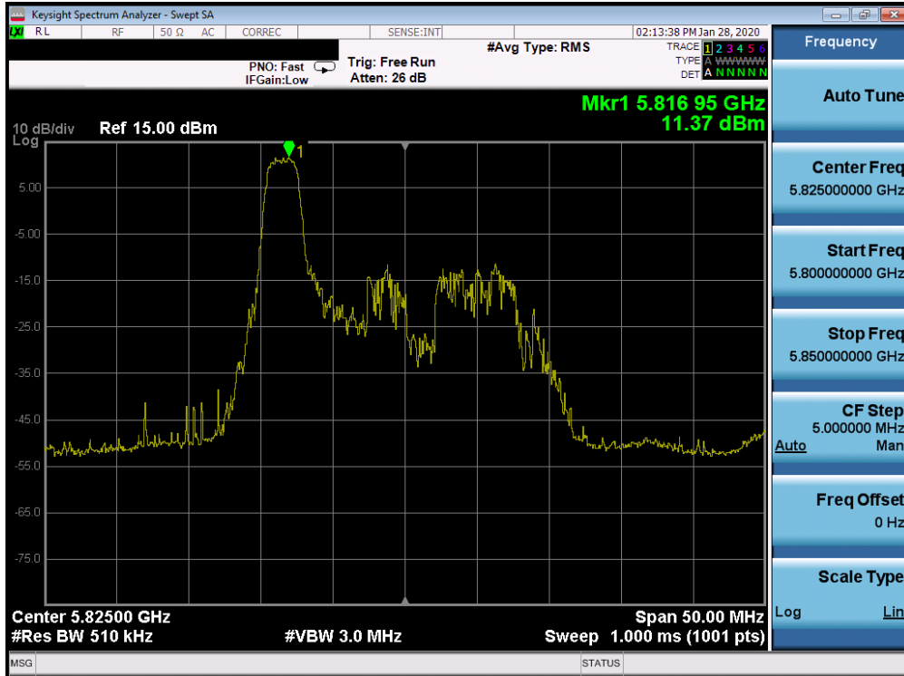
Plot 7-316. Power Spectral Density Plot SISO CORE 0 (20MHz BW 802.11ax Index 0 – RU26 (UNII Band 3) – Ch. 165)
