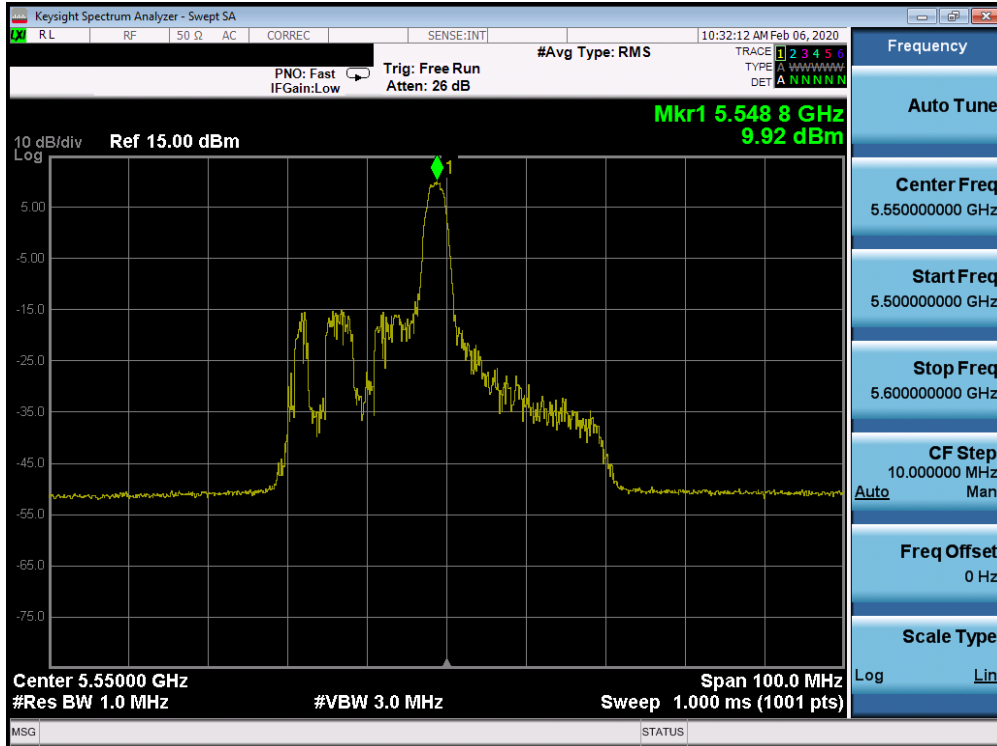
Plot 7-273. Power Spectral Density Plot SISO CORE 0 (40MHz BW 802.11ax Index 8 – RU26 (UNII Band 2C) – Ch. 110)
