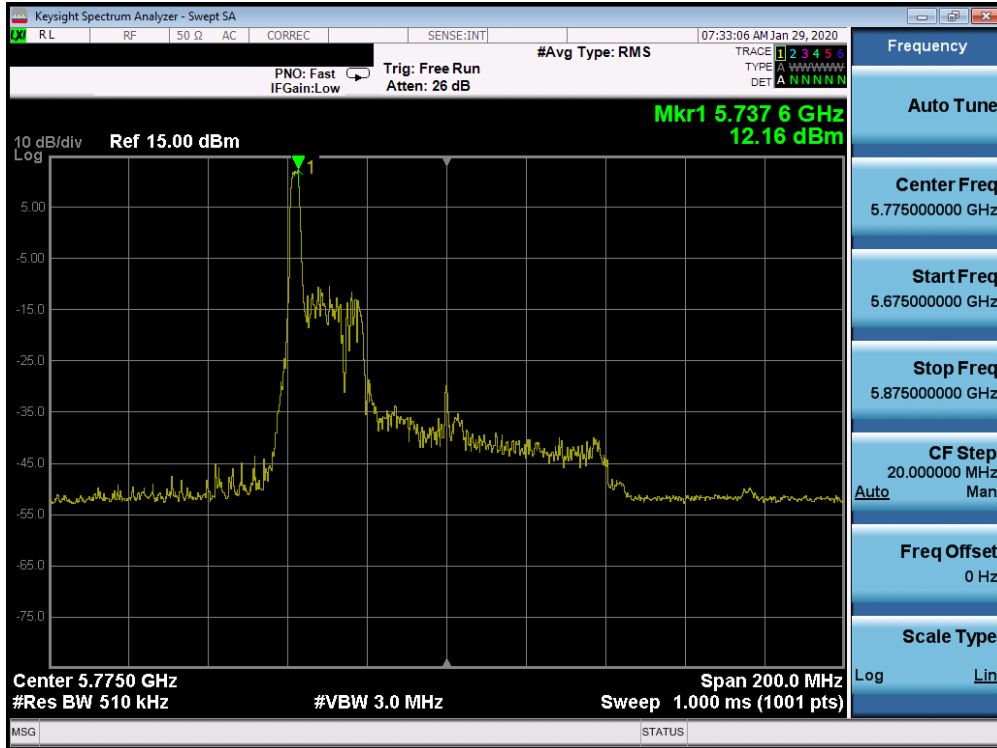
Plot 7-330. Power Spectral Density Plot SISO CORE 0 (80MHz BW 802.11ax Index 0 – RU26 (UNII Band 3) – Ch. 155)
