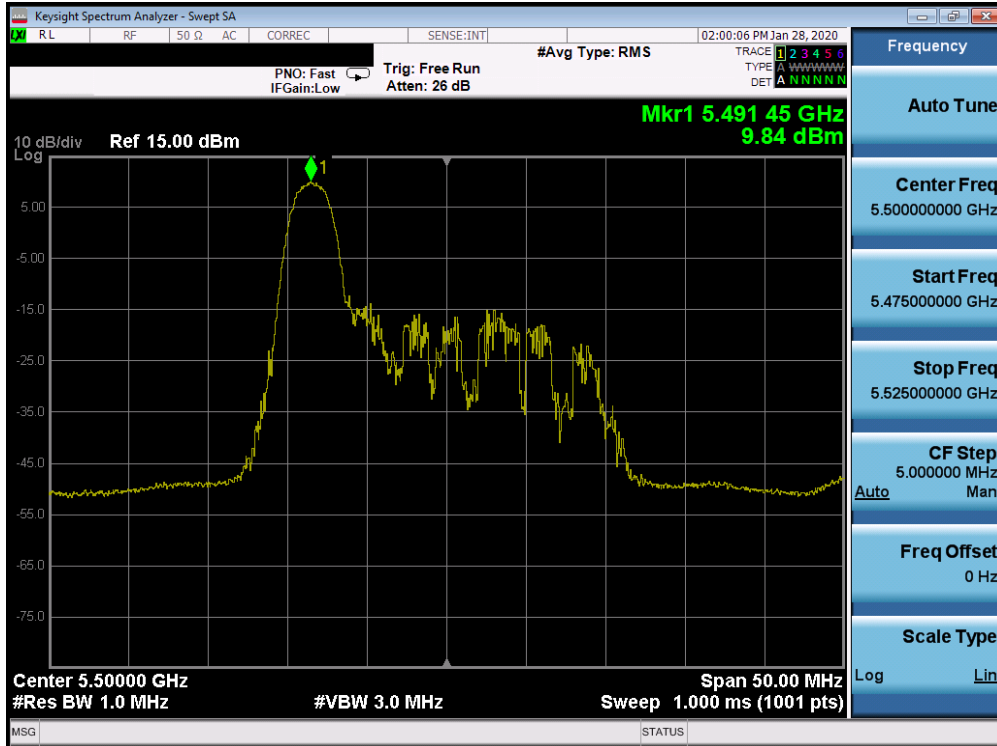
Plot 7-257. Power Spectral Density Plot SISO CORE 0 (20MHz BW 802.11ax Index 0 – RU26 (UNII Band 2C) – Ch. 100)
