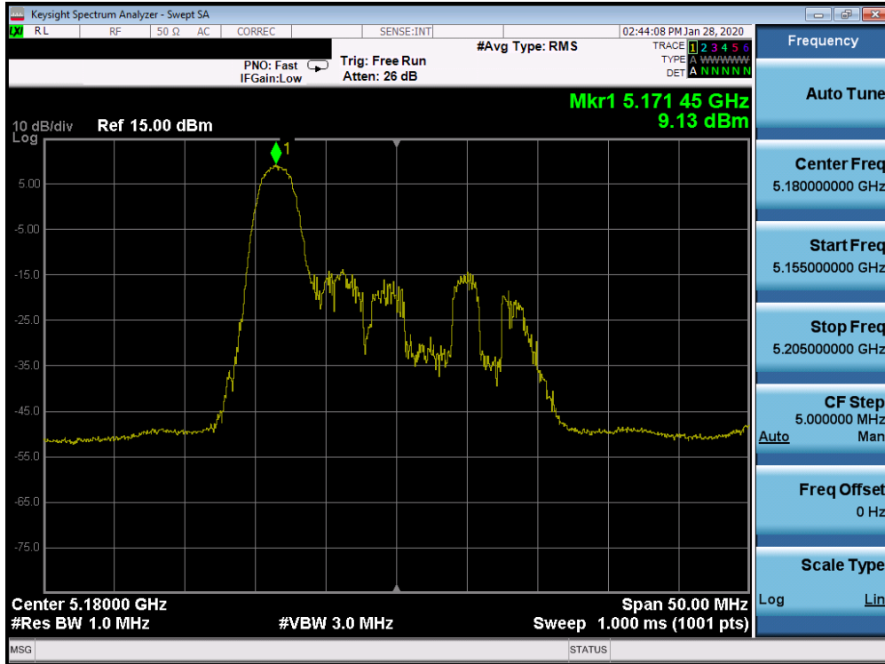
Plot 7-334. Power Spectral Density Plot SISO CORE 1 (20MHz BW 802.11ax Index 0 – RU26 (UNII Band 1) – Ch. 36)
