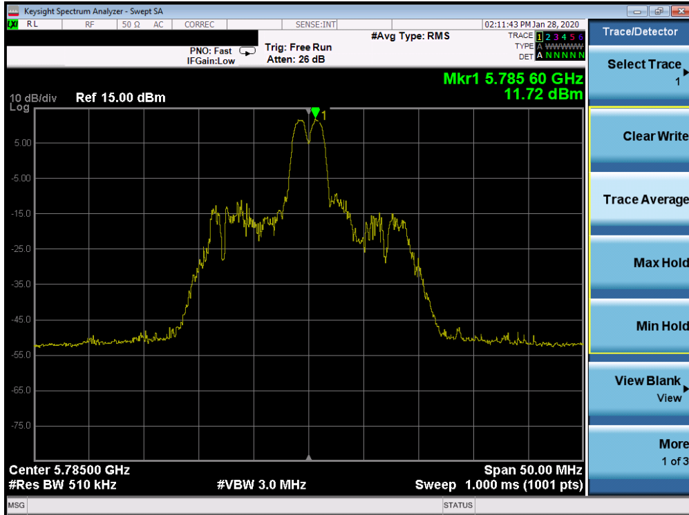
Plot 7-314. Power Spectral Density Plot SISO CORE 0 (20MHz BW 802.11ax Index 4 – RU26 (UNII Band 3) – Ch. 157)
