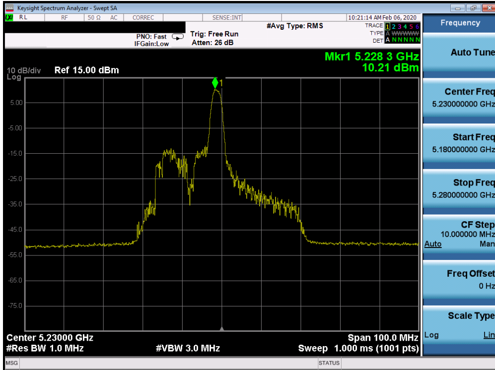
Plot 7-225. Power Spectral Density Plot SISO CORE 0 (40MHz BW 802.11ax Index 8 – RU26 (UNII Band 1) – Ch. 46)
