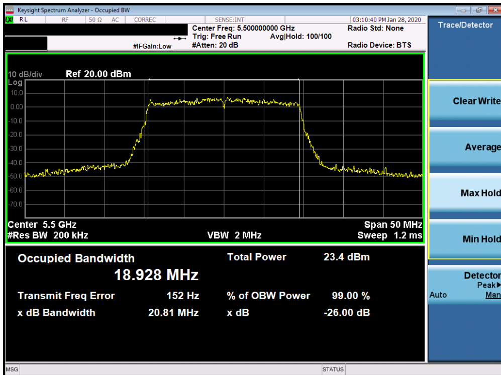
Plot 7-138. 26dB Bandwidth Plot SISO CORE 1 (20MHz BW 802.11ax– RU242 (UNII Band 2C) – Ch. 100)
