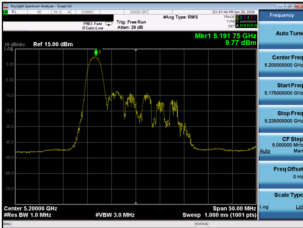
Plot 7-212. Power Spectral Density Plot SISO CORE 0 (20MHz BW 802.11ax Index 0 – RU26 (UNII Band 1) – Ch. 40)
