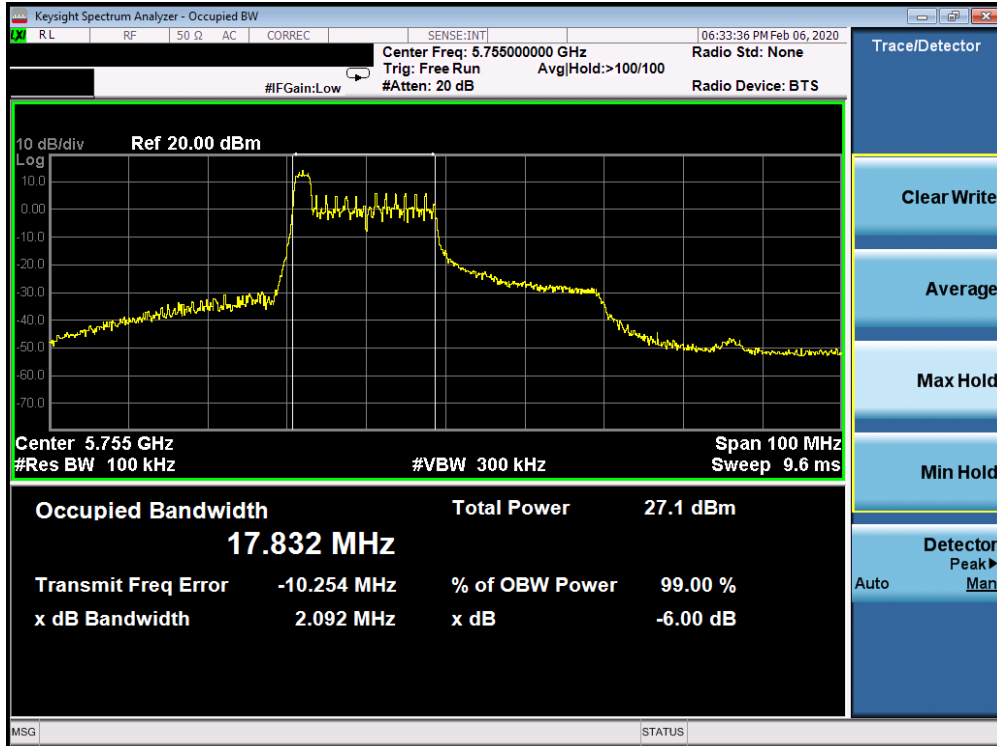
Plot 7-197. 6dB Bandwidth Plot SISO CORE 1 (40MHz BW 802.11ax Index 0 – RU26 (UNII Band 3) – Ch. 151)
