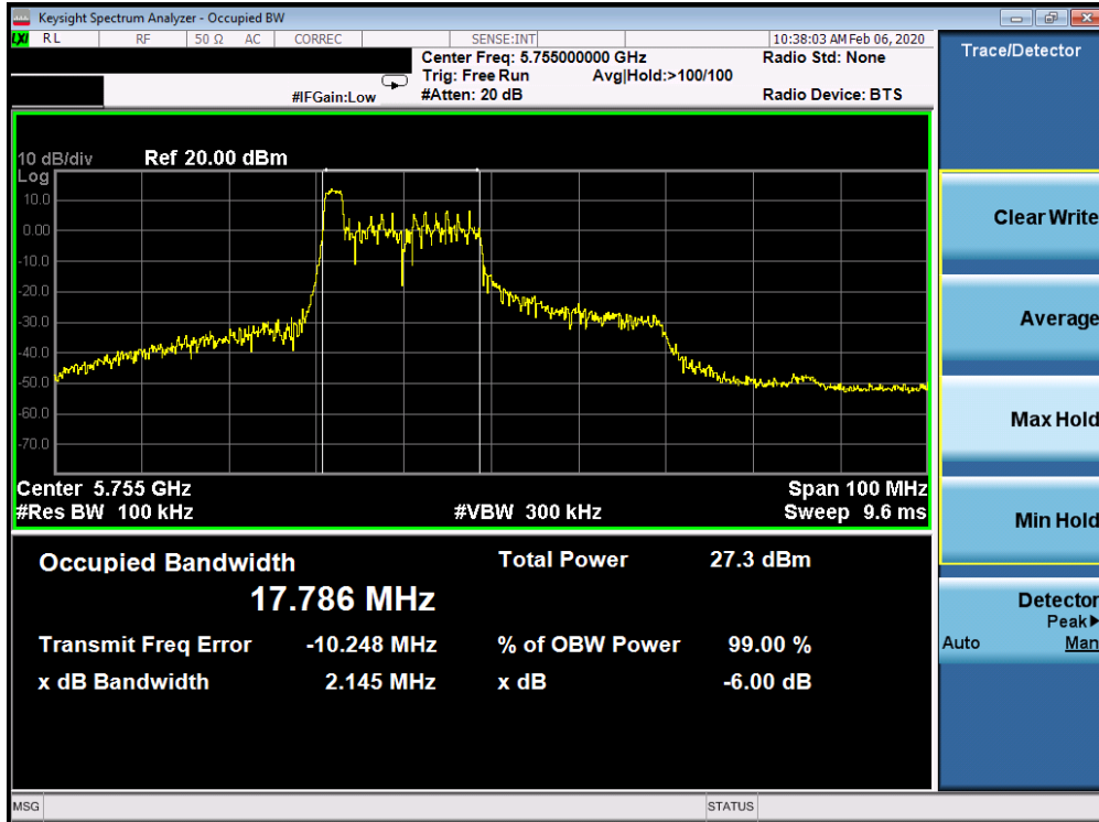
Plot 7-173. 6dB Bandwidth Plot SISO CORE 0 (40MHz BW 802.11ax Index 0 – RU26 (UNII Band 3) – Ch. 151)
