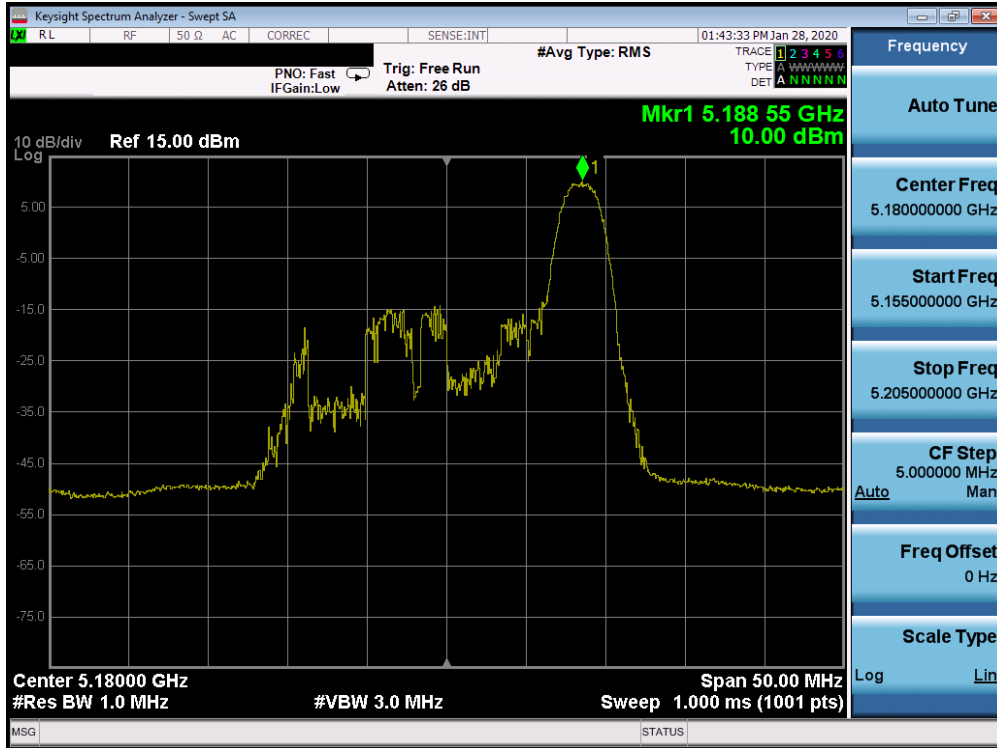
Plot 7-211. Power Spectral Density Plot SISO CORE 0 (20MHz BW 802.11ax Index 8 – RU26 (UNII Band 1) – Ch. 36)
