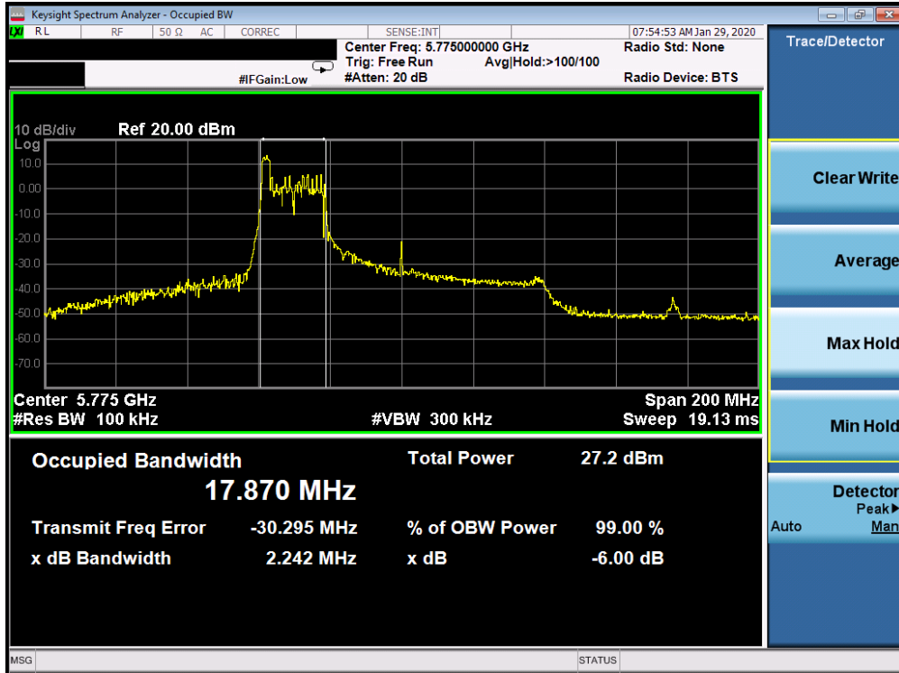
Plot 7-205. 6dB Bandwidth Plot SISO CORE 1 (80MHz BW 802.11ax Index 0 – RU26 (UNII Band 3) – Ch. 155)
