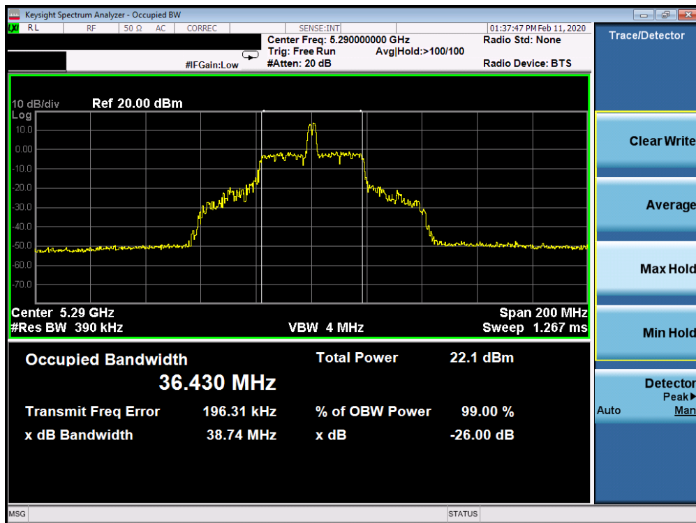
Plot 7-46. 26dB Bandwidth Plot SISO CORE 0 (80MHz BW 802.11ax Index 18 – RU26 (UNII Band 2A) – Ch. 58)
