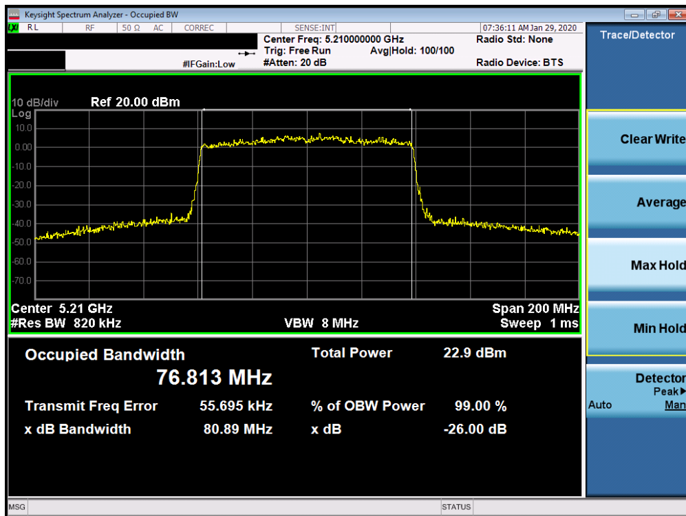
Plot 7-24. 26dB Bandwidth Plot SISO CORE 0 (80MHz BW 802.11ax – RU996 (UNII Band 1) – Ch. 42)
