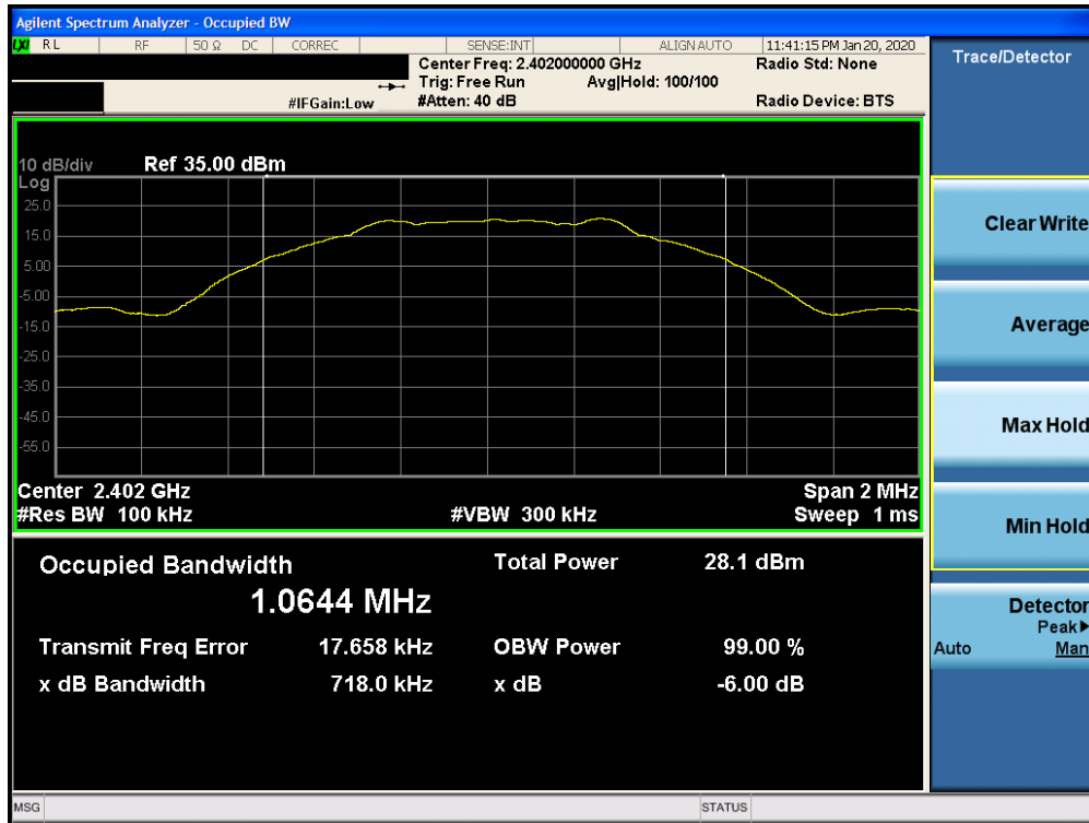
Plot 7-7. 6dB Bandwidth Plot Ant WF7 (Bluetooth (LE), 1Mbps, ePA – Ch. 0)
