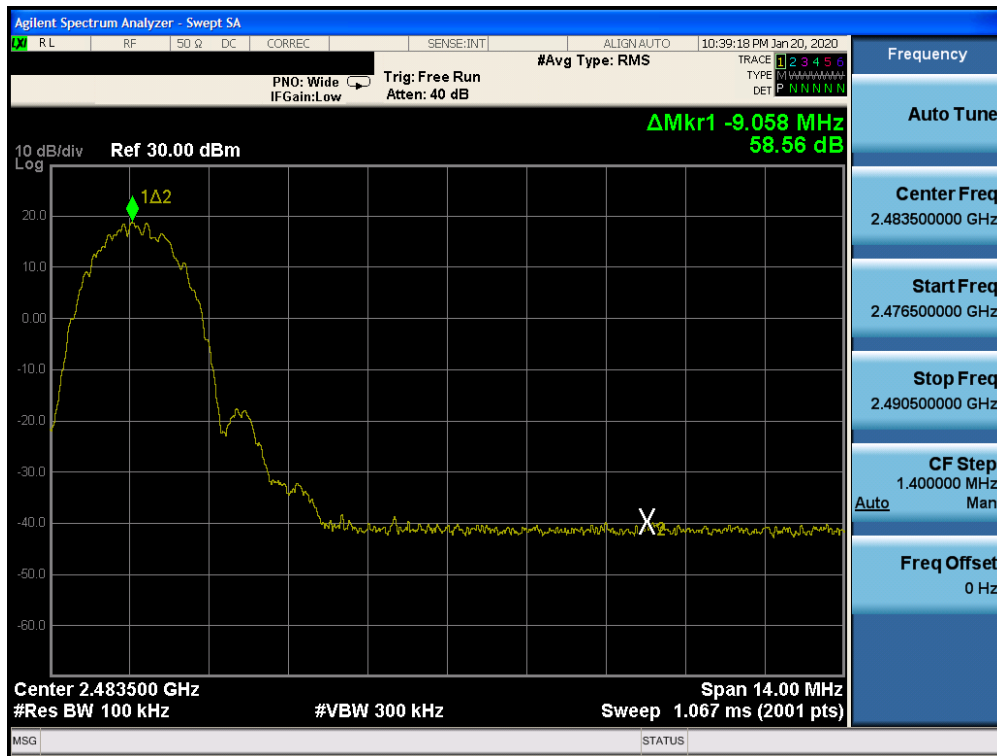
Plot 7-64. Band Edge Plot Ant WF8 (Bluetooth (LE), 2Mbps ePA – Ch. 38)
