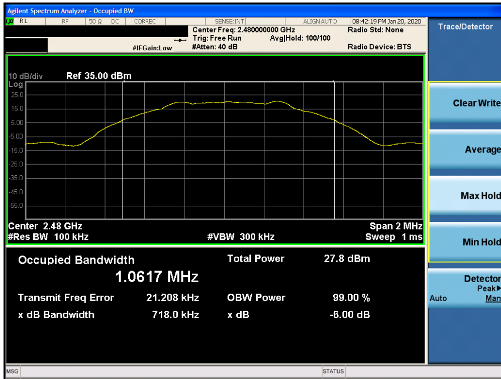
Plot 7-3. 6dB Bandwidth Plot Ant WF8 (Bluetooth (LE), 1Mbps, ePA – Ch. 39)
