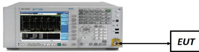
Figure 7-4. Test Instrument & Measurement Setup
