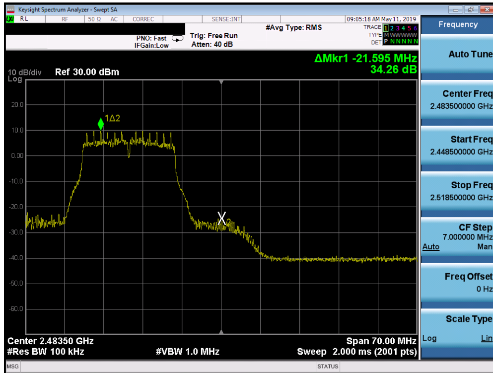
Plot 7-55. Band Edge Plot SISO CORE 0 (802.11g – Ch. 12)
