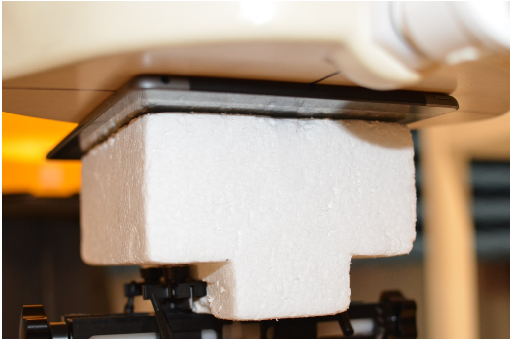
SAR Test Setup Photo 1: Back Side at 0.0 cm – Antenna C/Antenna D
