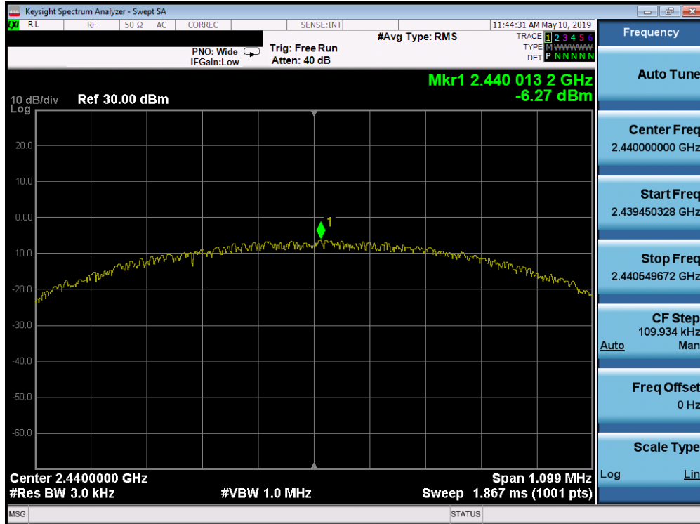
Plot 7-11. Power Spectral Density Plot (Bluetooth (LE), iPA – Ch. 19)
