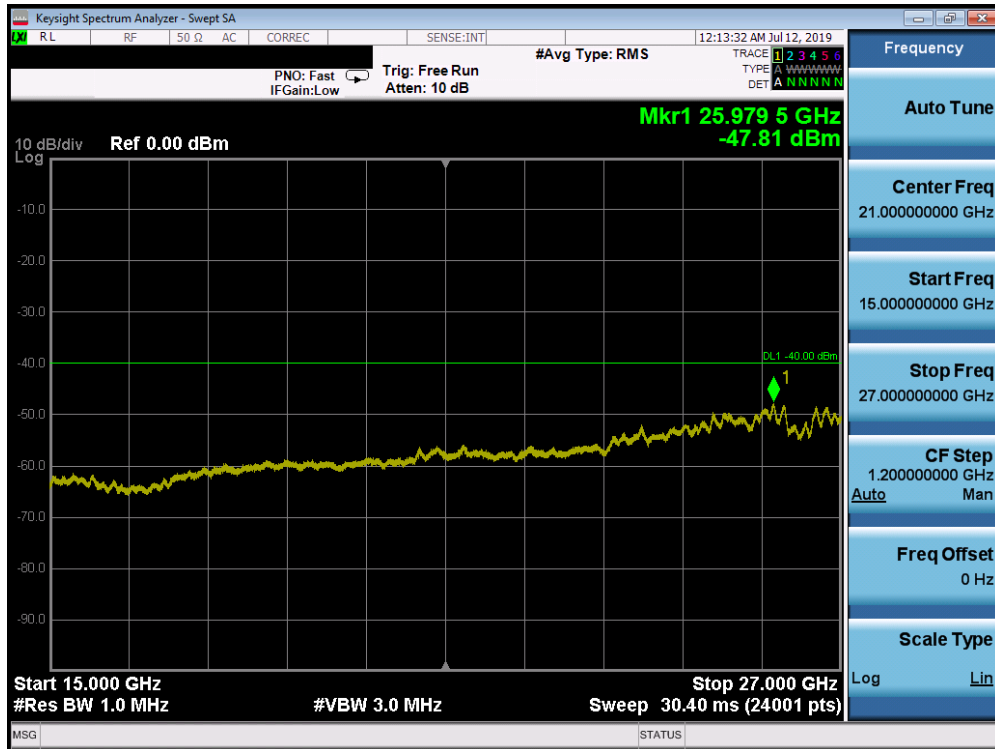
Plot 7-171. Conducted Spurious Plot (Band 30 - 5.0MHz QPSK - RB Size 1, RB Offset 0 - High Channel)
