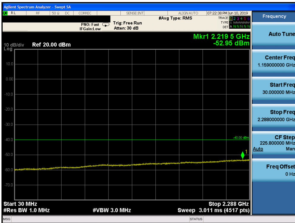
Plot 7-166. Conducted Spurious Plot (Band 30 - 10.0MHz QPSK - RB Size 1, RB Offset 0 - Mid Channel)
