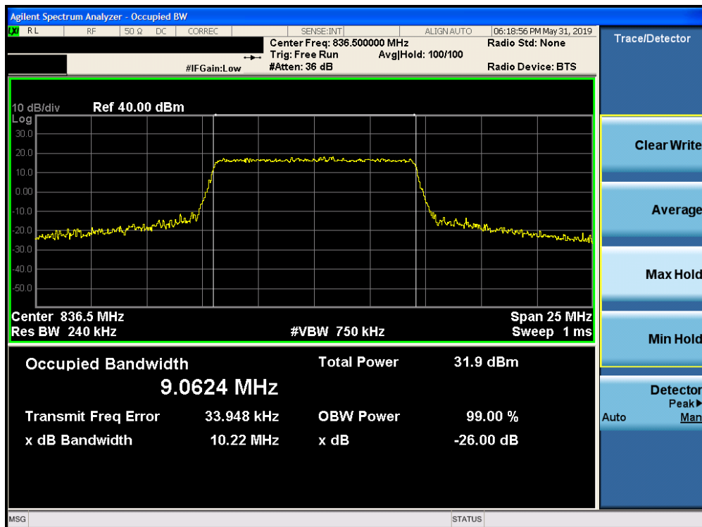
Plot 7-42. Occupied Bandwidth Plot (Band 26/5 - 10.0MHz 64-QAM - Full RB Configuration)
