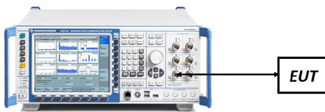
Figure 7-5. ERP/EIRP Measurement Setup
