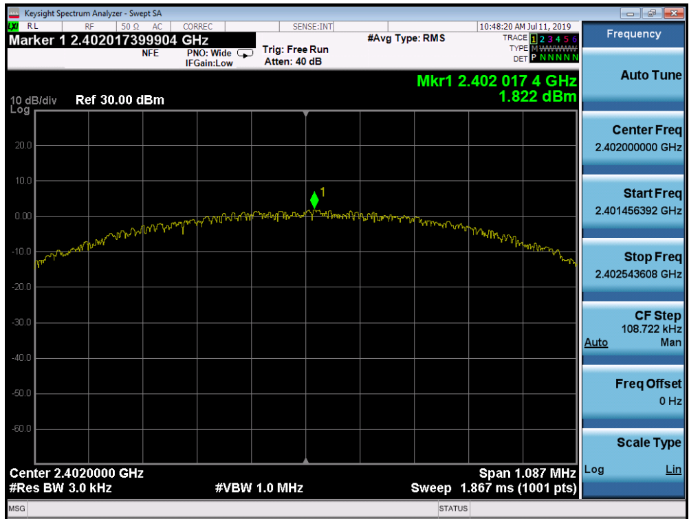
Plot 7-7. Power Spectral Density Plot (Bluetooth (LE), ePA – Ch. 0)
