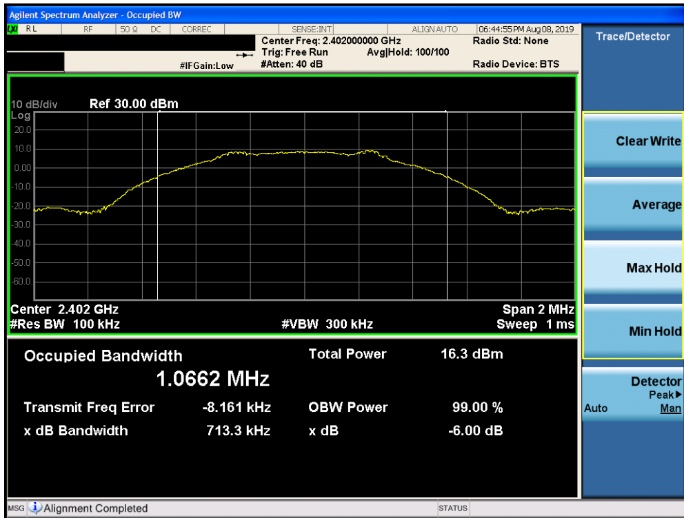
Plot 7-4. 6dB Bandwidth Plot (Bluetooth (LE), iPA – Ch. 0)
