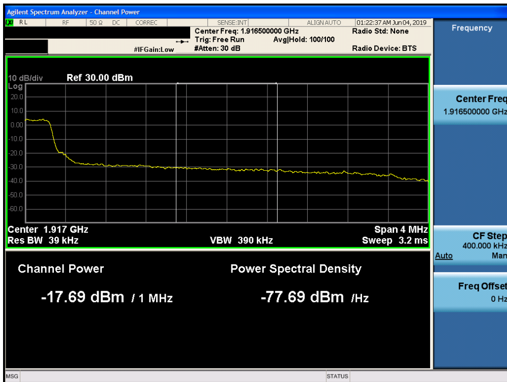
Plot 7-260. Upper Extended Band Edge Plot (Band 25 - 5.0MHz QPSK - Full RB Configuration)
