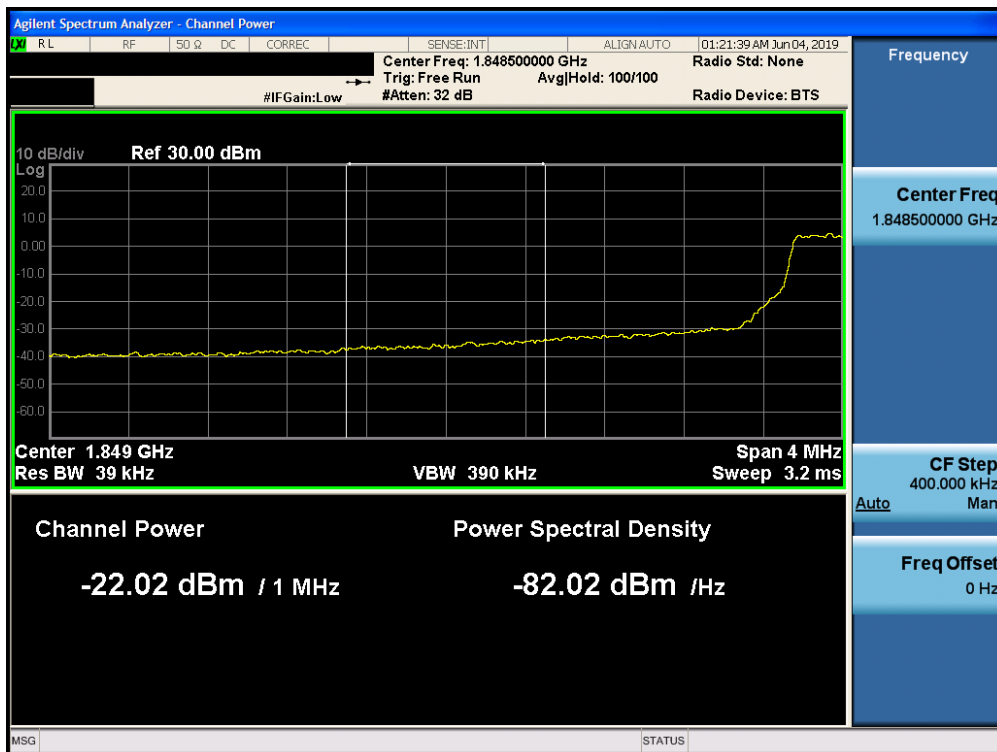
Plot 7-258. Lower Extended Band Edge Plot (Band 25 - 5.0MHz QPSK - Full RB Configuration)
