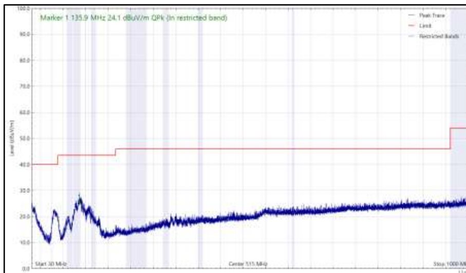
Figure 14- 2405 MHz (CH11), Thread, 30 MHz to 1 GHz, Vertical (Peak)
