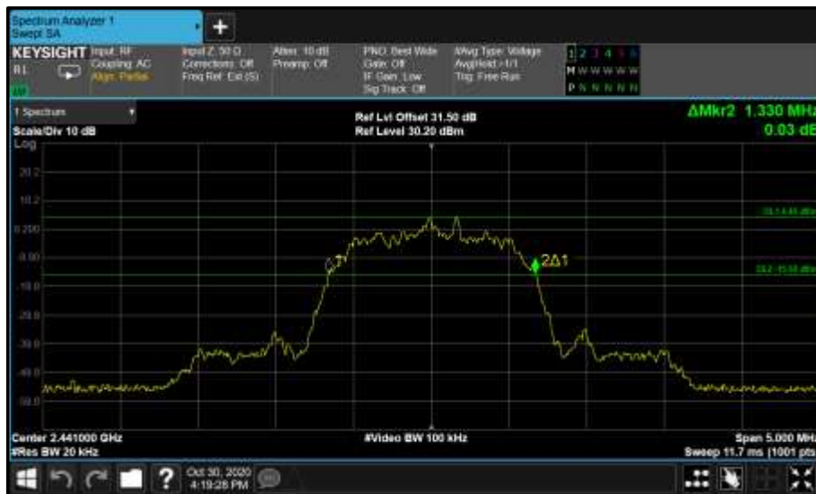
Figure 66 - Core1 \pi/4 DQPSK 2441 MHz (CH39) 20 dB Bandwidth
