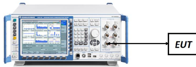
Figure 7-5. Conducted Power Measurement Setup
