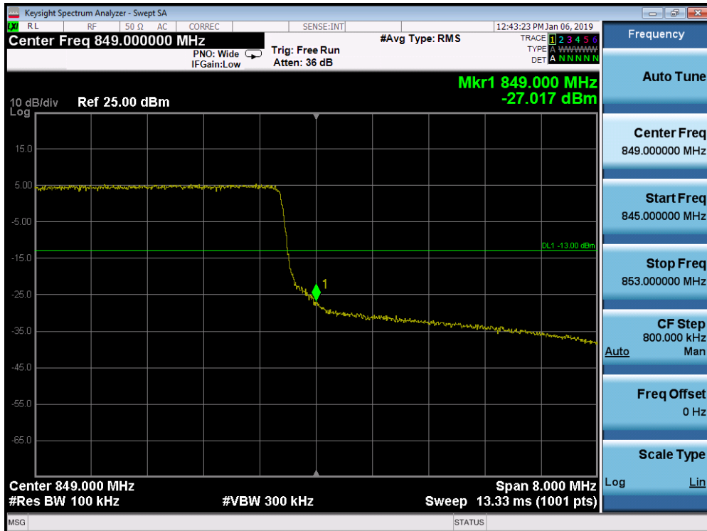
Plot 7-229. Upper Band Edge Plot (Band 5 - 10.0MHz QPSK - Full RB Configuration)
