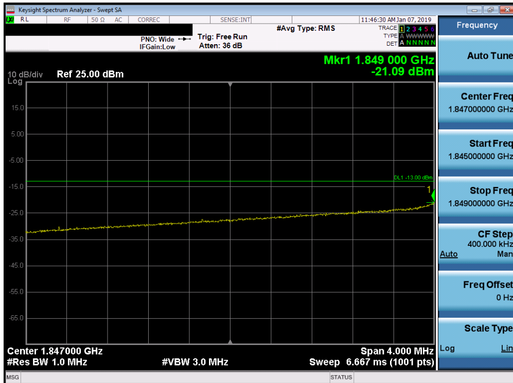
Plot 7-291. Lower Extended Band Edge Plot (Band 25 - 10.0MHz QPSK - Full RB Configuration)
