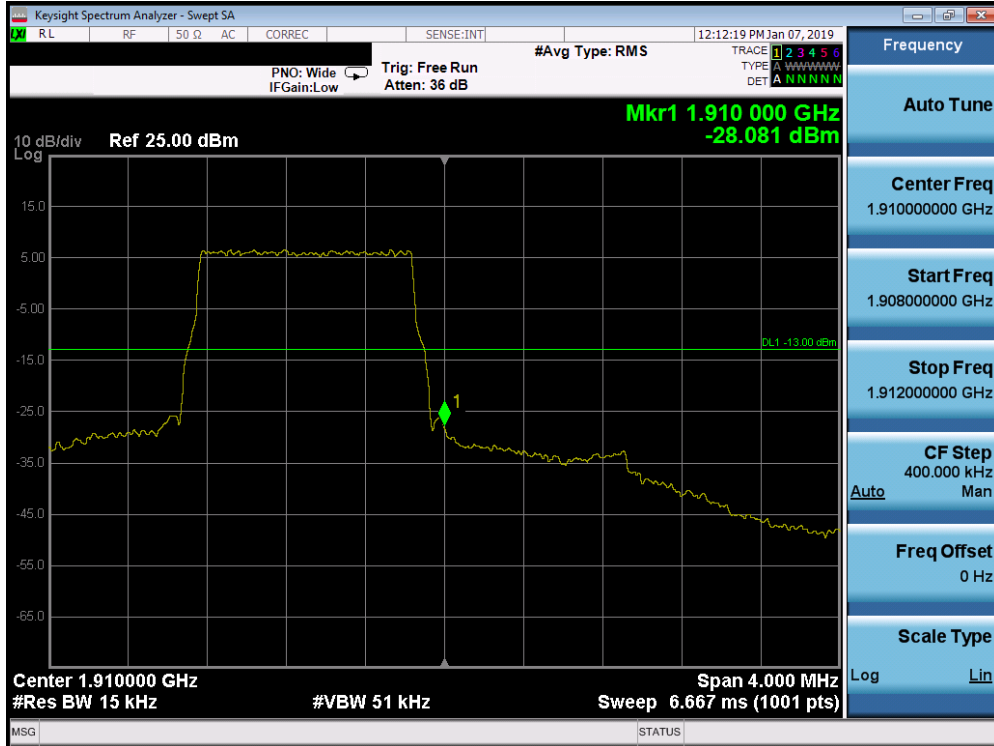
Plot 7-304. Upper Band Edge Plot (Band 2 - 1.4MHz QPSK - Full RB Configuration)
