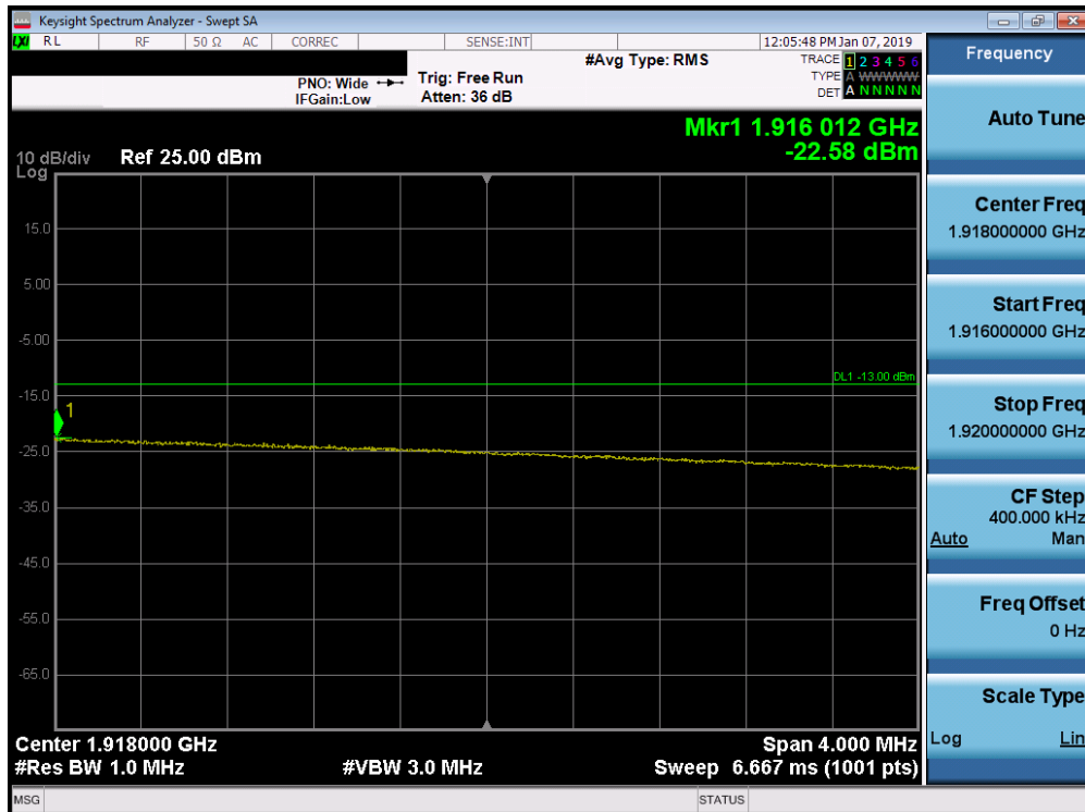
Plot 7-301. Upper Extended Band Edge Plot (Band 25 - 20.0MHz QPSK - Full RB Configuration)
