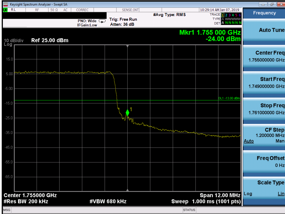
Plot 7-272. Upper Band Edge Plot (Band 4 - 15.0MHz QPSK - Full RB Configuration)
