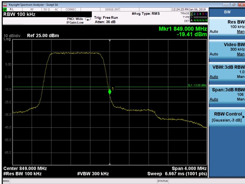
Plot 7-223. Upper Band Edge Plot (Band 5 - 1.4MHz QPSK - Full RB Configuration)
