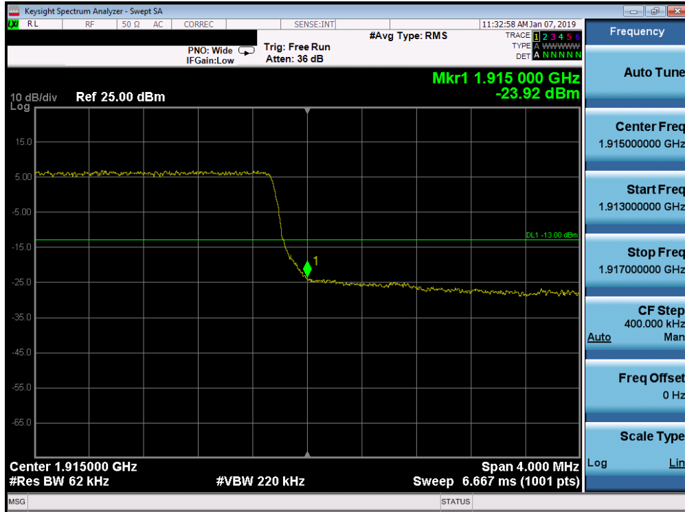
Plot 7-288. Upper Band Edge Plot (Band 25 - 5.0MHz QPSK - Full RB Configuration)
