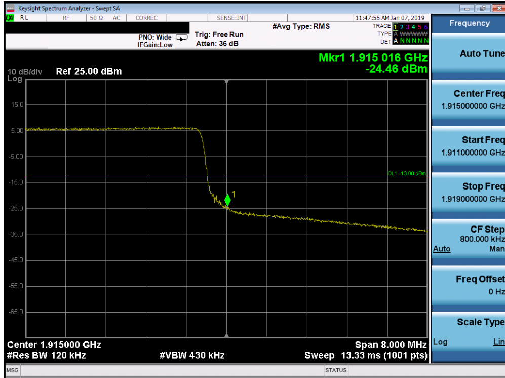
Plot 7-292. Upper Band Edge Plot (Band 25 - 10.0MHz QPSK - Full RB Configuration)
