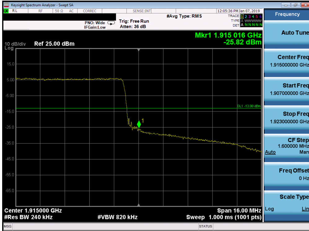
Plot 7-300. Upper Band Edge Plot (Band 25 - 20.0MHz QPSK - Full RB Configuration)
