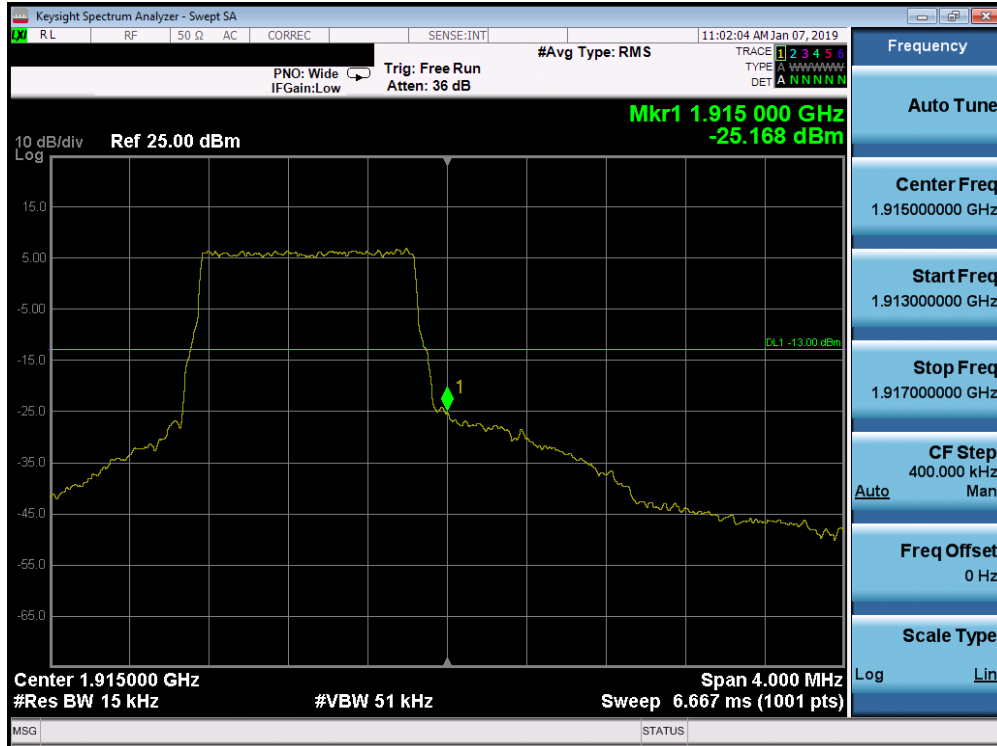
Plot 7-280. Upper Band Edge Plot (Band 25 - 1.4MHz QPSK - Full RB Configuration)
