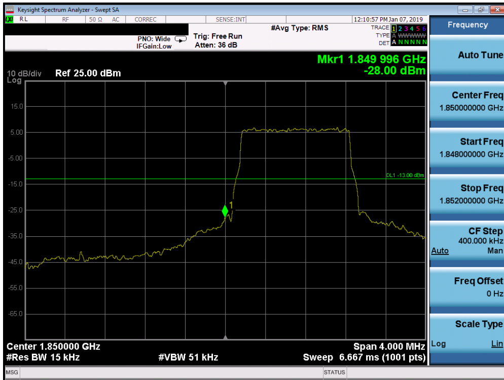
Plot 7-302. Lower Band Edge Plot (Band 2 - 1.4MHz QPSK - Full RB Configuration)
