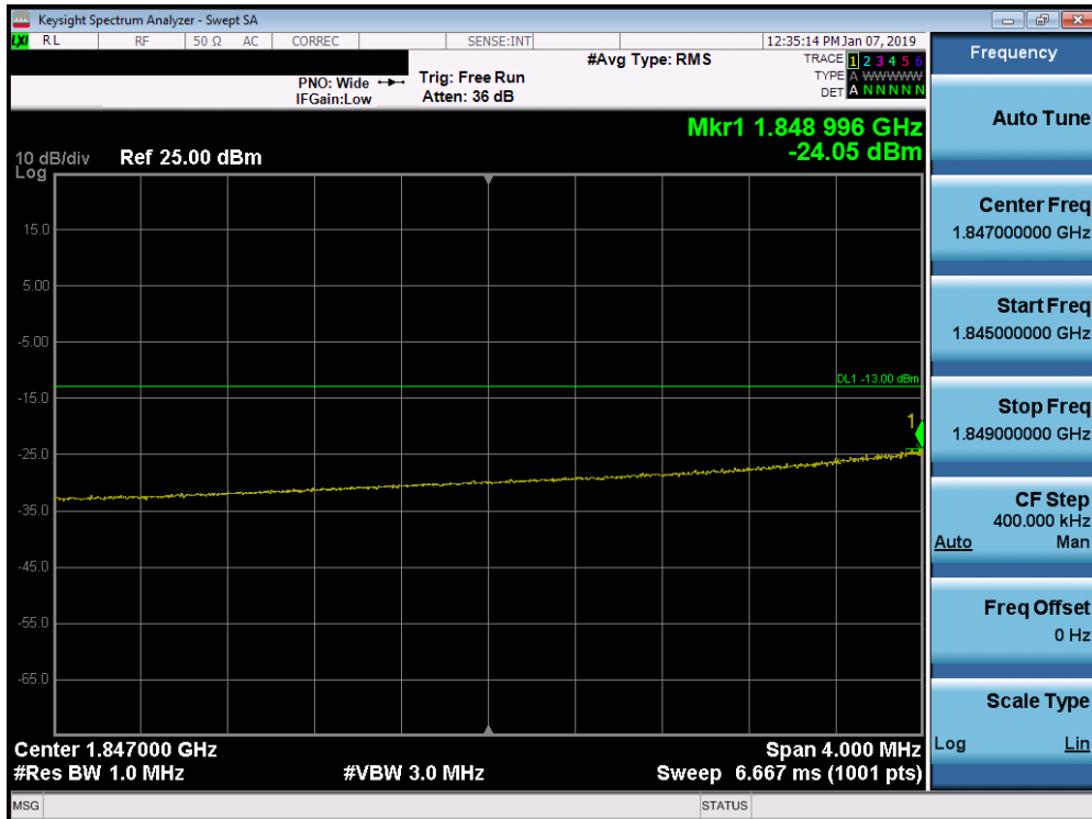
Plot 7-319. Lower Extended Band Edge Plot (Band 2 - 15.0MHz QPSK - Full RB Configuration)
