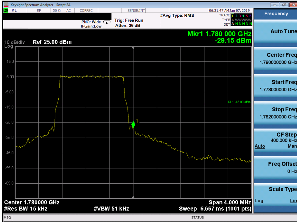
Plot 7-232. Upper Band Edge Plot (Band 66 - 1.4MHz QPSK - Full RB Configuration)
