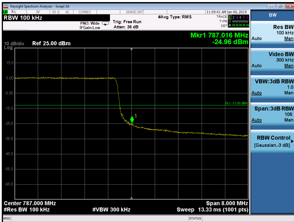
Plot 7-213. Upper Band Edge Plot (Band 13 - 10.0MHz QPSK - Full RB Configuration)
