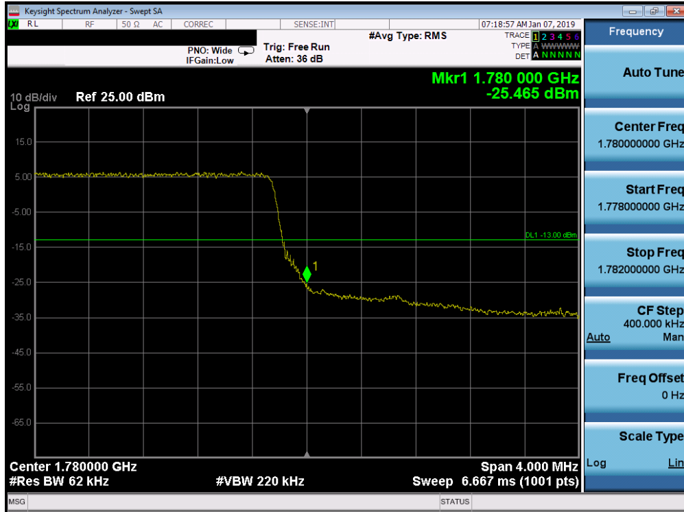
Plot 7-240. Upper Band Edge Plot (Band 66 - 5.0MHz QPSK - Full RB Configuration)
