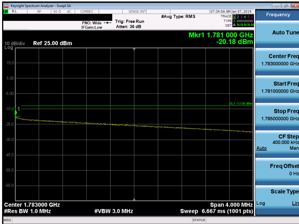
Plot 7-245. Upper Extended Band Edge Plot (Band 66 - 10.0MHz QPSK - Full RB Configuration)
