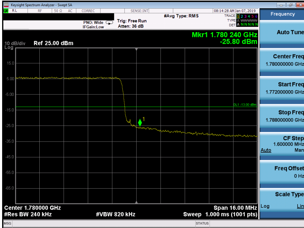
Plot 7-252. Upper Band Edge Plot (Band 66 - 20.0MHz QPSK - Full RB Configuration)
