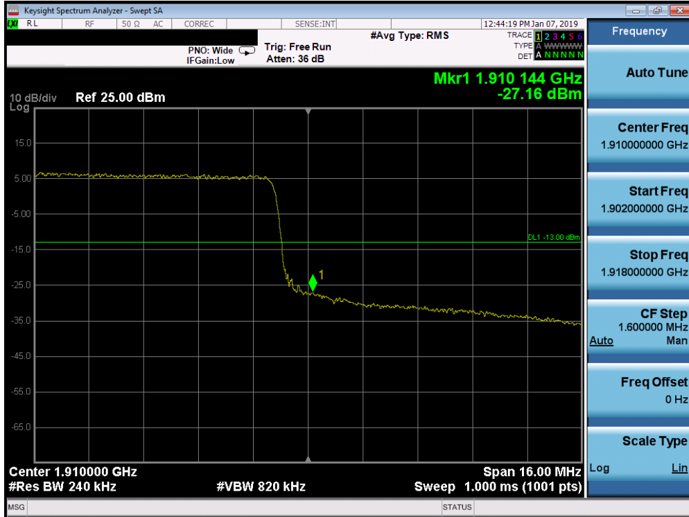
Plot 7-324. Upper Band Edge Plot (Band 2 - 20.0MHz QPSK - Full RB Configuration)
