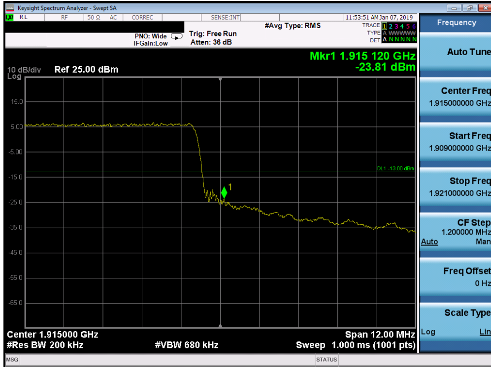
Plot 7-296. Upper Band Edge Plot (Band 25 - 15.0MHz QPSK - Full RB Configuration)
