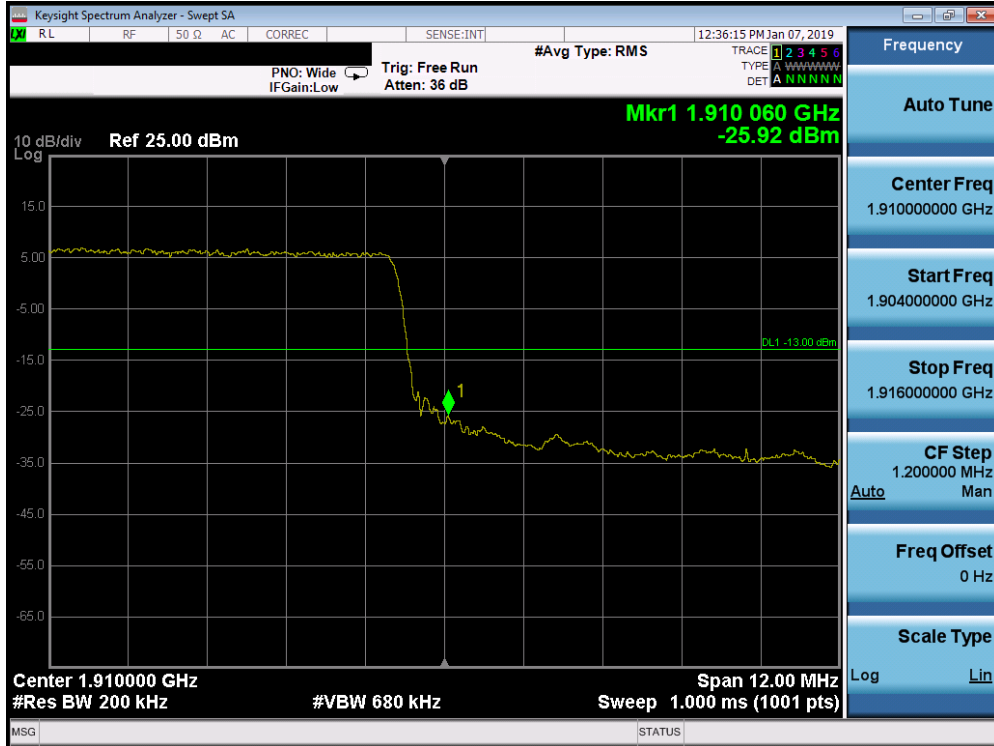
Plot 7-320. Upper Band Edge Plot (Band 2 - 15.0MHz QPSK - Full RB Configuration)
