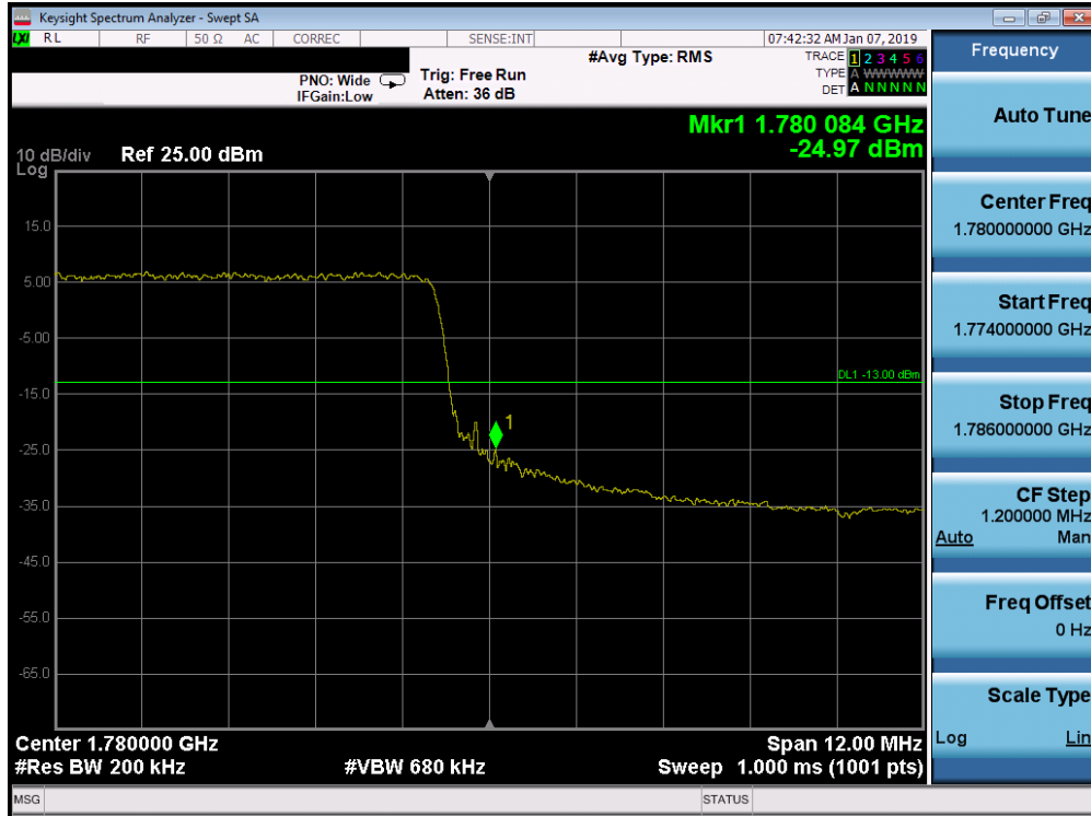
Plot 7-248. Upper Band Edge Plot (Band 66 - 15.0MHz QPSK - Full RB Configuration)
