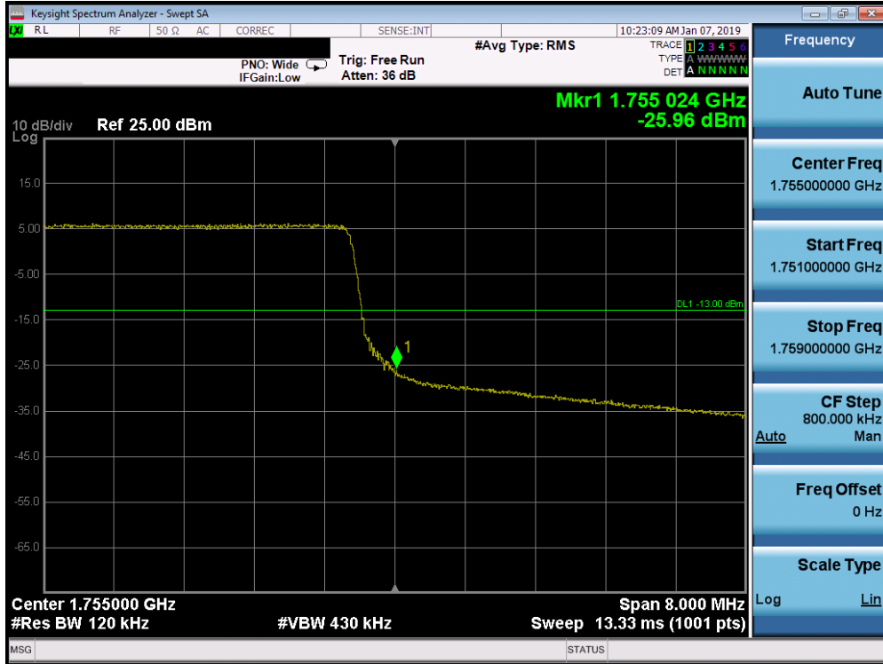
Plot 7-268. Upper Band Edge Plot (Band 4 - 10.0MHz QPSK - Full RB Configuration)
