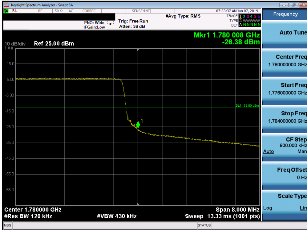
Plot 7-244. Upper Band Edge Plot (Band 66 - 10.0MHz QPSK - Full RB Configuration)
