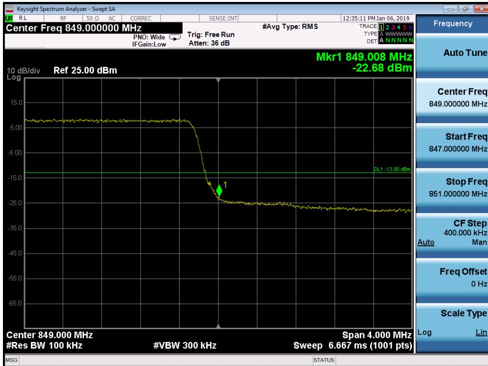
Plot 7-227. Upper Band Edge Plot (Band 5 - 5.0MHz QPSK - Full RB Configuration)
