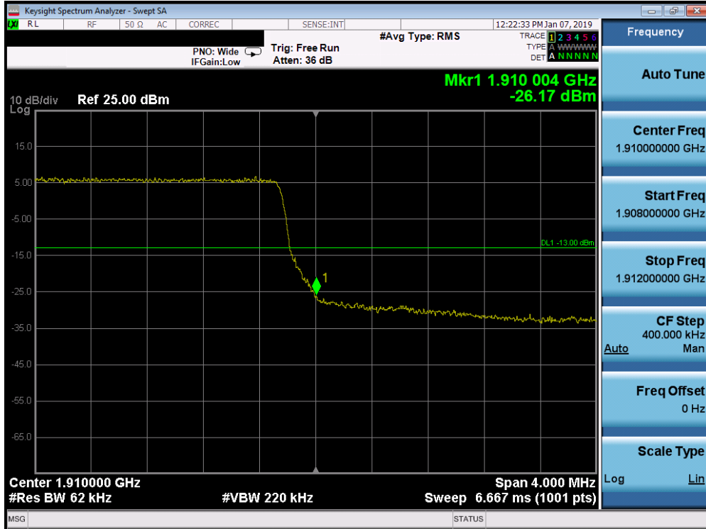
Plot 7-312. Upper Band Edge Plot (Band 2 - 5.0MHz QPSK - Full RB Configuration)
