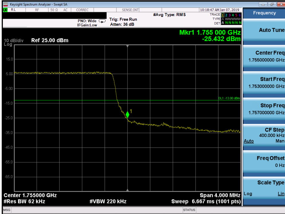
Plot 7-264. Upper Band Edge Plot (Band 4 - 5.0MHz QPSK - Full RB Configuration)
