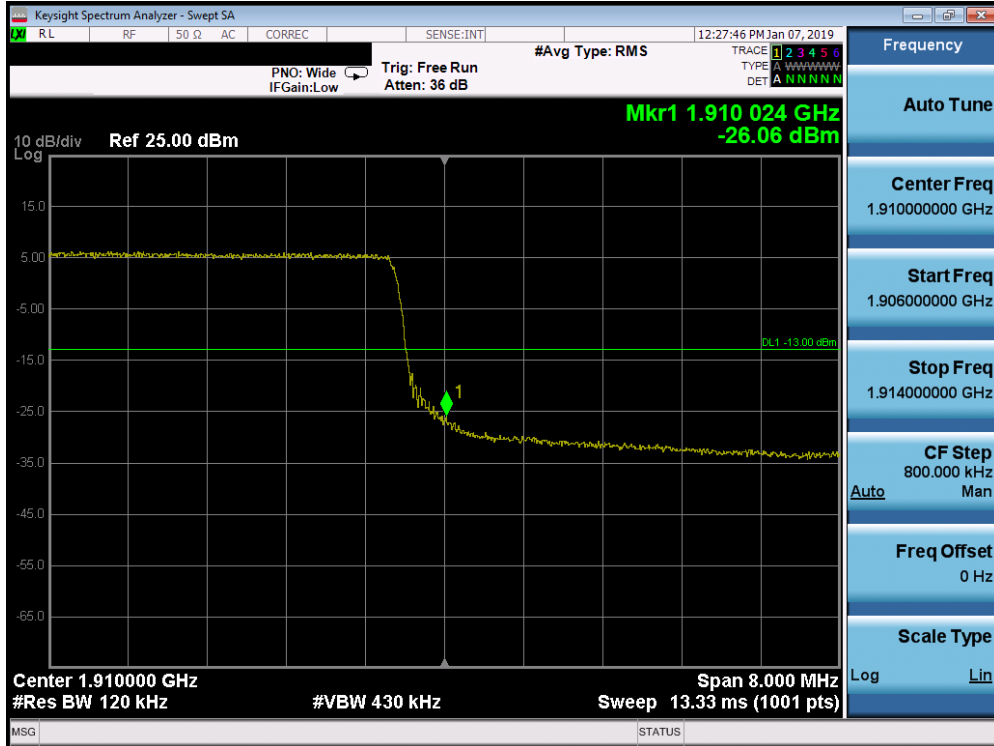
Plot 7-316. Upper Band Edge Plot (Band 2 - 10.0MHz QPSK - Full RB Configuration)
