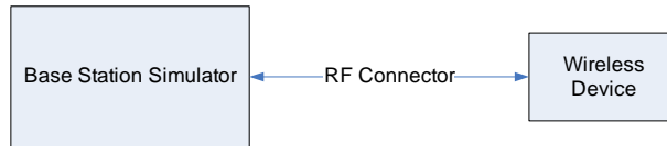
Figure 8-1 Power Measurement Setup
