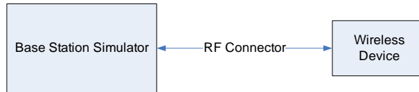
Figure 8-2 Power Measurement Setup
