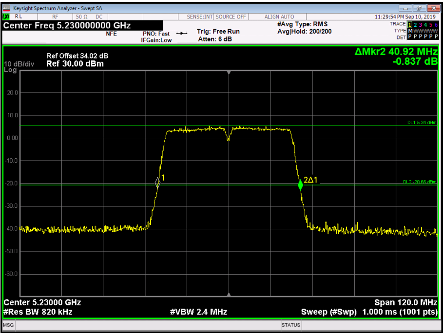
Figure 135 - 5230 MHz - 26 dB Emission Bandwidth
