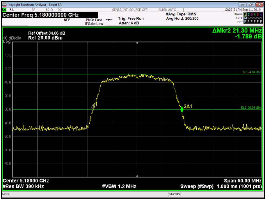
Figure 183 - 5180 MHz - 26 dB Emission Bandwidth
