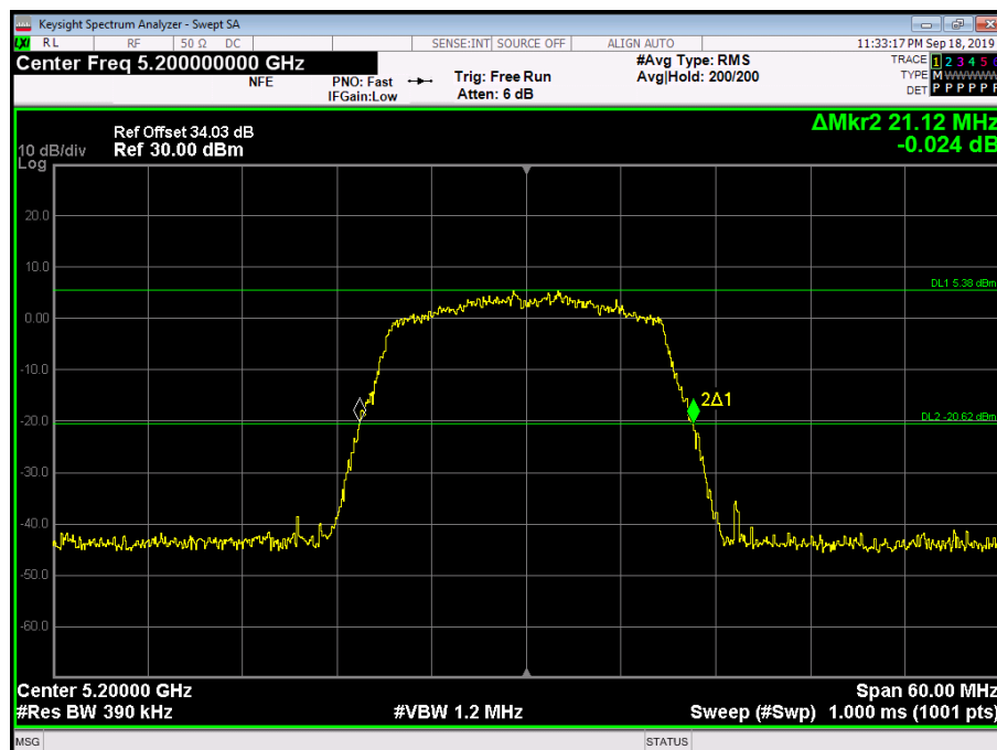
Figure 179 - 5200 MHz - 26 dB Emission Bandwidth
