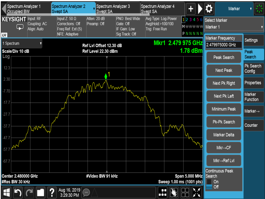
Figure 8 - 2480 MHz, Power Spectral Density
