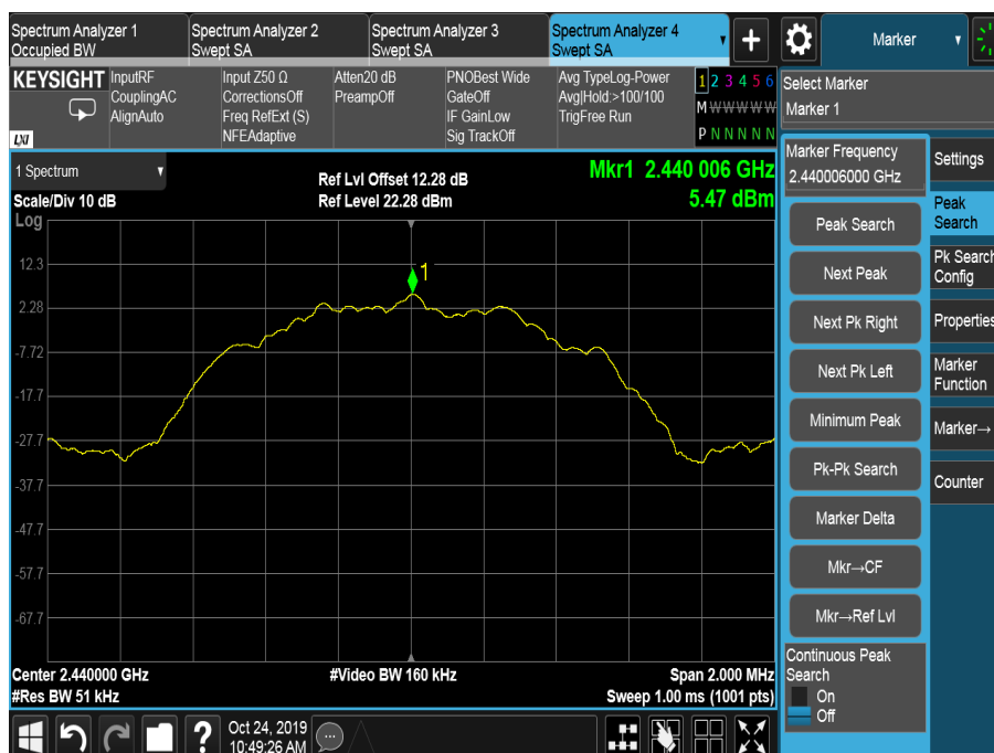
Figure 4 - 2440 MHz, Power Spectral Density
