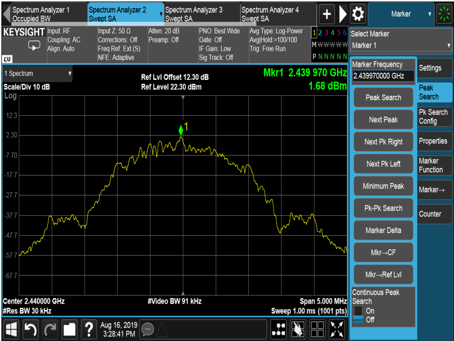
Figure 7 - 2440 MHz, Power Spectral Density
