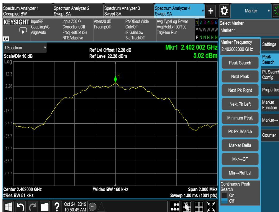
Figure 3 - 2402 MHz, Power Spectral Density
