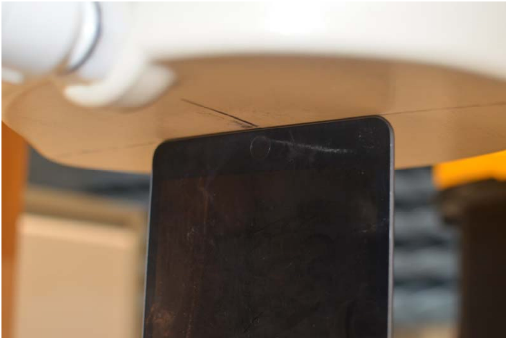
SAR Test Setup Photo 4: Bottom Edge at 0 mm
