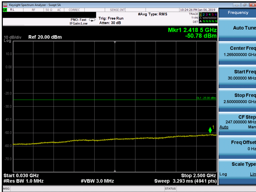
Plot 7-178. Conducted Spurious Plot (Band 7 - 20.0MHz QPSK - RB Size 1, RB Offset 0 - High Channel)
