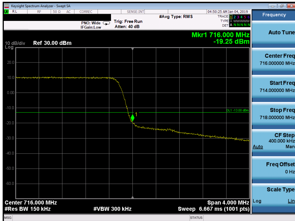
Plot 7-207. Higher Band Edge Plot (Band 17 - 5.0MHz QPSK - Full RB Configuration)
