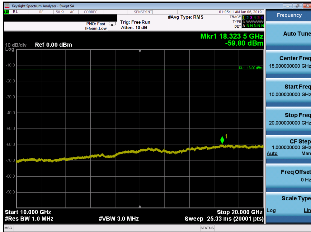
Plot 7-162. Conducted Spurious Plot (Band 25/2 - 20.0MHz QPSK - RB Size 1, RB Offset 0 - High Channel)
