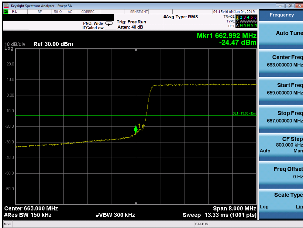
Plot 7-192. Lower Band Edge Plot (Band 71 - 10.0MHz QPSK - Full RB Configuration)
