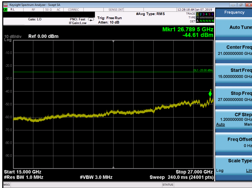
Plot 7-189. Conducted Spurious Plot (Band 41 - 20.0MHz QPSK - RB Size 1, RB Offset 0 - High Channel)
