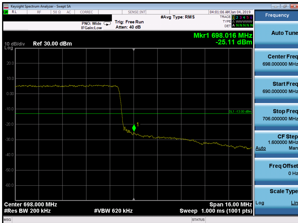
Plot 7-197. Upper Band Edge Plot (Band 71 - 20.0MHz QPSK - Full RB Configuration)
