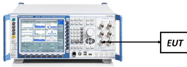
Figure 7-5. ERP Measurement Setu
