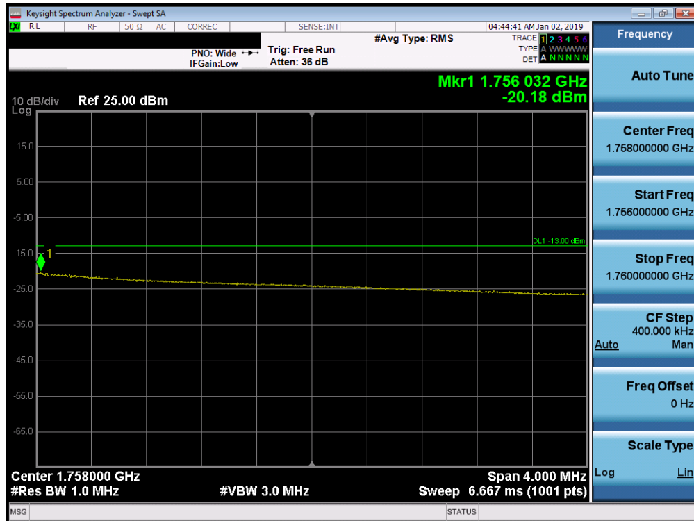
Plot 7-248. Upper Extended Band Edge Plot (Band 4 - 15.0MHz QPSK - Full RB Configuration)
