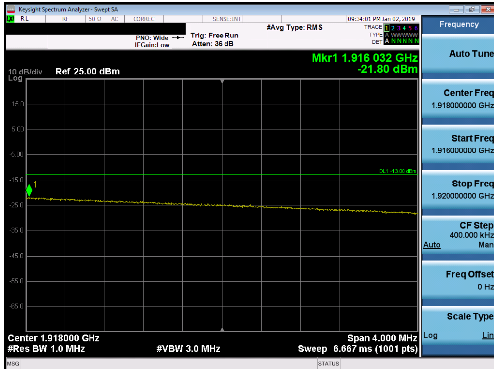
Plot 7-300. Upper Extended Band Edge Plot (Band 25 - 20.0MHz QPSK - Full RB Configuration)
