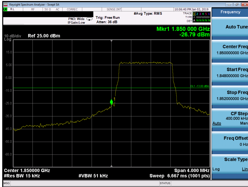
Plot 7-253. Lower Band Edge Plot (Band 2 - 1.4MHz QPSK - Full RB Configuration)
