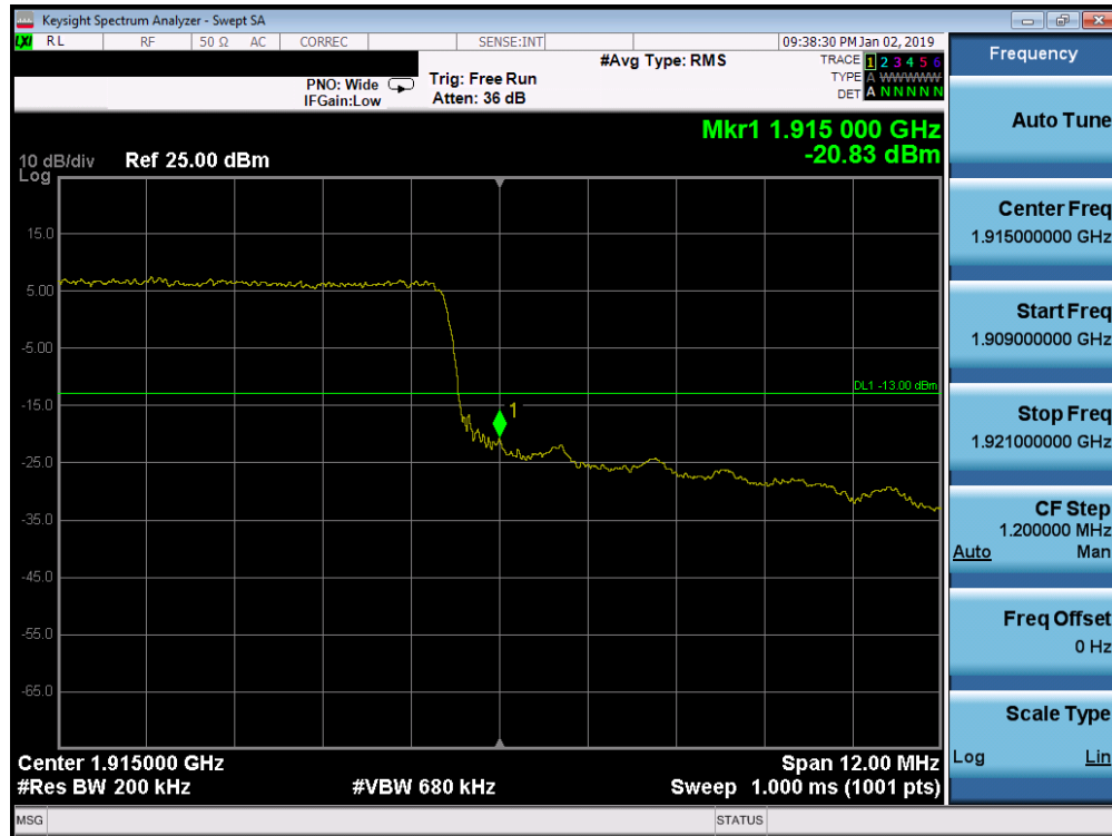
Plot 7-295. Upper Band Edge Plot (Band 25 - 15.0MHz QPSK - Full RB Configuration)
