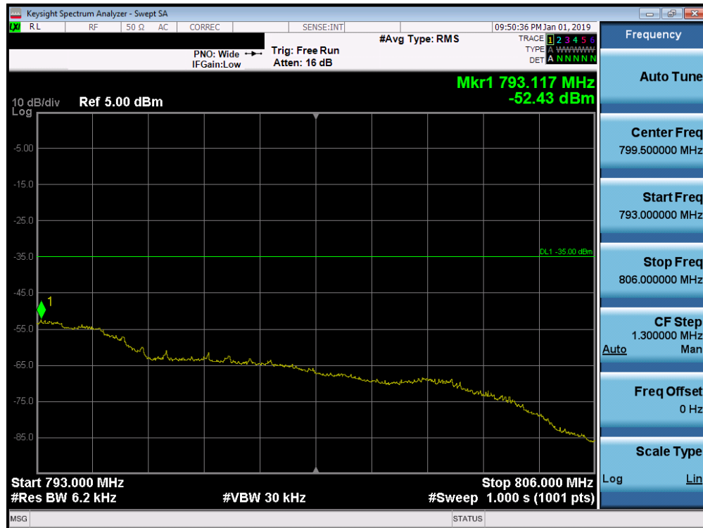
Plot 7-184. Higher Emission Mask Edge Plot (Band 13 - 5.0MHz QPSK - Full RB Configuration)
