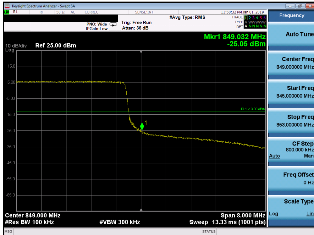
Plot 7-204. Upper Band Edge Plot (Band 26 - 10.0MHz QPSK - Full RB Configuration)
