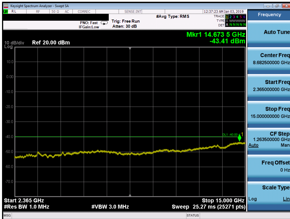
Plot 7-143. Conducted Spurious Plot (Band 30 - 5.0MHz QPSK - RB Size 1, RB Offset 0 - Low Channel)
