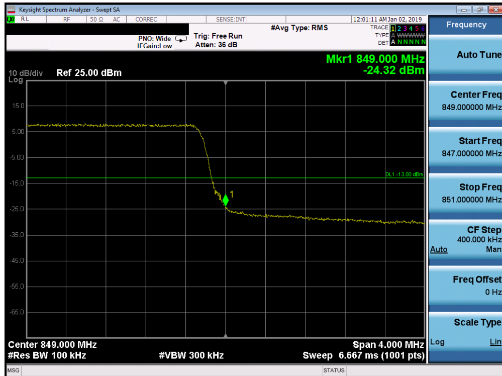
Plot 7-202. Upper Band Edge Plot (Band 26 - 5.0MHz QPSK - Full RB Configuration)
