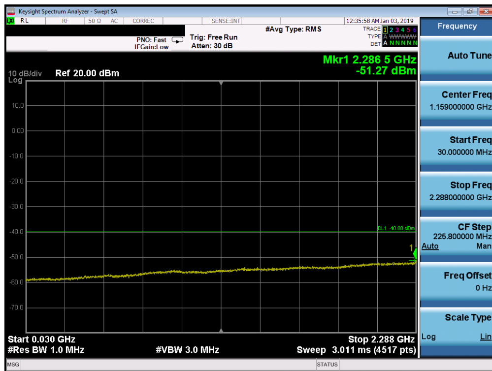
Plot 7-145. Conducted Spurious Plot (Band 30 - 5.0MHz QPSK - RB Size 1, RB Offset 0 - Mid Channel)
