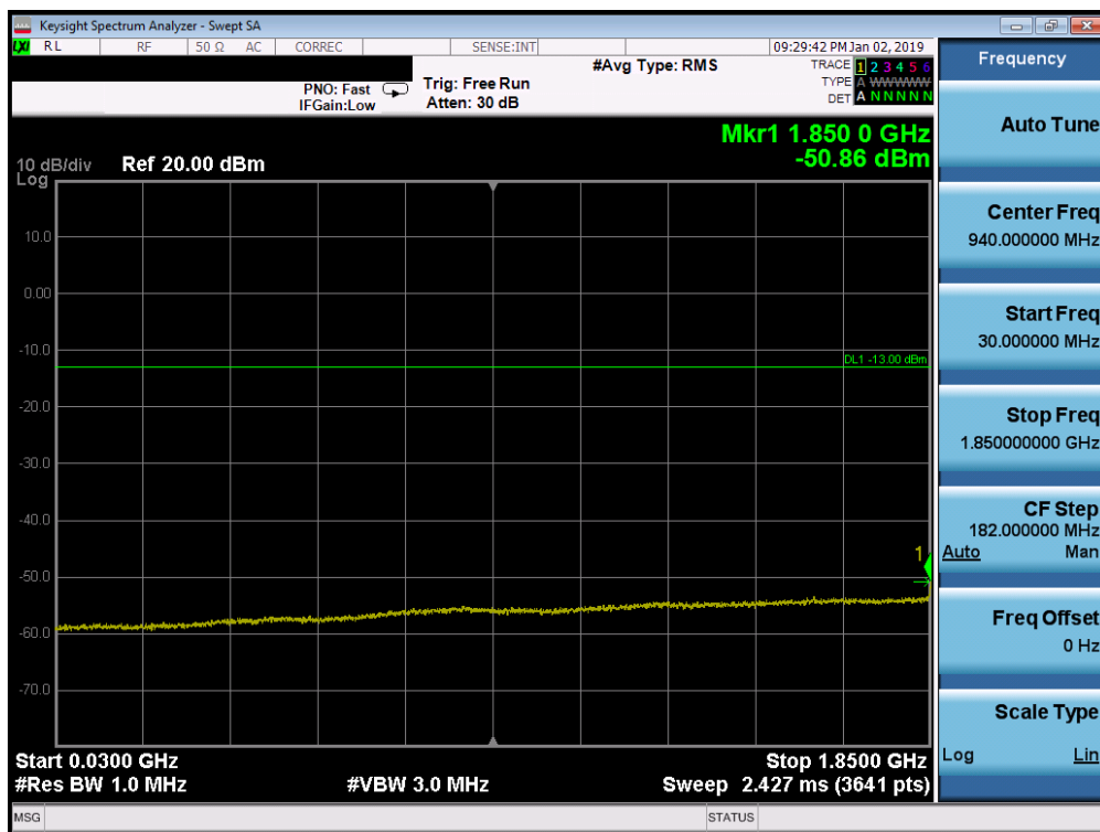
Plot 7-136. Conducted Spurious Plot (Band 25/2 - 20.0MHz QPSK - RB Size 1, RB Offset 0 - Mid Channel)
