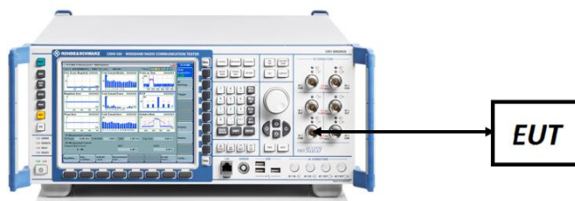
Figure 7-5. ERP/EIRP Measurement Setup
