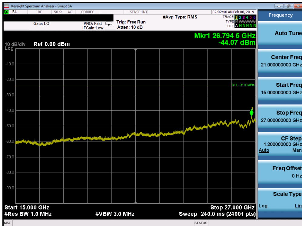
Plot 7-165. Conducted Spurious Plot (Band 41 - 20.0MHz QPSK - RB Size 1, RB Offset 0 - Mid Channel)
