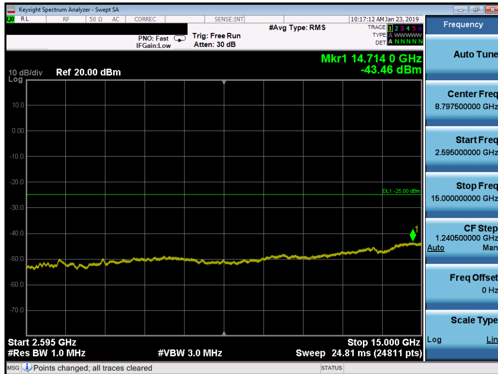
Plot 7-158. Conducted Spurious Plot (Band 7 - 20.0MHz QPSK - RB Size 1, RB Offset 0 - High Channel)
