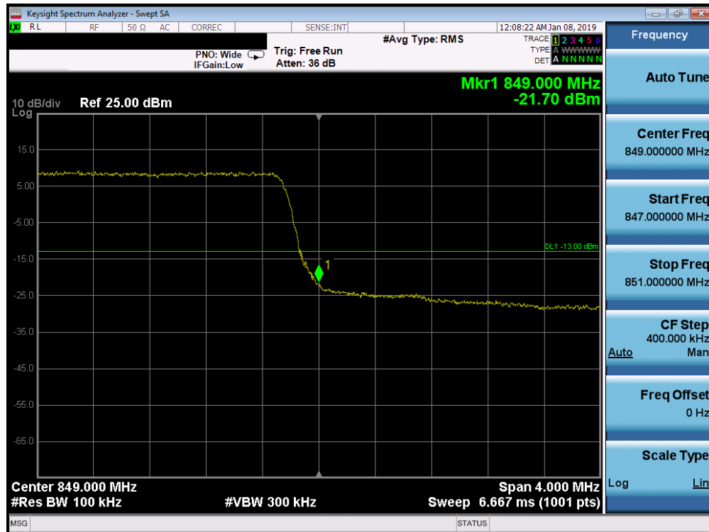
Plot 7-190. Upper Band Edge Plot (Band 26 - 5.0MHz QPSK - Full RB Configuration)
