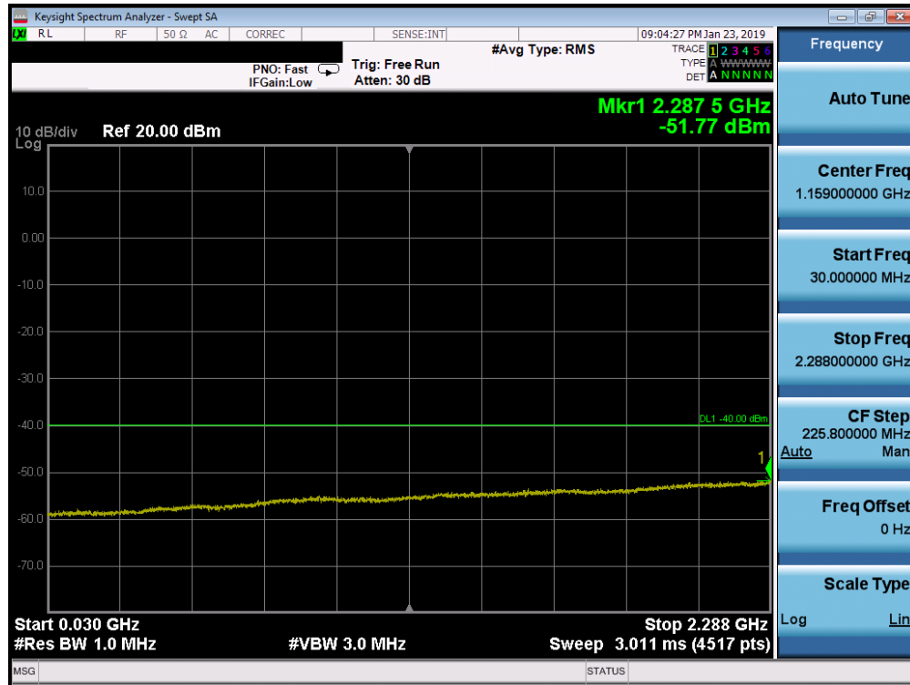
Plot 7-142. Conducted Spurious Plot (Band 30 - 10.0MHz QPSK - RB Size 1, RB Offset 0 - Low Channel)
