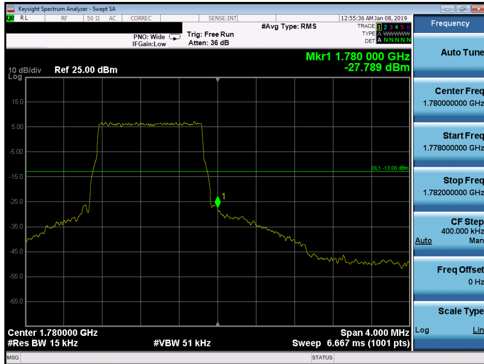
Plot 7-203. Upper Band Edge Plot (Band 66 - 1.4MHz QPSK - Full RB Configuration)
