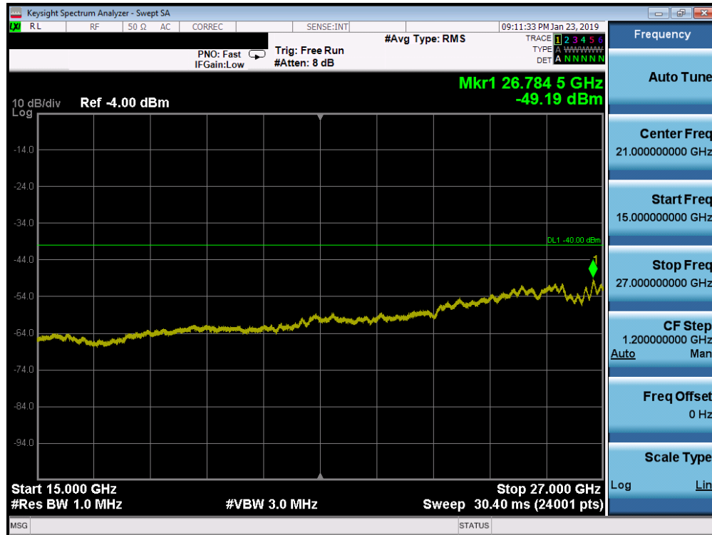
Plot 7-150. Conducted Spurious Plot (Band 30 - 10.0MHz QPSK - RB Size 1, RB Offset 0 - High Channel)
