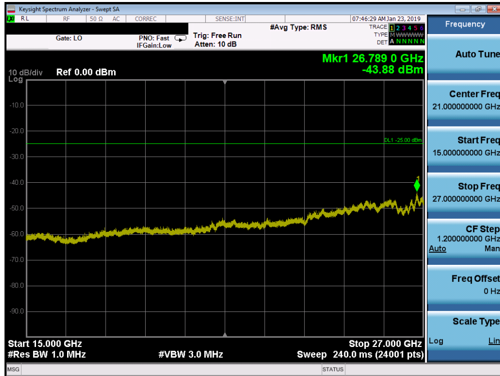
Plot 7-168. Conducted Spurious Plot (Band 41 - 20.0MHz QPSK - RB Size 1, RB Offset 0 - High Channel)
