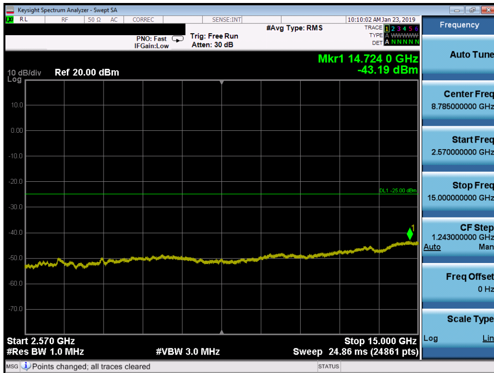
Plot 7-152. Conducted Spurious Plot (Band 7 - 20.0MHz QPSK - RB Size 1, RB Offset 0 - Low Channel)
