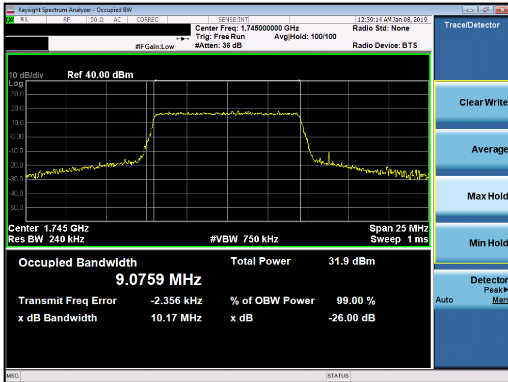
Plot 7-42. Occupied Bandwidth Plot (Band 66/4 - 10.0MHz 64-QAM - Full RB Configuration)
