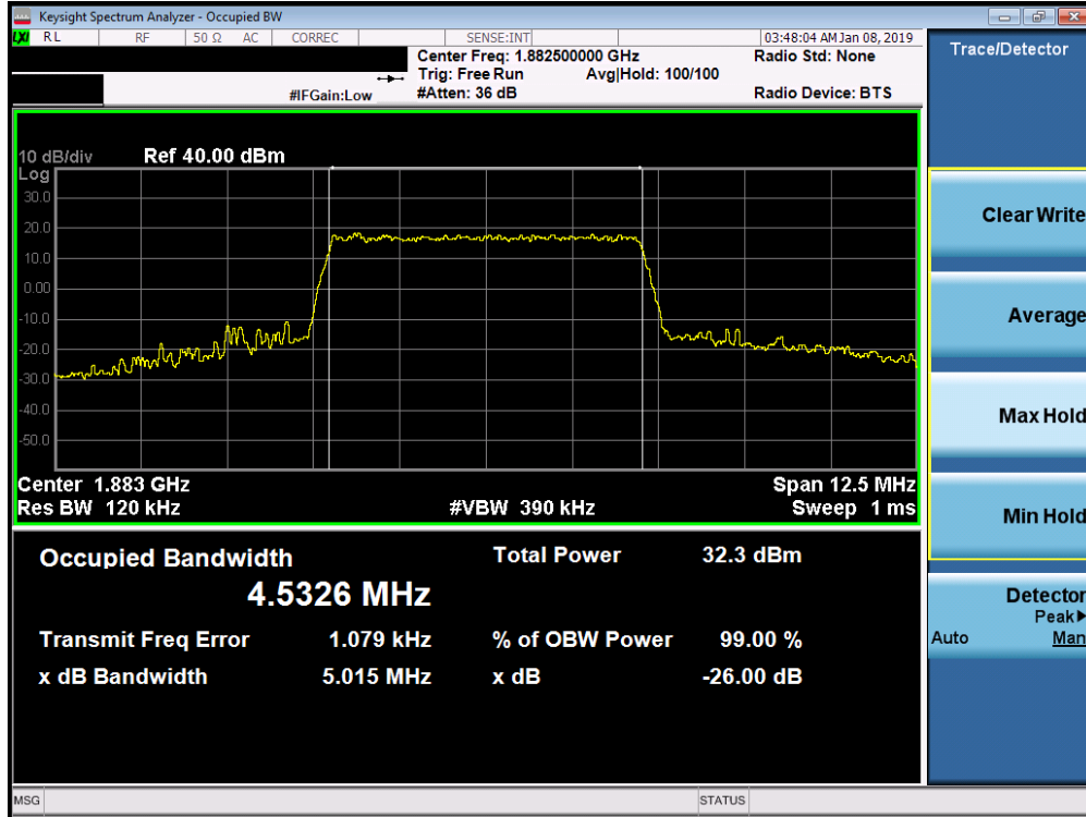
Plot 7-57. Occupied Bandwidth Plot (Band 25/2 - 5.0MHz 64-QAM - Full RB Configuration)
