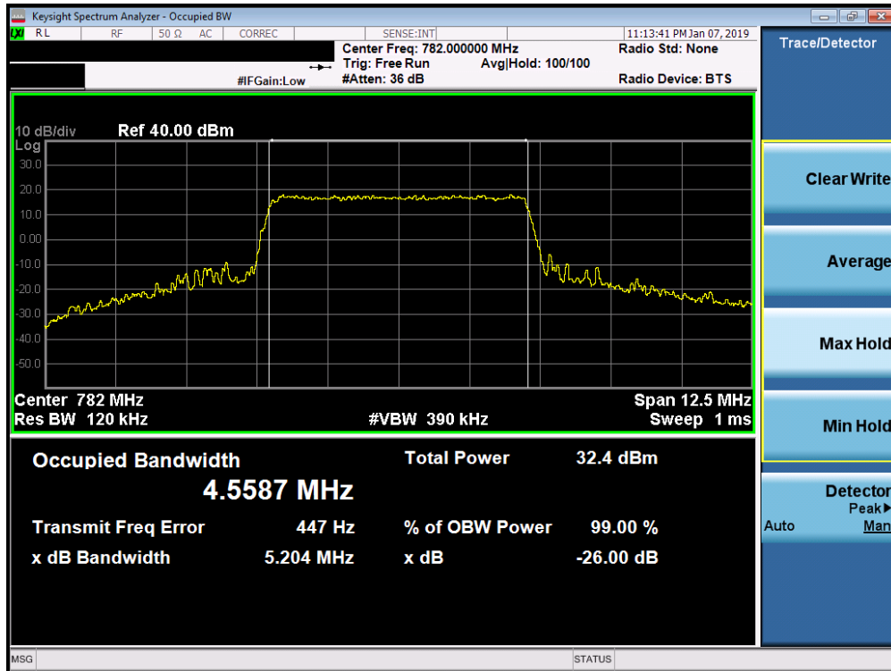
Plot 7-15. Occupied Bandwidth Plot (Band 13 - 5.0MHz 64-QAM - Full RB Configuration)
